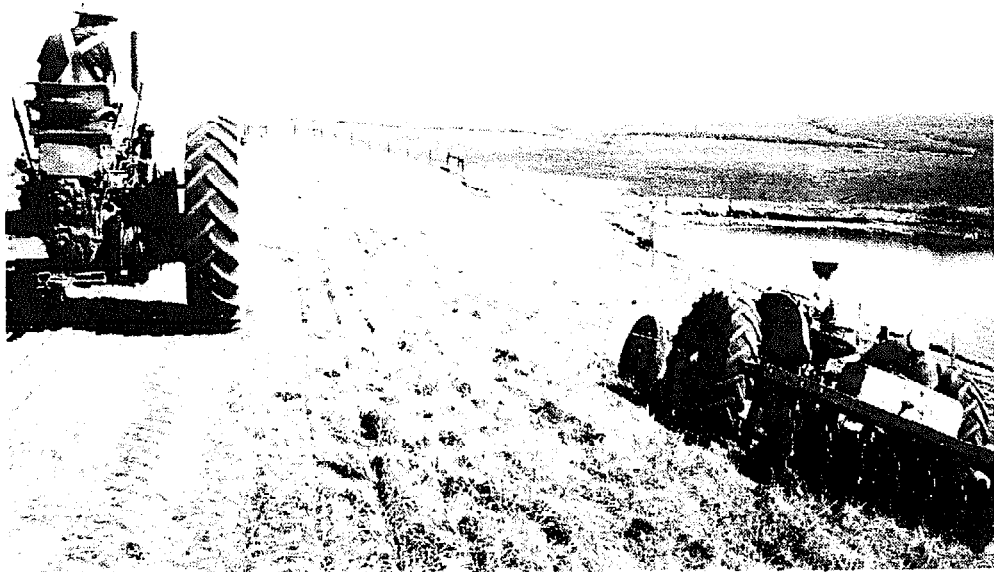
Fig. 13-13. Notched disk cutting notches into which mulch is anchored.
