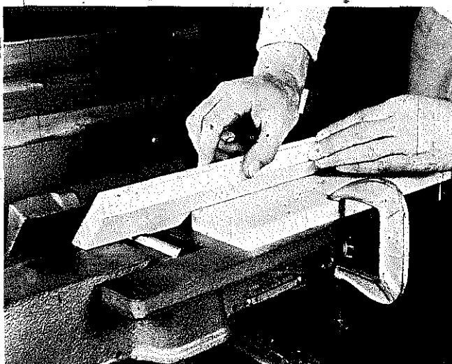
Bevels or chamfers are accomplished by tilting the fence to the angle desired. A closed angle is best since it creates a nook for the work. Even so, a clamped guide block keeps the work in just-so position.
