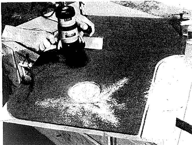
The router, equipped with a template guide and used with a pattern, is excellent for outlining duplicate pieces.
