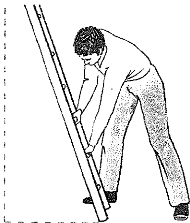
The foot should be extended one quarter of the ladder's length.
