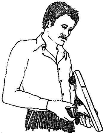
Use a long plane for accurate results on a long edge.
