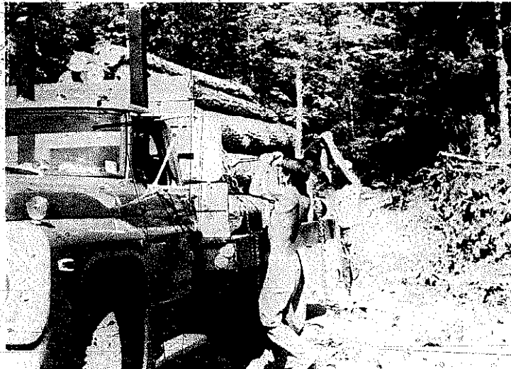
PLATE 270 When the truck is loaded, the logs are chained down with chains tightened by log binders for the trip to the mill. Before leaving, the men put Charley in the shed they have built for him on the site and feed him. Charley spends each night there waiting for them to return early the next morning with an empty truck.
