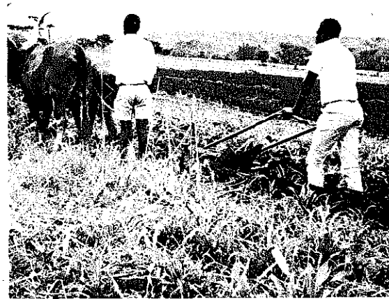
Photo 1.5. An animal-drawn, two-bottom moldboard plow (Kenya).
