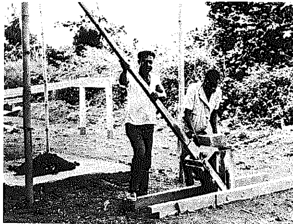
Photo 8.12. Cinva Ram block-making machine.
