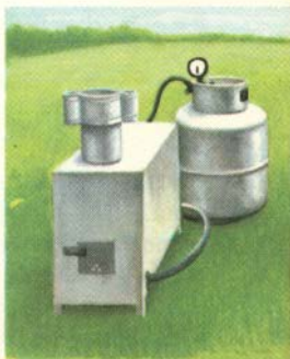
Silver iodide generator.
