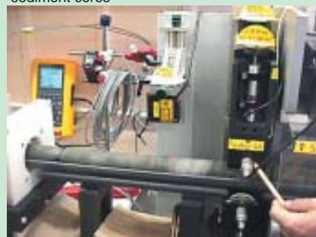
Core scanning equipment measures the physical properties of the drill core
