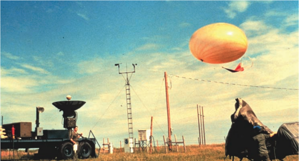
Scientists release a rawinsonde balloon, while weather instruments and a mobile radar unit (background) also monitor humidity, air pressure, precipitation, and temperature. (NOAA Photo Library, NOAA Central Library; OAR/ERL/National Severe Storms Laboratory)
