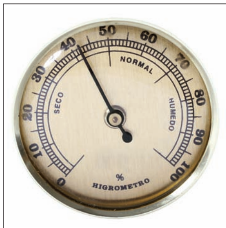
Hygrometers like this one have been used for hundreds of years to measure humidity.
