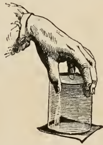
Fig. 12.—Atmospheric pressure under an inverted glass.
