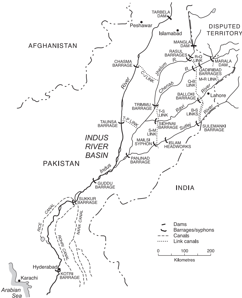
FIGURE 4.10. Map of the Indus River basin, showing the principal tributaries and the principal elements of the Indus water control projects.
