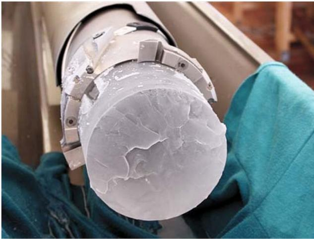
Figure 13 Ice core protruding from the drill head from EPICA Dome C, Antarctica (photo courtesy of Eric Lefèvre, LGGE, Grenoble).
