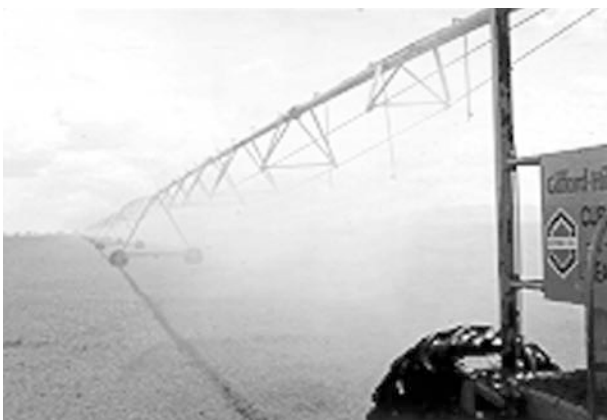
Fig. 12 Linear move irrigation systems have equipment similar to center pivots but move from one end of the field to the other as side roll systems operate. (Courtesy of Natural Resource Conservation Service, USDA; www.nrcs.usda.gov .)
