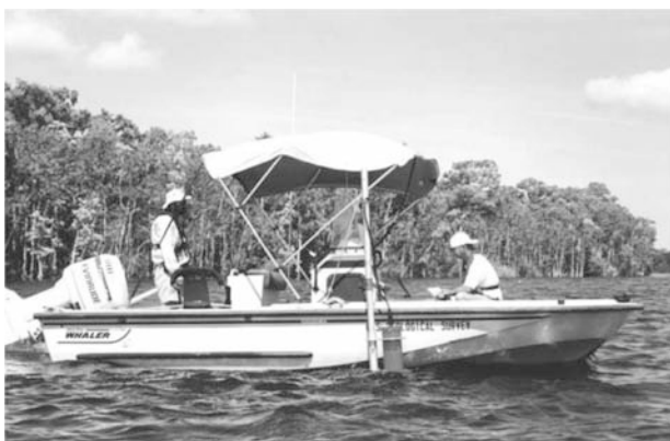
Fig. 2 Hydrologist measuring streamflow using an acoustic doppler current profiler.
