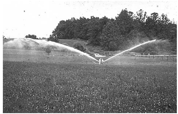
Fig. 13 Traveling sprinkle systems commonly use large guns and pull themselves across the field using a cable and winch. (Courtesy of Dr. Harold Duke, ARS, USDA retired.)
