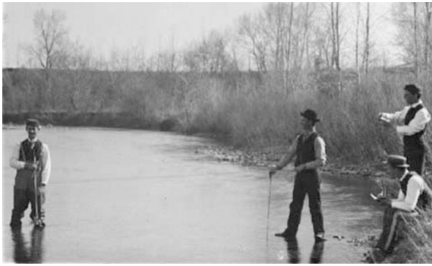
Fig. 3 Rating party stream-gaging on the Cache la Poudre River near Fort Collins, Colorado, 1902.
