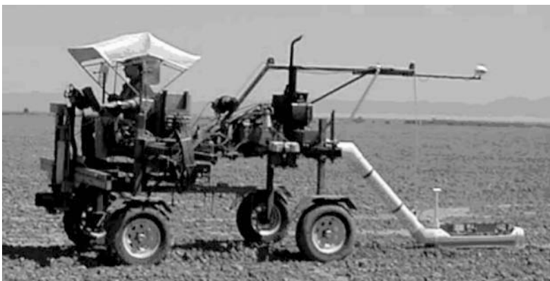
Fig. 3 Mobile dual-dipole EM-38 equipment for the continuous measurement of EC_a . Dual-dipole EM meter rests in the tail section or sled at the rear of the vehicle with a GPS antenna overhead at the midpoint of the meter.
