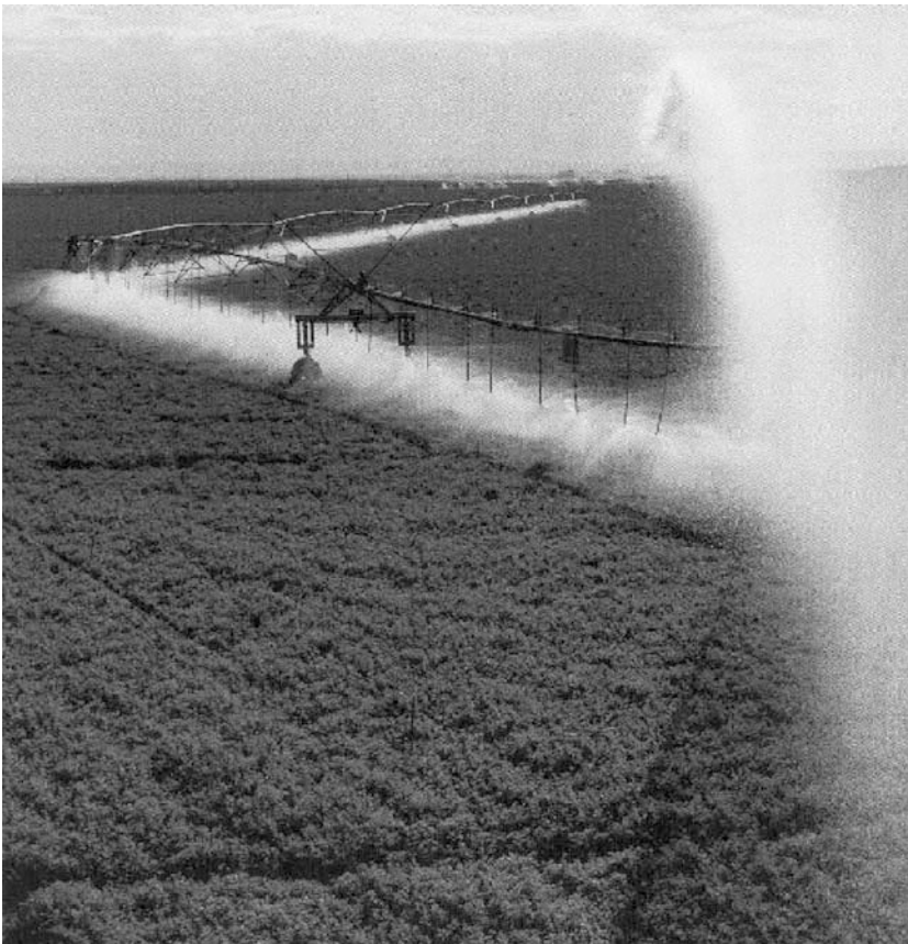
Fig. 2 Center-pivot lateral with swingspan corner system partly extended. Sprinklers are mounted on drop tubes below the lateral.
