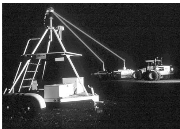
Fig. 7 Laser controlled leveling, for level basins in United States up to 8 ha in size, is now used to accomplish precision land leveling in surface irrigation around-the-world. (Courtesy of Natural Resource Conservation Service, USDA; www.nrcs.usda.gov .)
