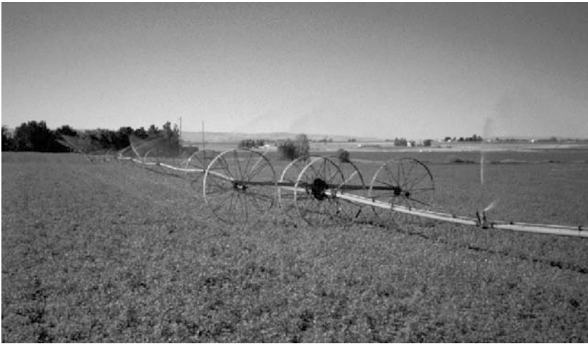
Fig. 1 Sideroll lateral with mover unit in foreground. Note the small driveshaft parallel to the lateral pipe on the right, which transfers power to the mover mechanism.
