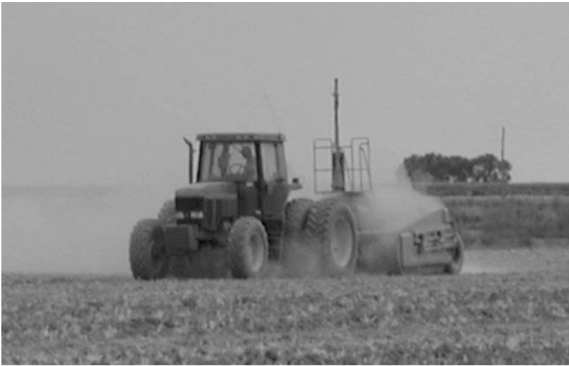
Fig. 7 Laser guided land leveling equipment. (Utah State University Irrigation Photo Archives.)
