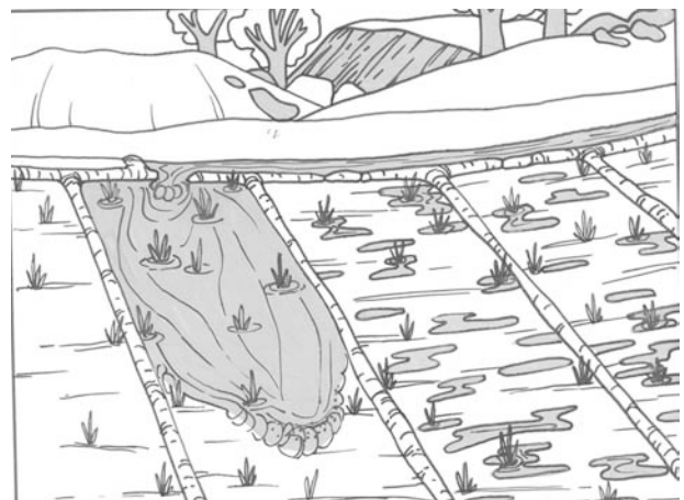
Fig. 4 Graded border irrigation systems with bunds to guide the water down the slope and cross slopes eliminated. (Water Management Synthesis II Project, Colorado State Univ., Fort Collins, CO.)
