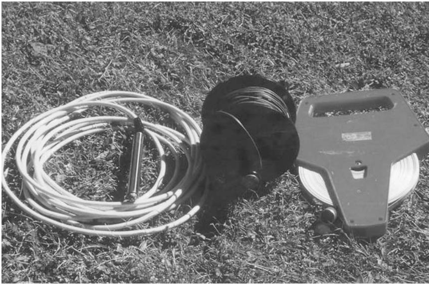
Fig. 1 Pressure transducer (left), electrical sensor (middle), and vinyl tape and popper (right).
