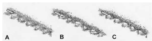
Fig. 6 Flow conditions on a stepped channel: (A) skimming flow; (B) transition flow; (C) nappe flow.
