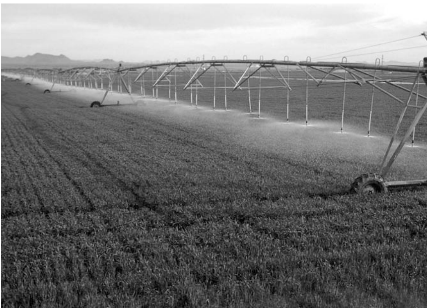
Fig. 10 Center pivot irrigation system for irrigation of a field. (Courtesy of Natural Resource Conservation Service, USDA; www.nrcs.usda.gov .)
