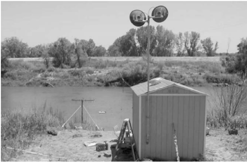
Fig. 3 Pulsed Doppler radar on top of equipment shelter, and UHF radar antenna to left of shelter on bank of San Joaquin River, CA, are used for surface-velocity measurements. Cable across channel is used to suspend Ground Penetrating Radar (GPR) system over the water to measure channel cross section. Non-contact methods of streamgaging show substantial promise, but much remains to be learned.
