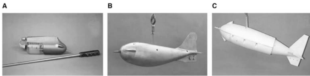
Fig. 3 (A) The U.S. DH-48 suspended-sediment sampler, glass sample bottle shown. (B) The U.S. D-74 suspended-sediment sampler, glass sample bottle in sampler body. (C) The U.S. D-96 suspended-sediment sampler, flexible sample bag in sampler body. Source: From Refs. [3,4,6,7] .
