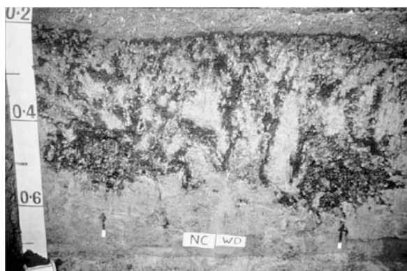
Fig. 2 Illustration of macropore flow. This strongly structured, cultivated soil was flood irrigated with dye solution, causing preferential flow through macropores. This type of flow in “dual-porosity” soils, subsoils, or underlying rock (e.g., limestone with fissures or conduits) can fast-track contaminants and pathogens to groundwater. (Photo courtesy of K.C. Cameron, Lincoln University, Canterbury, New Zealand.)
