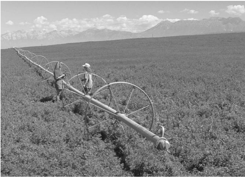
Fig. 9 Side roll sprinkler systems for irrigation of a field. (Courtesy of Natural Resource Conservation Service, USDA; www.nrcs.usda.gov .)
