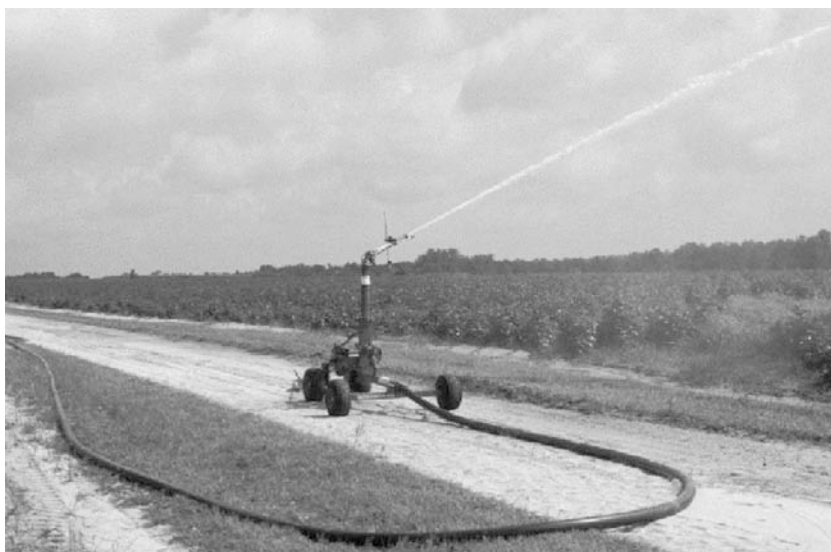
Fig. 5 Soft-hose traveler beginning a pass. The sprinkler cart is towed by a cable (not visible).
