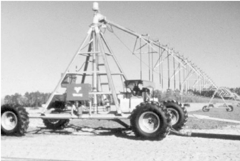
Fig. 3 Linear-traveling lateral, hose-drag type, with on-board engine. This lateral can also pivot about the inlet structure. Sprinklers are mounted on drop tubes.
