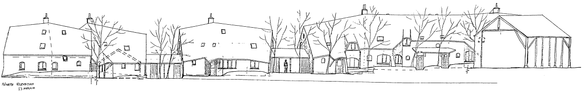
Low, wind-shedding, north-facing front, higher south-facing, rear. Welcoming scale and minimum shade on communal green side, maximum solar gain to south.
