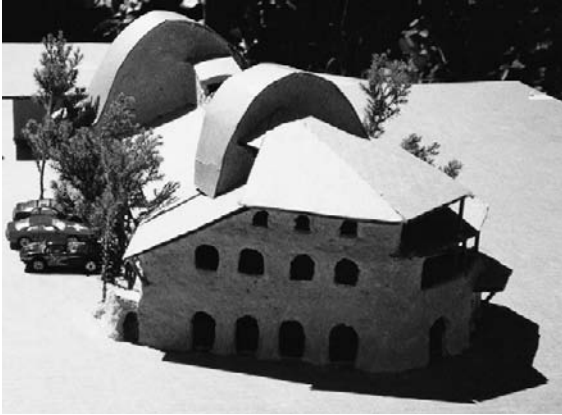
Models – design tools to work out space and construction – are also useful to test sun and shade at different times of day. (Shops, offices and apartments, California)
