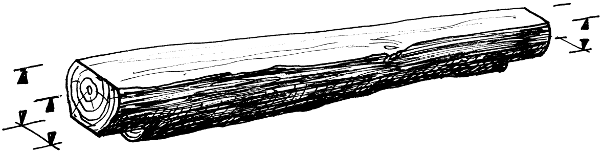
Small-section roundwood, minimally sawn for true faces only where needed, utilizes timber and fibre strength wasted by conventional sawing.
