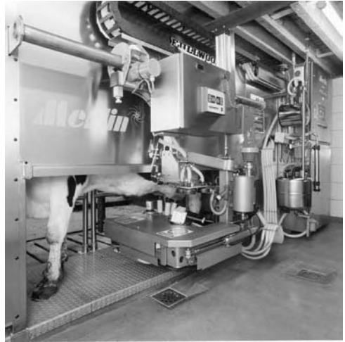
Fig. 25.3. Over 3000 robotic milking installations are now operating. Cows can now be farmed with only occasional contact with humans. This places great emphasis on designing the environment with which they interact to optimize production and welfare. Photo: Fullwood Ltd.
