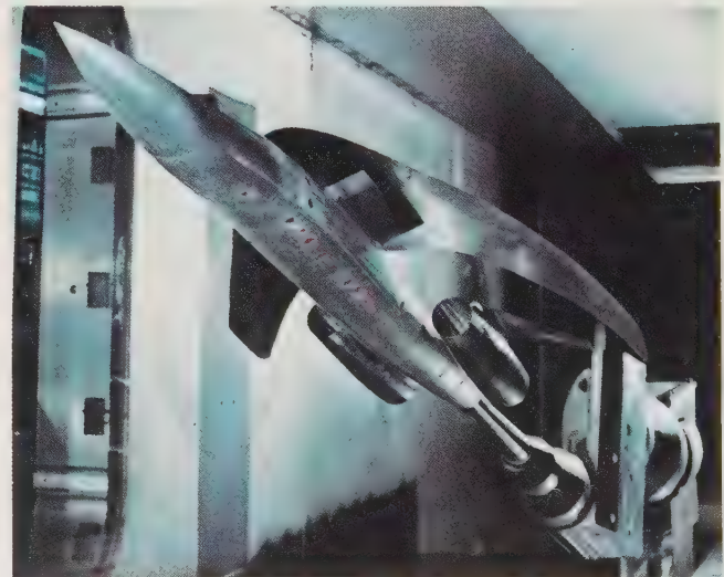
A model of a Mach 4.5 interceptor with scimitar wings undergoing tests in a wind tunnel at Arnold Engineering Development Center. (Photo, AEDC)
