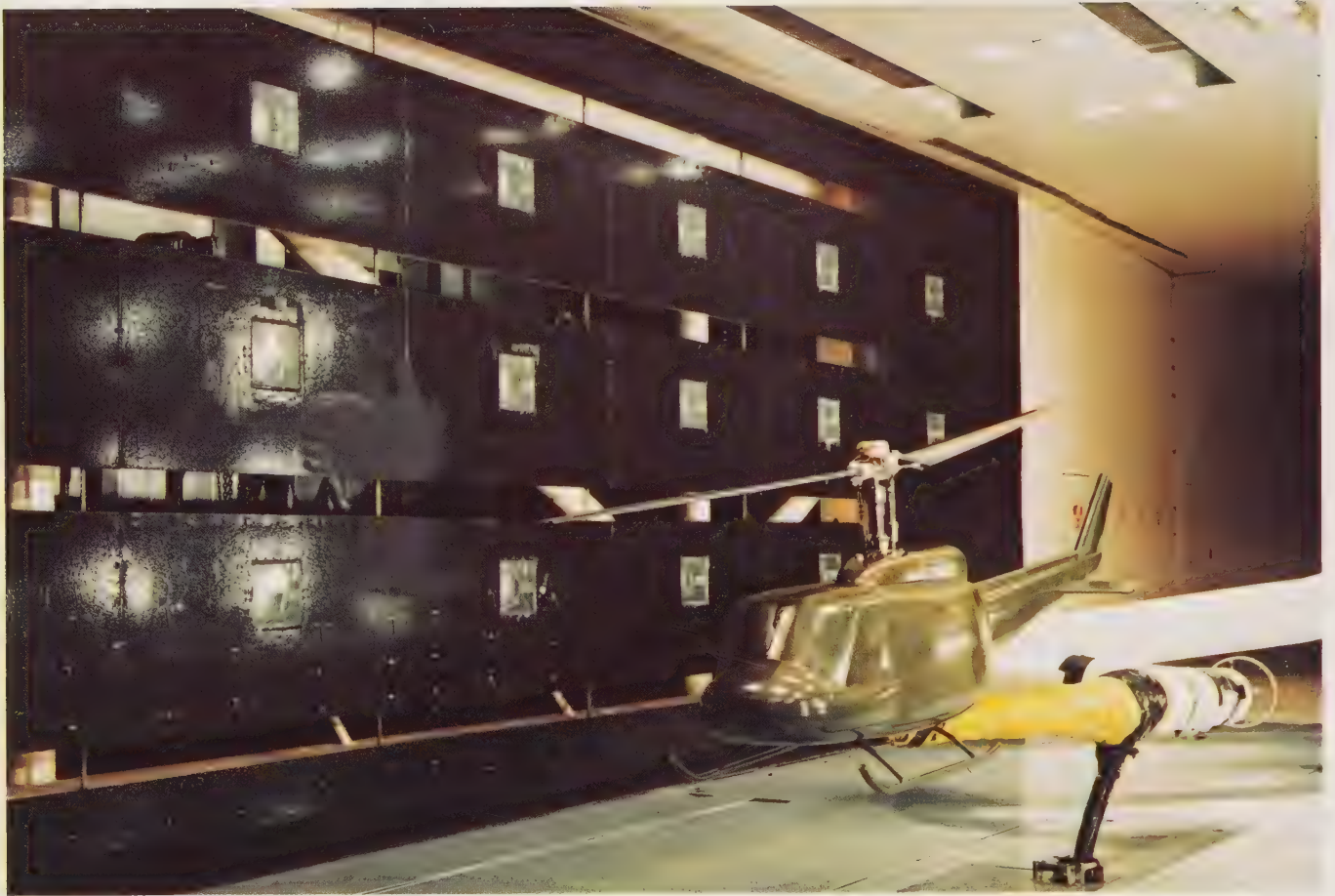
The slotted wall, one of the Tinkertoy interchangeable wall sections that helped reduce wall interference in the V/STOL wind tunnel.
