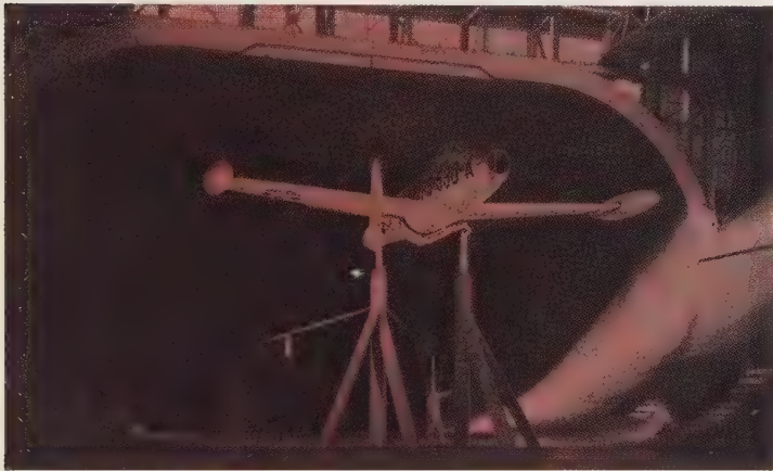
An F-84 Thunderjet has room to spare in the test section of the Ames 40 x 80-foot tunnel.
