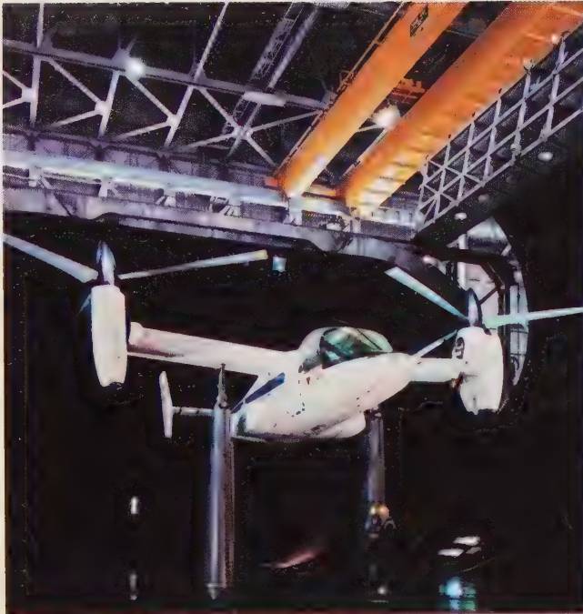
The XV-15 tilt-rotor research aircraft undergoing tests in the Ames 40 × 80-foot tunnel. The critical transition occurs when the rotors tilt forward for horizontal flight.
