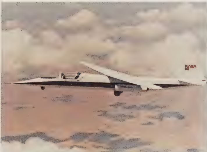
A flight model of the experimental NASA pivot-wing AD-1. The wing is shown canted in the high-speed position. At low speeds it is perpendicular to the fuselage axis.
