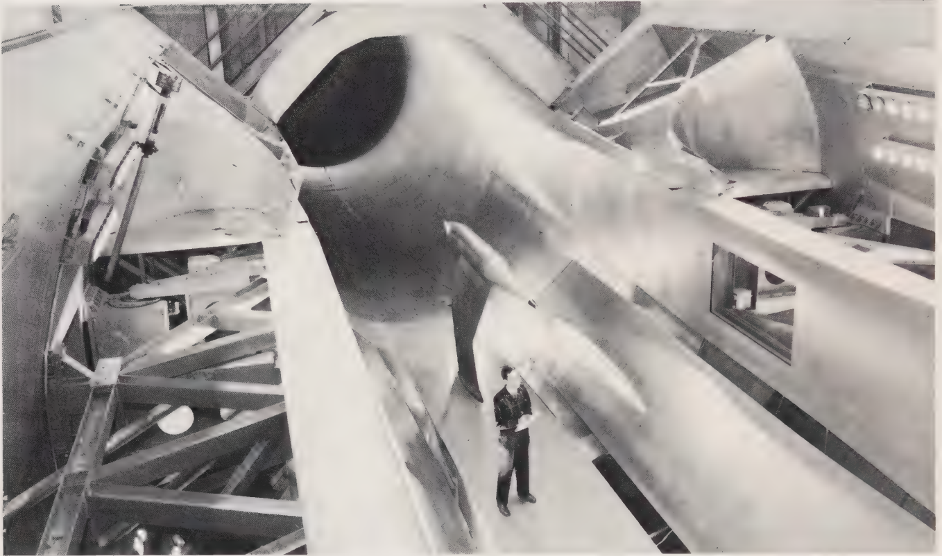
The Langley 16-foot high-speed tunnel with the slotted wall installed to convert it to transonic operation. (The top half of the test section is shown open.)
