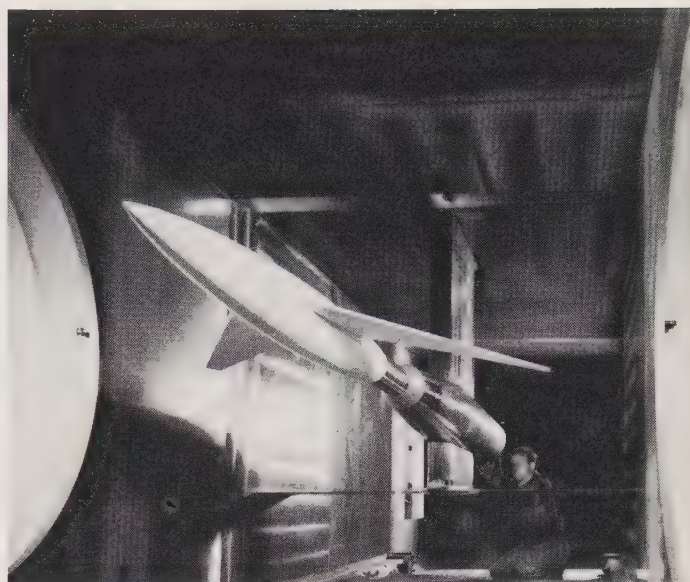
An aircraft model mounted inside the test section of the Ames 6 × 6-foot supersonic tunnel. The 50-inch-diameter circular glass windows are precisely ground and almost free of imperfections so that schlieren photos can be taken.
