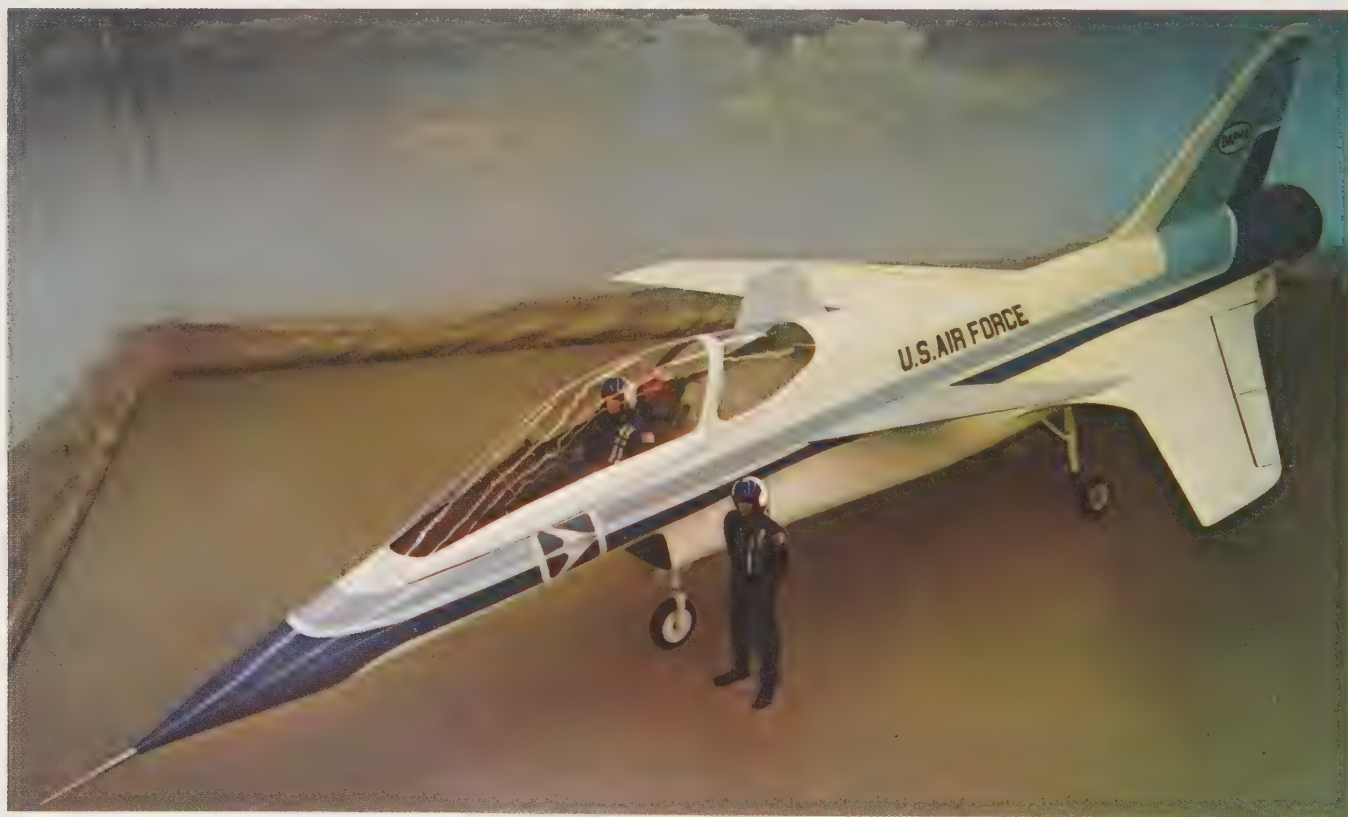
Full-scale mockup of a fighter with swept-forward wings. (Photo, Rockwell International)
