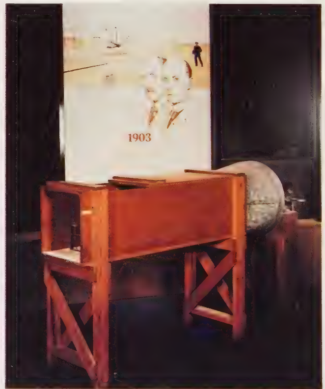
Working replica of the 1901 Wright brothers wind tunnel in the National Air and Space Museum. (Photo, National Air and Space Museum)
