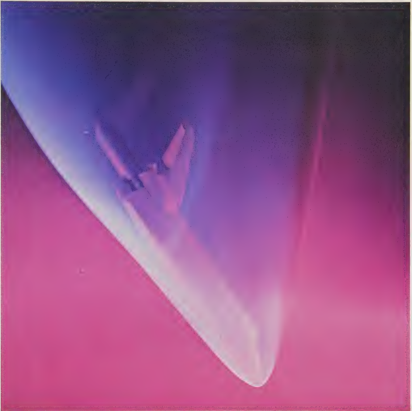
A model of the Space Shuttle in the Langley 22-inch helium tunnel at Mach 20. The flow is made visible by bombardment of an electron beam.
