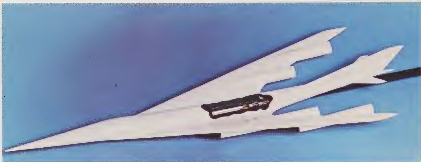
Supersonic transport model with its aerodynamically clean sting support. The cutaway of the model reveals the components of an internal balance.
