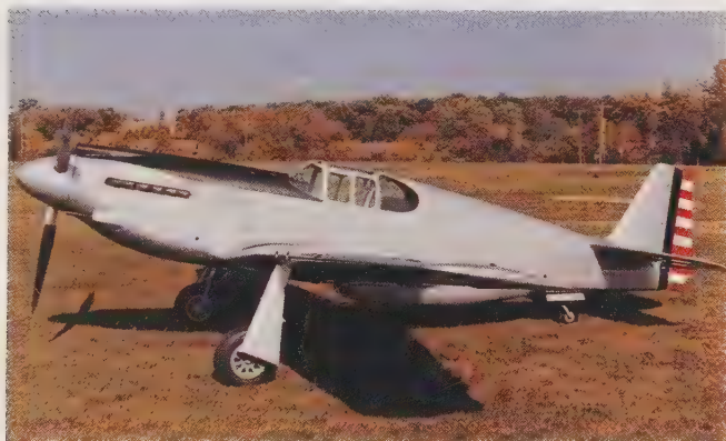
A P-51 at Langley in December 1951. The great range of this fighter was credited to the new NACA 6-series, low-drag wing, developed in NACA's low-turbulence tunnel. With less fuel needed to fight drag, the P-51 could escort bombers all the way to Berlin, drastically cutting bomber losses. (Photo courtesy EAA Air Museum Foundation)
