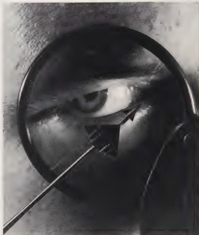
Tiny SST models used in sonic boom research in wind tunnels.
