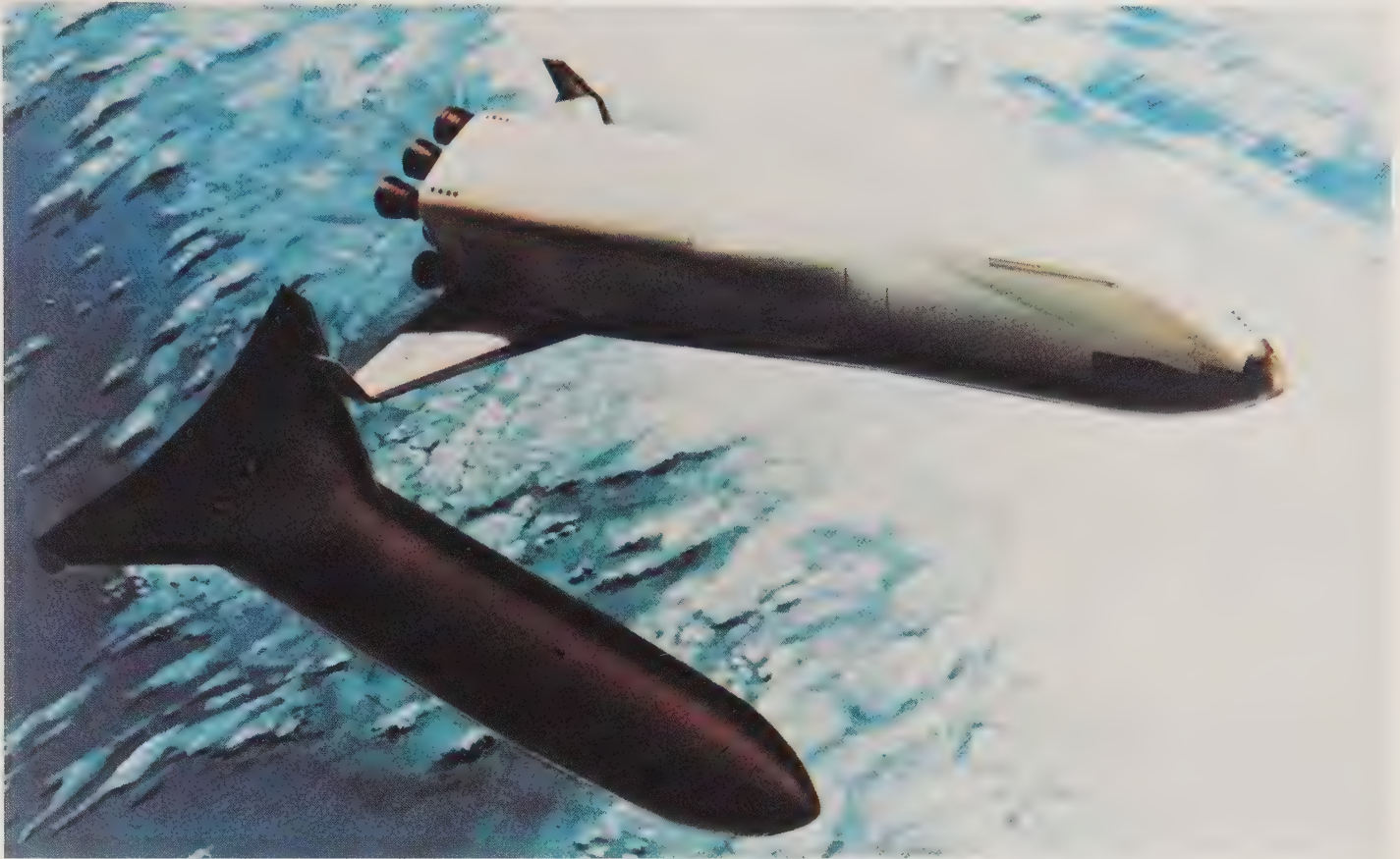
A possible configuration of a heavy-lift launch vehicle. Taking off vertically, like the Space Shuttle, this launcher could place up to 500 tons into low Earth orbit. Both stages are recoverable. (Photo, The Boeing Company)
