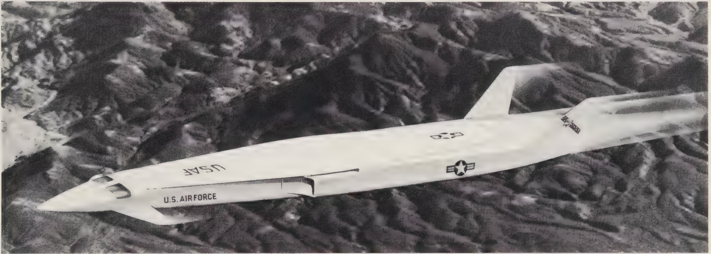
A bomber with pivoting wings rotated back almost flush with the fuselage for high-speed flight. Body lift is sufficient for high-speed flight at low altitudes. (Courtesy Rockwell International)
