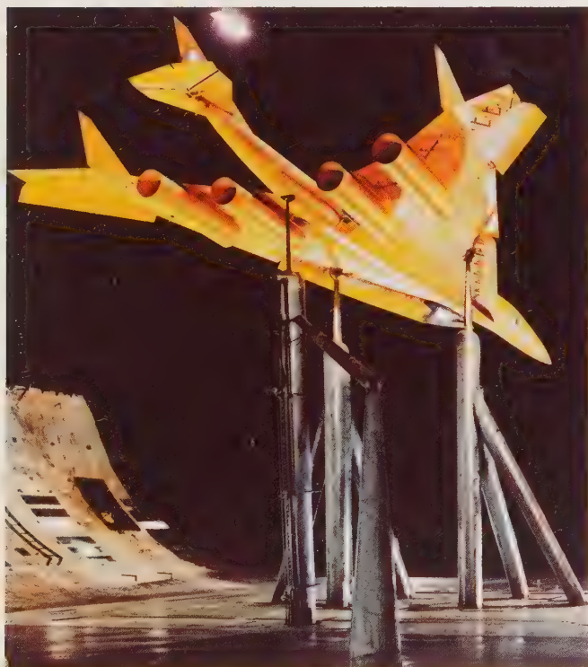
An SST model in the cavernous test section of the Ames 40 × 80-foot tunnel.
