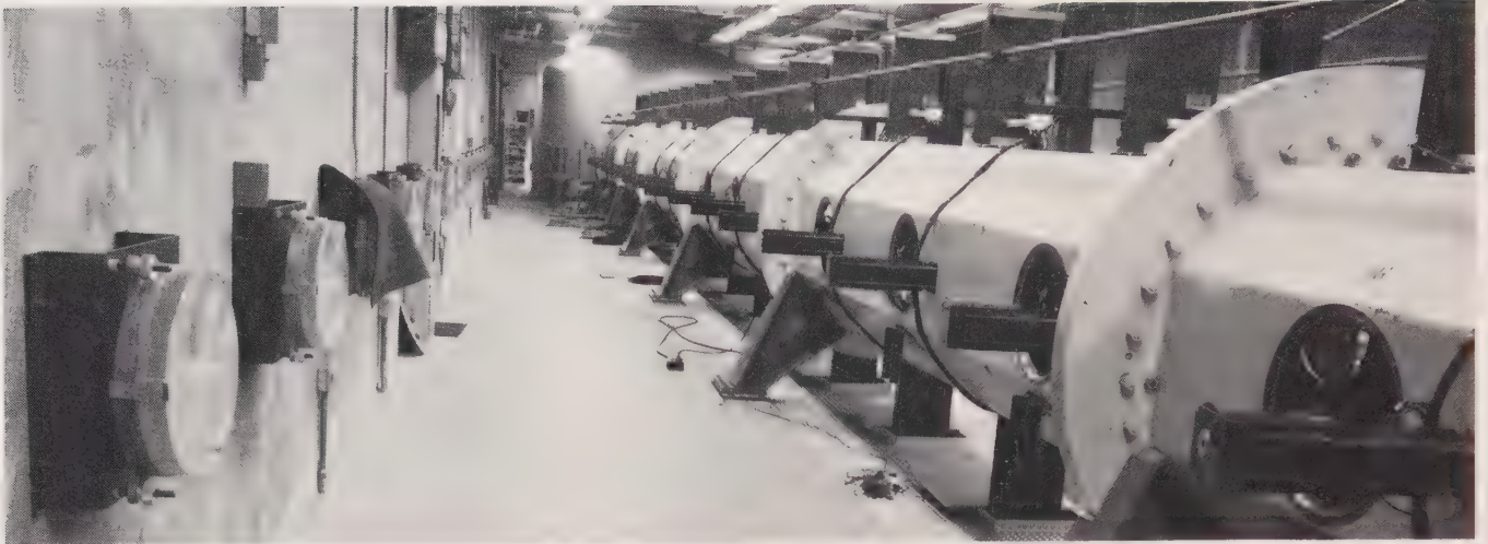
Two guns firing at each other at the Ames Hypersonic Free-Flight Aerodynamic Facility. The shock tube (left) fires a gaseous bullet at the light-gas gun (right), which shoots a small model into the onrushing gas.
