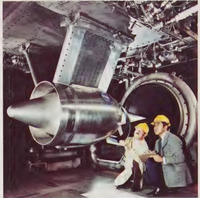
Full-scale "boilerplate" version of a hypersonic ramjet mounted in the Lewis hypersonic tunnel.
