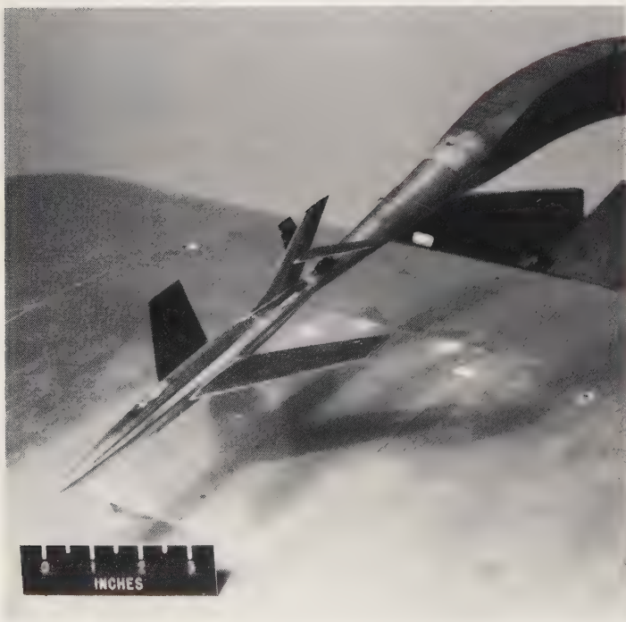
An early version of the X-2 research aircraft undergoes tests on the transonic "bump" of the Langley high-speed 7 × 10-foot wind tunnel. Local airflow over the bump reaches the speed of sound.
