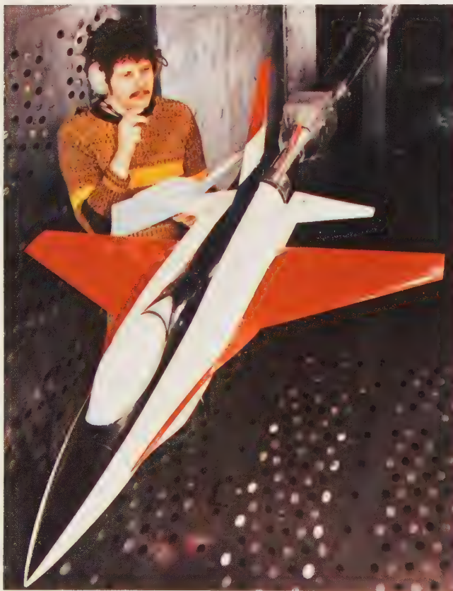
Nozzle drag tests on the General Dynamics F-16 inside the supersonic test section of the Lewis 8 × 6-foot tunnel.
