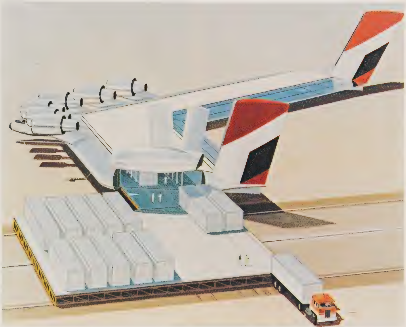
A swept-wing span-loader concept. The cargo space is inside the thick wings. (Courtesy The Boeing Company)
