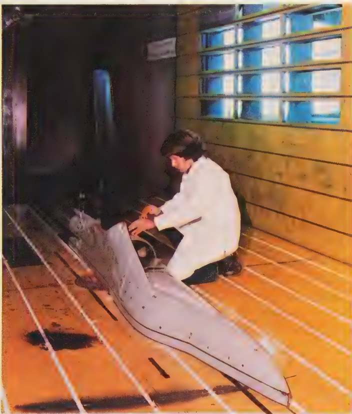
A 1/6-scale model in the Ames 11-foot Unitary Plan transonic tunnel. Note the rows of wall perforations.
