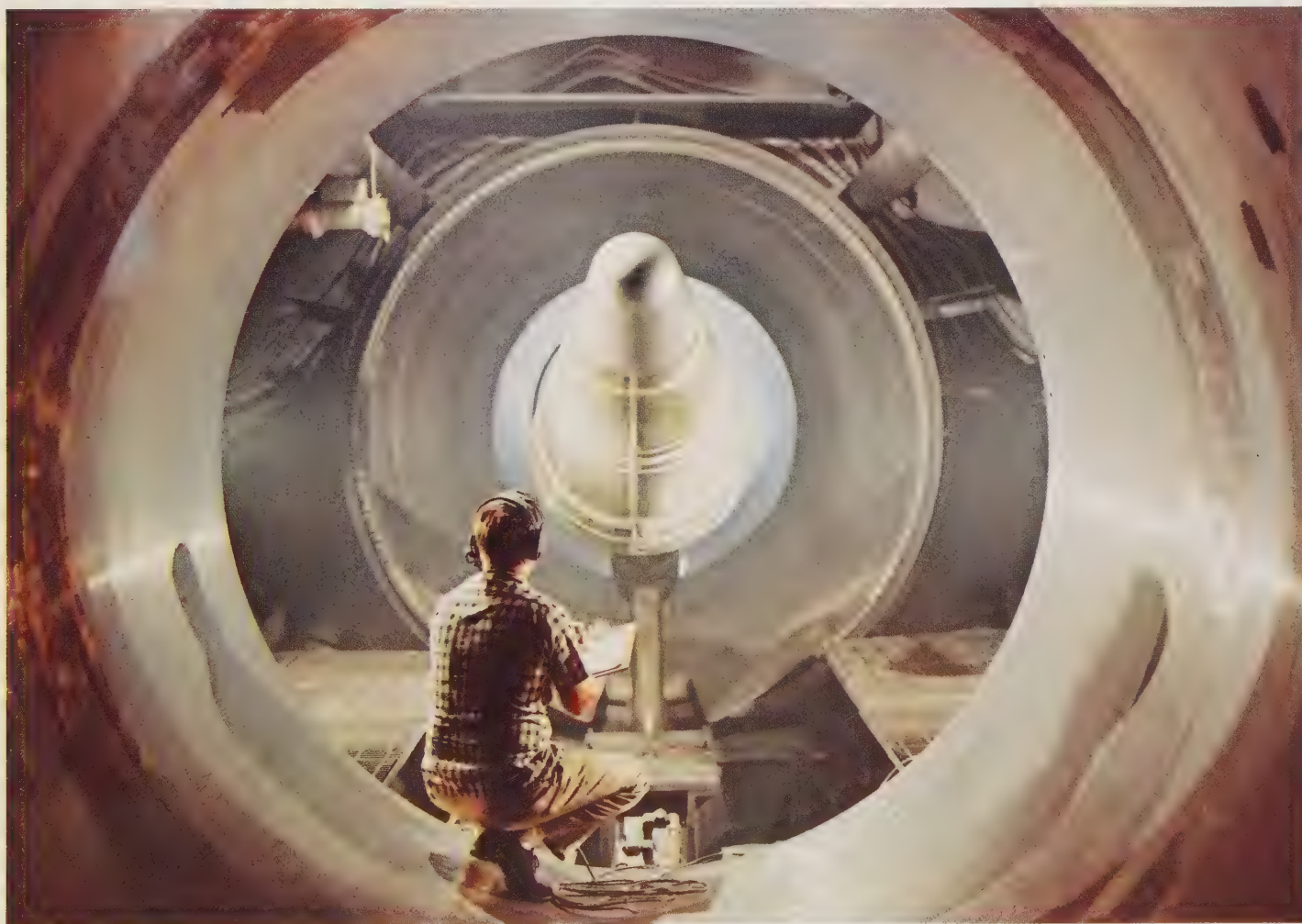
In the 8-foot test section of the Langley high-temperature structures tunnel, models are subjected to a Mach 7 gas flow provided by a huge methane burner.
