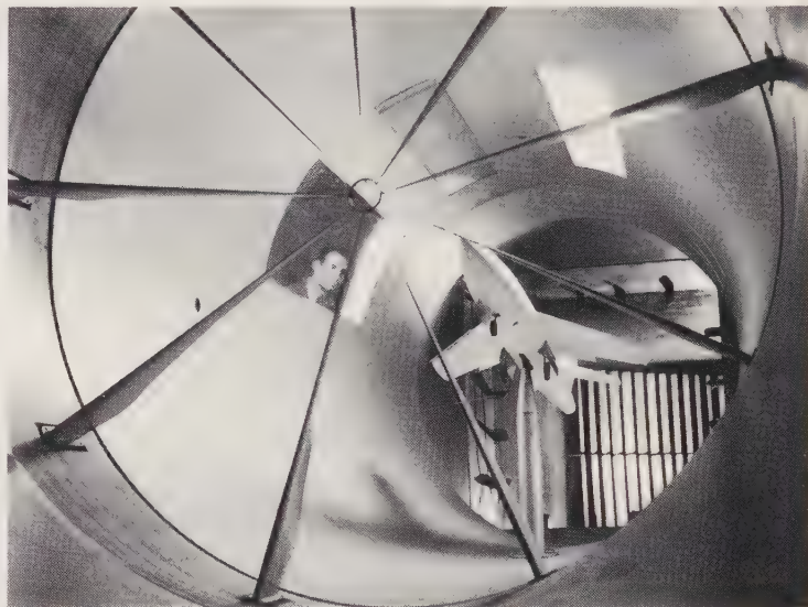
Inside the Langley stability tunnel, rim-driven rotating paddles set the air swirling to simulate the rolling action of the model.
