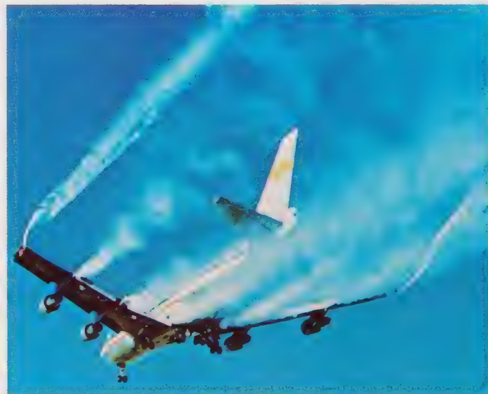
The selective deployment of spoilers and wing flaps on this Boeing 747 reduced the strength of the trailing vortices.
