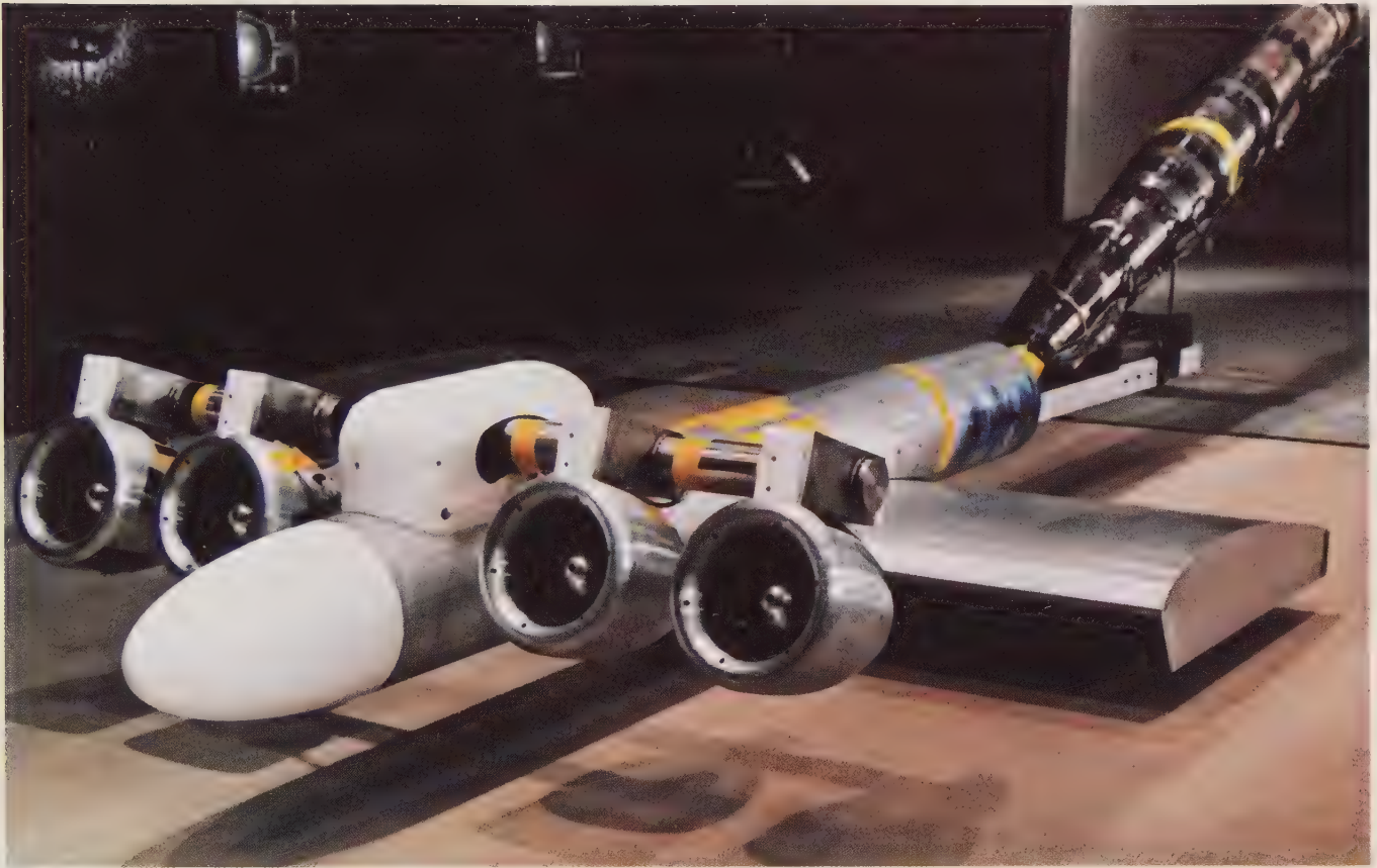
A model of a VTOL aircraft with tilting engines mounted over the moving ground board of the V/STOL wind tunnel.
