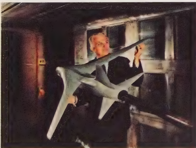
Wind tunnels provided crucial data in the development of the supercritical wing. (Left) Tunnel tests. (Right) Resulting aircraft.
