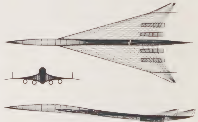
Three views of an SST configuration drawn entirely by a computer. Such analytical techniques proved inadequate for “off-design” portions of the SST mission, such as stability under various aerodynamic forces. Wind tunnel testing was necessary.
