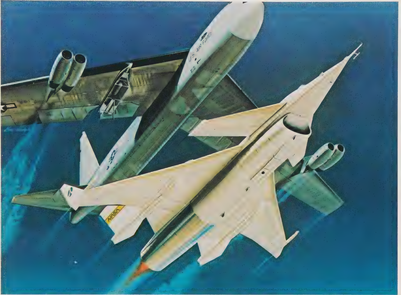
HiMAT is released from its B-52 mother ship in this artist's conception. (HiMAT = Highly Maneuverable Aircraft Technology.) Maneuverability is achieved by canard control surfaces.
