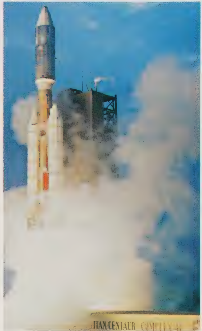
Viking was launched by a Titan-2 rocket. The bulging payload atop the cluster of three rockets generated complex shock waves as the launch vehicle pushed through the transonic range.
