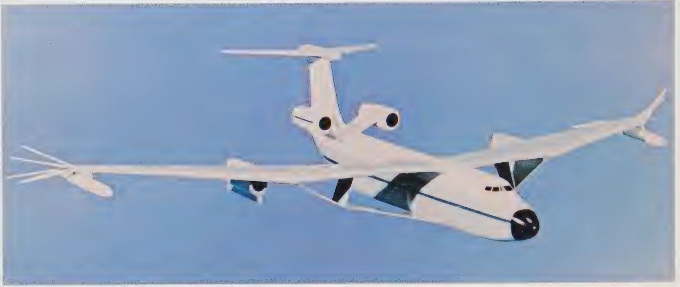
An idealized transport configuration with laminar flow control (LFC) applied to the wings, struts, engine nacelles, and fuselage. By reducing fuel consumption with LFC, payload fractions can be raised to about 30 percent, a large increase over current aircraft.
