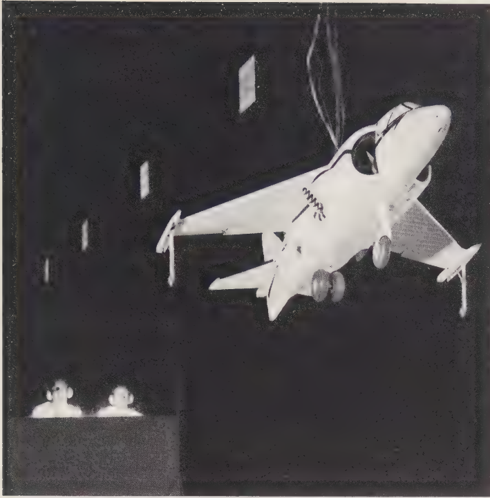
A powered model of the Harrier VTOL fighter flying in the Langley full-scale wind tunnel.
