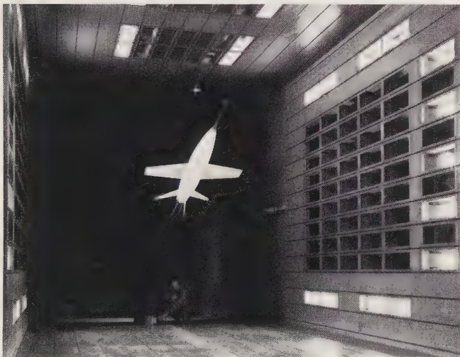
In 1955 the Ames 14-foot transonic tunnel began operations incorporating a "ventilated" wall.
