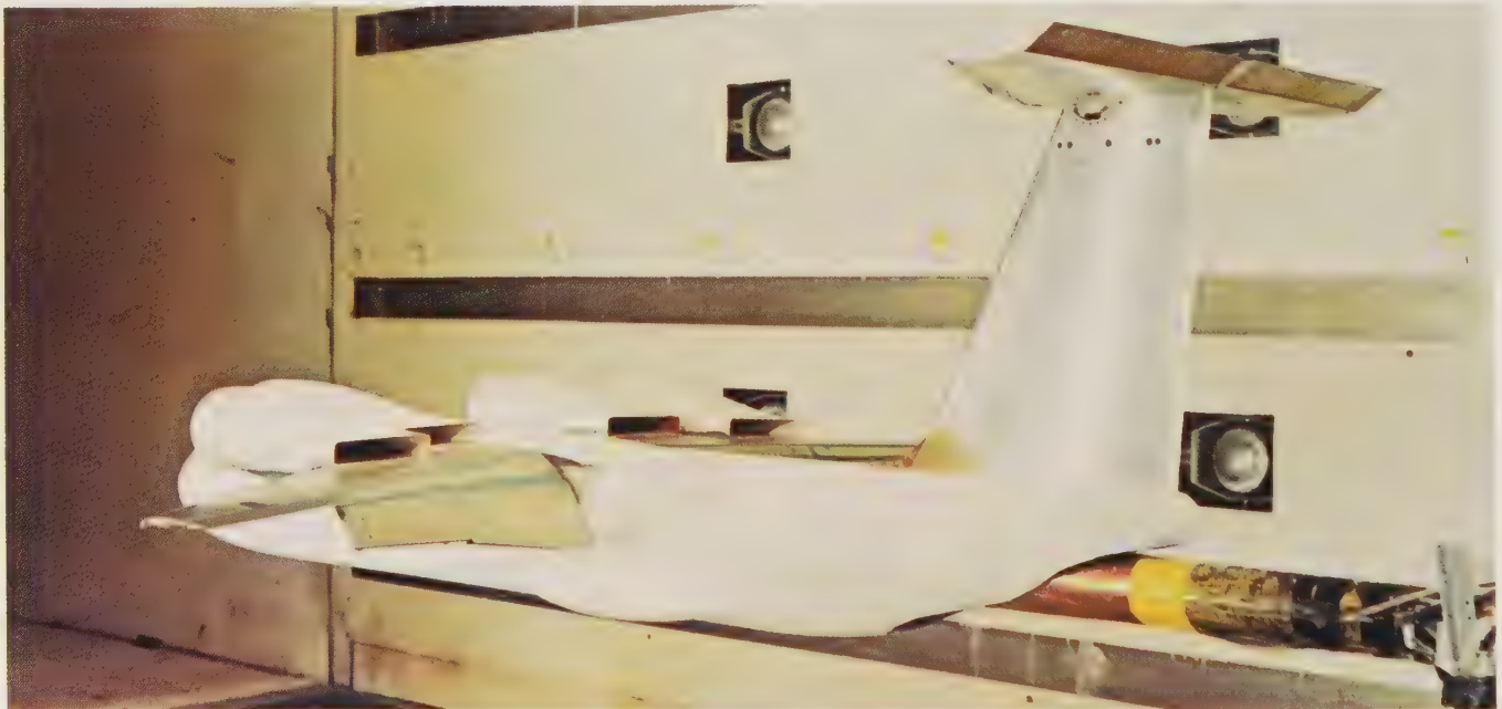
A model being tested in the Langley V/STOL tunnel employs upper-surface blowing over the large flaps to turn the engine jets downward for powered lift.
