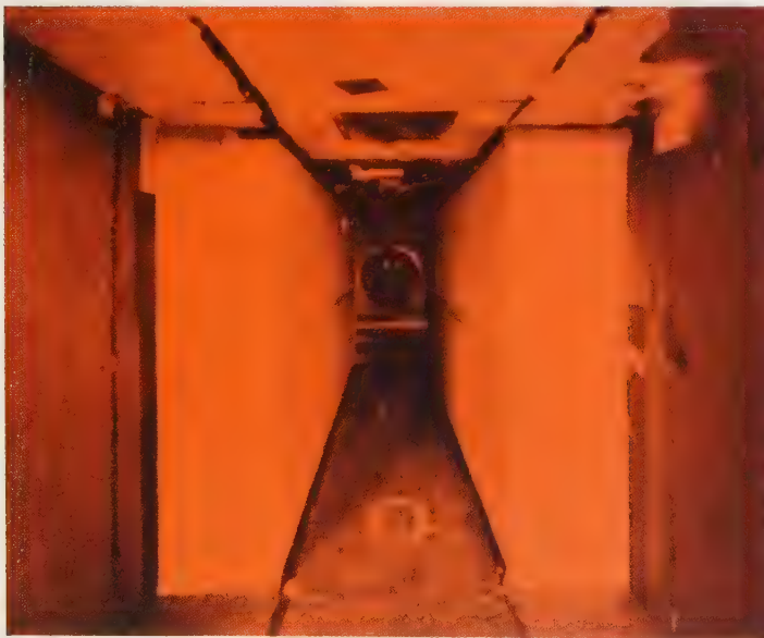
Albert Zahm's "air tunnel" built at Catholic University, Washington, DC, in 1901 with funds from an industrial sponsor. (Courtesy University of Notre Dame Archives)
