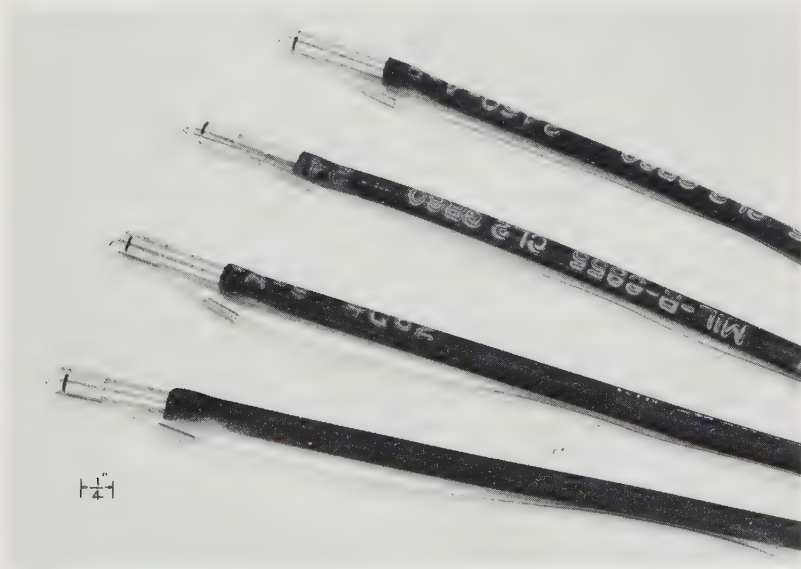
Fig. 15-9. Pneumatic sample collectors designed for ingesting dust and fine debris from the surface of the Moon or a planet. (Courtesy of the Jet Propulsion Laboratory)
