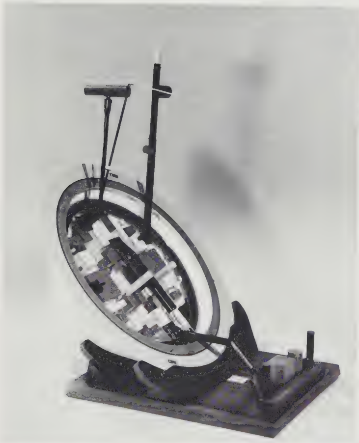
Fig. 10-37. A typical Mars, Voyager-class landing capsule. This design assumes atmospheric braking will be possible on Mars. (Courtesy of General Electric Co.)
