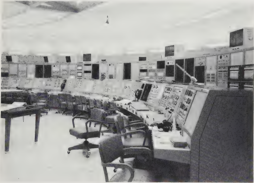
Fig. 8-9. Interior view of Blockhouse 37 at Cape Kennedy, showing some of the consoles and electronic equipment. (NASA photograph)
