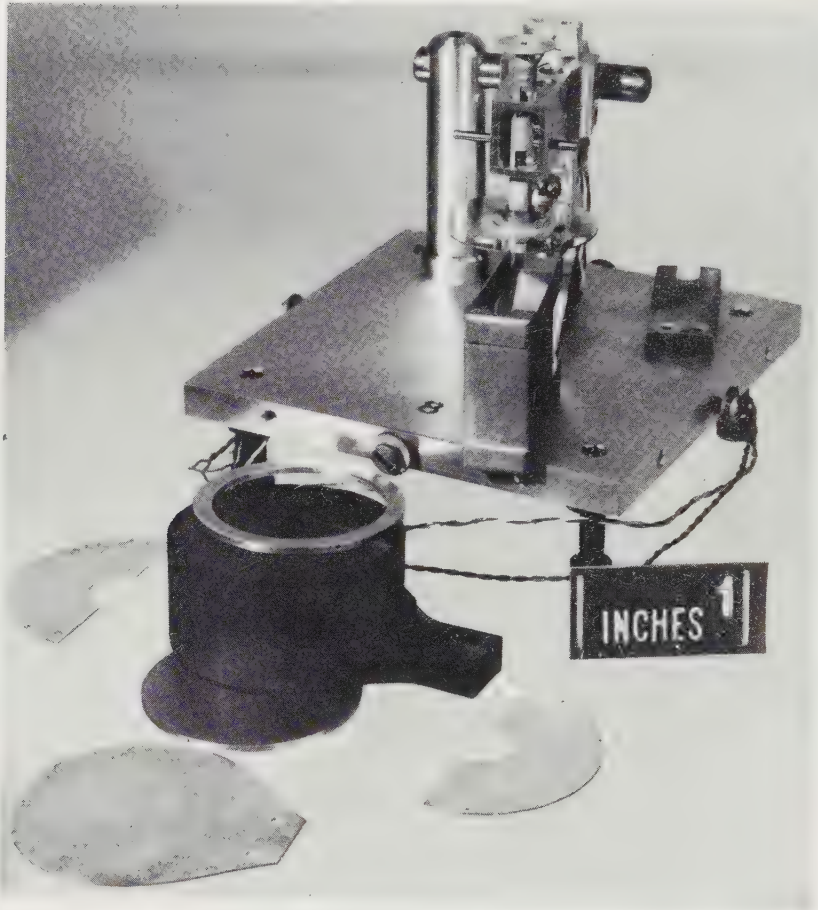
Fig. 13-61. Prototype of the Ames Research Center ballistic-pendulum micro-meteoroid detector. The sounding board is mounted on piezoelectric beams. (NASA photograph)
