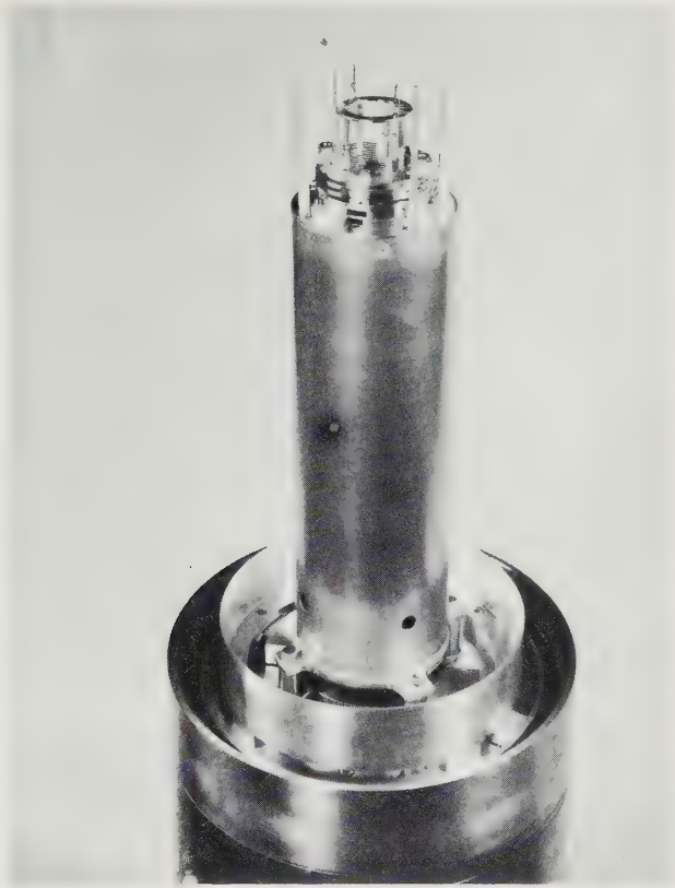
Fig. 14-18. A University of Michigan quadrupole mass spectrometer in a sounding-rocket configuration. (Courtesy of the University of Michigan)
