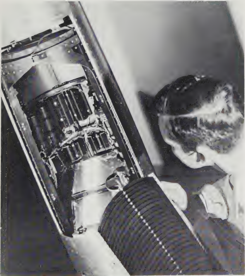
Fig. 14-13. The ultraviolet spectrometer of Fig 14-12 mounted in an Aerobee-III nose. (Courtesy of Perkin-Elmer Corp.)
