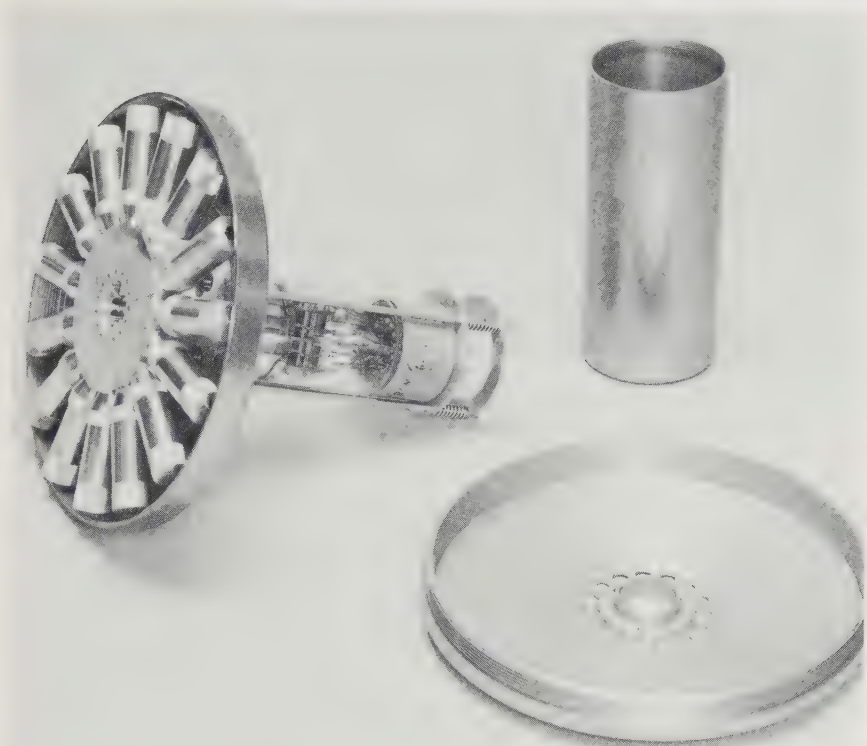
Fig. 16-13. One of the Multivator prototypes. This model shows fifteen reaction chambers and a photomultiplier tube, which is used with those chambers employing light signals. Dust and aerosol samples are blown into the radial chambers. (Courtesy of Stanford University)
