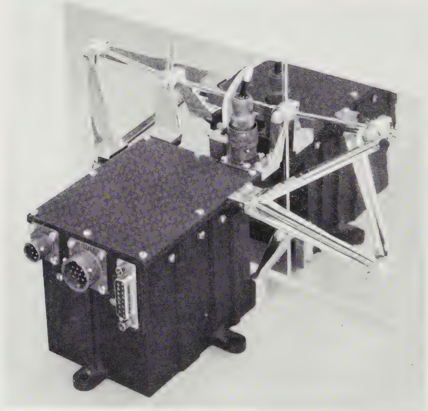
Fig. 13-57. Rear view of the Mariner-2, microphone-type micrometeoroid detector. (Ref. 13-59)
