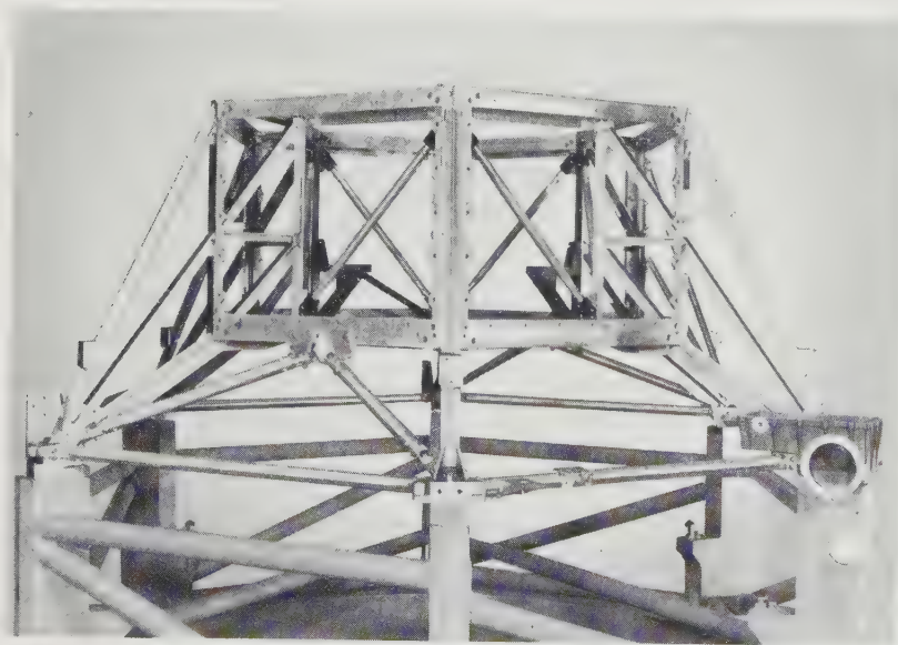
Fig. 10-35. Mariner 2 used a hexagonal frame as its basic structure. The six chassis shown in Fig. 10-34 are hinged to this structure for easy access. (Courtesy of the Jet Propulsion Laboratory)
