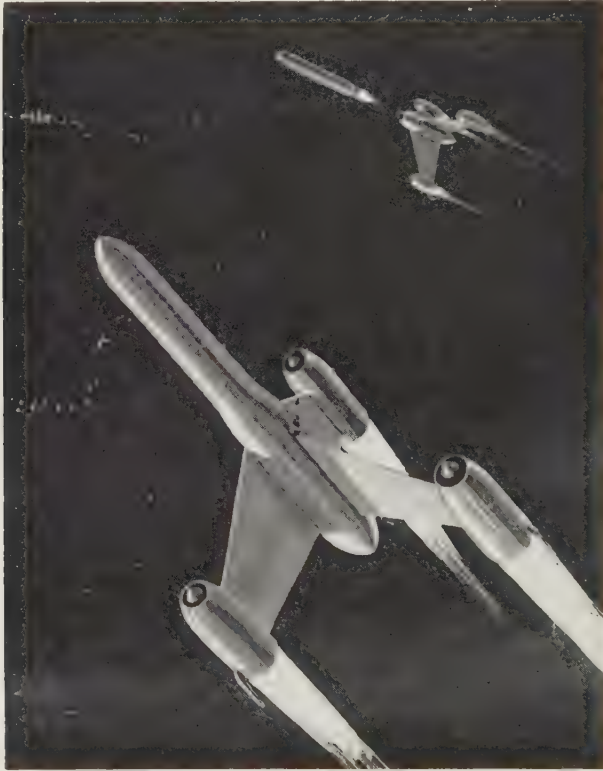
FIG. 5-5. A conceptual drawing of an air-breathing boost vehicle. Turbojet engines are located in the body of the vehicle and the three pods. The first stage may be detached, as shown in the upper portion of the illustration, landed, and used again. (General Electric Co.)
