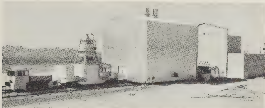
FIG. 5-18. The KIWI-A nuclear-rocket experimental engine at the Nevada test site. The KIWI-A was successfully tested in 1959. ( Los Alamos Scientific Laboratory, University of California. )
