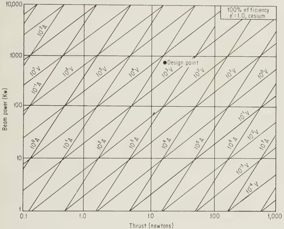
FIG. 6-14. Power-thrust curves for a cesium ion drive. The design point from Table 6-3 is indicated approximately.
