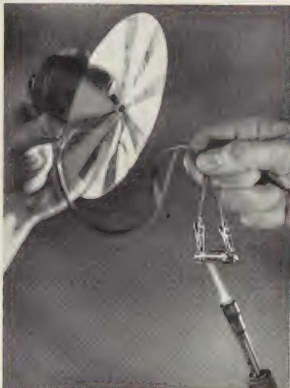
FIG. 4-29. Photograph of a vacuum type of thermionic converter. (General Electric Co.)
