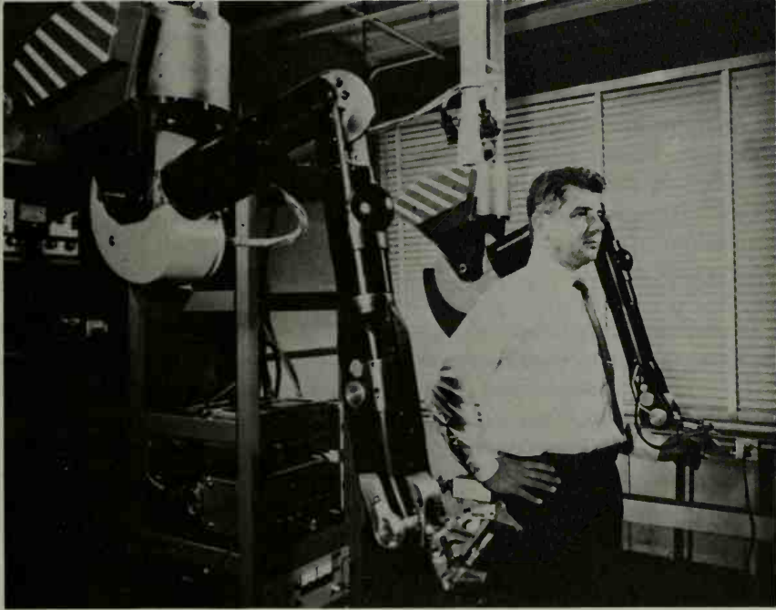
Figure 7.10 The Brookhaven electric master-slave arm. The slave arm is on the right. Compare with the ANL E4A, Fig. 5.16. (Courtesy of C. R. Flatau.)
