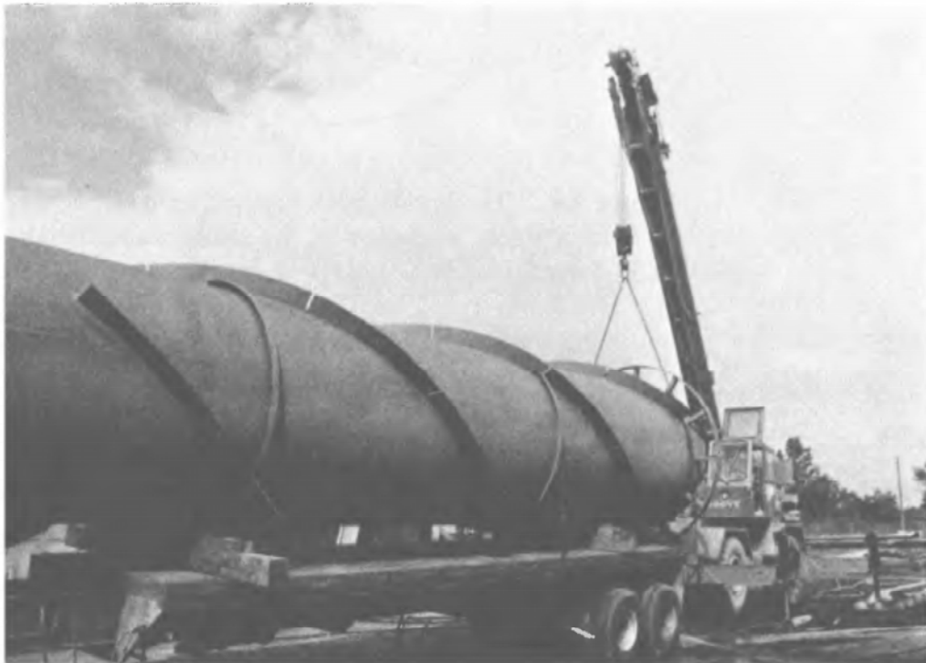
Figure 2.3. The metal strip, or strake, spirals around the smokestack on a helical path.
