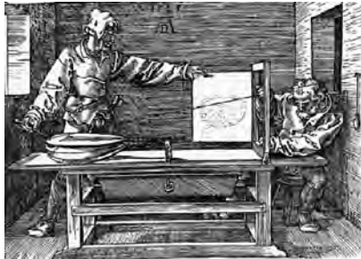
Figure 1 An artist using Dürer's perspective machine.
