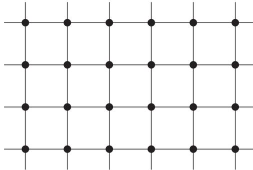
**FIGURE 13.16** A finite square lattice with  $n = 4$  rows and  $m = 6$  columns. In view of the periodic boundary conditions, sites on the leftmost column interact with sites on the rightmost column and the bottom row interacts with the top row.
