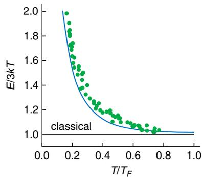
**FIGURE 8.10** Experimental results for the mean energy per particle divided by the equipartition value of  $3kT$  versus scaled temperature ( $T/T_F$ ) for ultracold  $^{40}\text{K}$  atoms in a harmonic trap compared to the theoretical Fermi gas value from equations (4) and (5). This shows the development of the Fermi degeneracy of the gas at low temperatures; from Jin (2002). Figure courtesy of the IOP. Reprinted with permission; copyright ©2002, American Institute of Physics.
