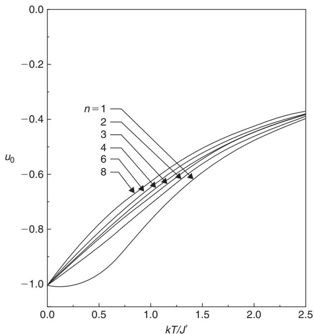
**FIGURE 13.6** The normalized energy  $u_0(= U_0/NnJ')$  of a one-dimensional chain as a function of the temperature parameter  $kT/J'$  for several values of  $n$  (after Stanley, 1969a,b). Note that for this *classical* model, the slopes as  $T \rightarrow 0$  are given by the equipartition theorem for  $n - 1$  degrees of freedom per spin.
