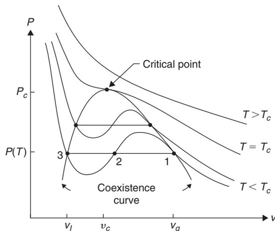
**FIGURE 12.3** The isotherms of a van der Waals system; those for  $T < T_c$  are “corrected” with the help of the Maxwell construction, thus leading to the coexistence curve at the top of which sits the critical point.
