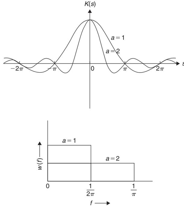
**FIGURE 15.7** The autocorrelation function  $K(s)$  and the power distribution function  $w(f)$  of a given variable  $y(t)$ ; the parameter  $a$  appears in terms of an arbitrary unit of  $(\text{time})^{-1}$ .
