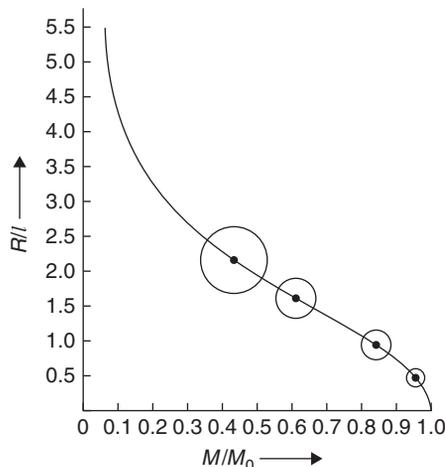
**FIGURE 8.11** The mass–radius relationship for white dwarfs (after Chandrasekhar, 1939). The masses are expressed in terms of the limiting mass  $M_0$  and the radii in terms of a characteristic length  $l$ , which is given by  $7.71\mu_e^{-1} \times 10^8 \text{ cm} \simeq 3.86 \times 10^8 \text{ cm}$ .
