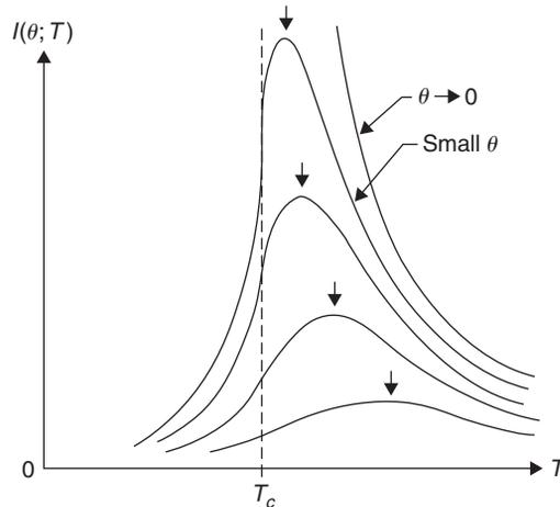
**FIGURE 12.13** Schematic plot of the elastic scattering intensity of neutrons scattered at an angle  $\theta$  from a magnetic system, such as iron, in the vicinity of the critical point  $T_c$ . The small arrows mark the smoothly rounded maxima (at fixed  $\theta$ ) which occur at a temperature  $T_{\max}(\theta)$  that approaches  $T_c$  as  $\theta \rightarrow 0$ .
