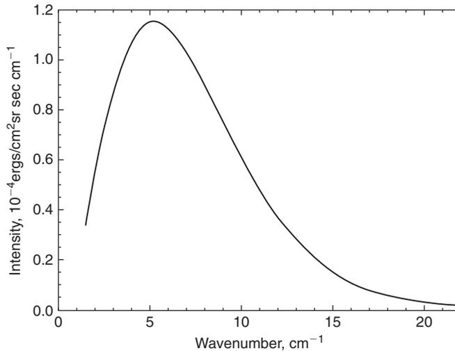
**FIGURE 9.2** Cosmic microwave background spectrum from COBE fit numerically to the Planck distribution with an average temperature  $T = 2.725 \pm 0.002 \text{ K}$ ; see equations (7.3.8) and (7.3.9), and Figure 7.13. The error bars at the 43 equally spaced frequencies from the Far Infrared Absolute Spectrophotometer (FIRAS) data are too small to be seen on this scale. Figure courtesy of NASA.
