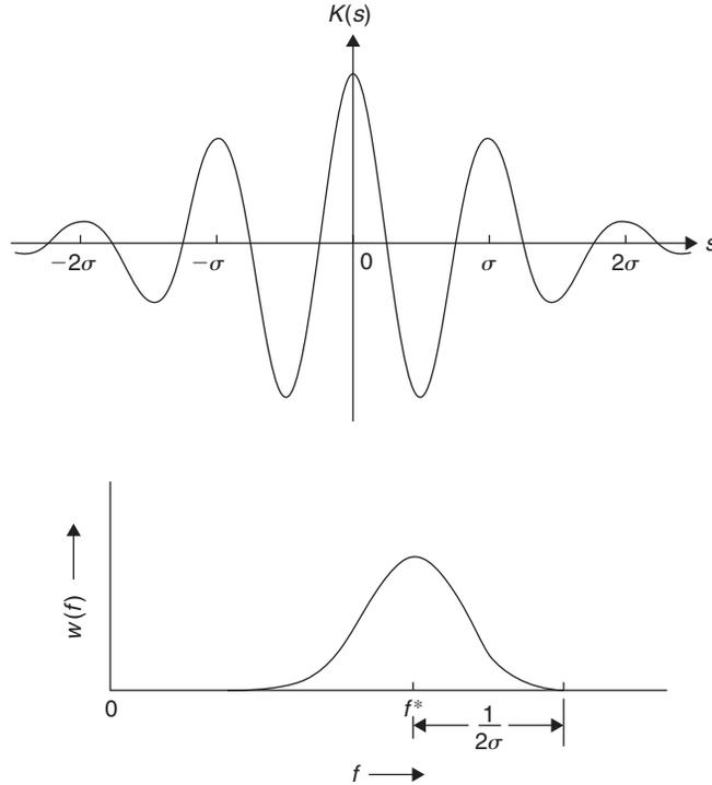
**FIGURE 15.9** The autocorrelation function  $K(s)$  and the power distribution function  $w(f)$  of a variable that has been filtered through a lightly damped tuned circuit, with mean frequency  $f^*$  and width  $\Delta f \sim (1/\sigma)$ .
