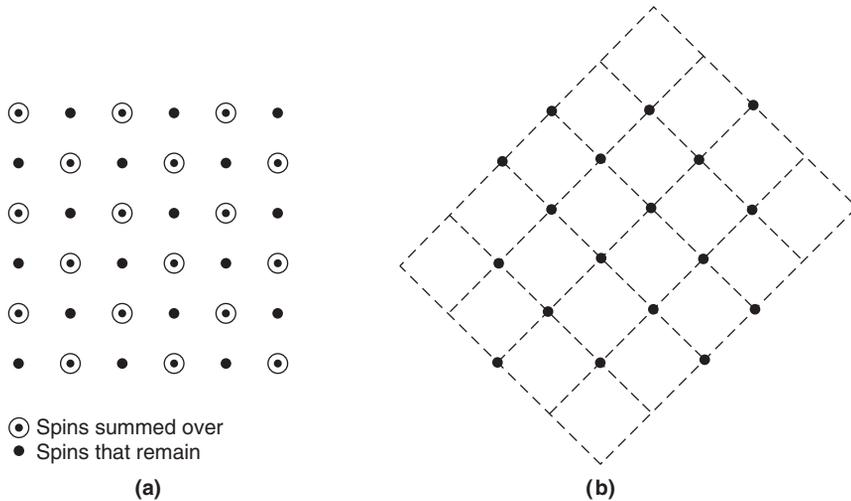
**FIGURE 14.2** A scale transformation by “decimation,” with  $l = \sqrt{2}$  and  $d = 2$ . The original lattice (a) has  $N (= 36)$  spins, the transformed one (b) has  $N' (= 18)$ ; the latter is yet to be rescaled (and rotated through an angle  $\pi/4$ ) so that it looks very much the same as the former, especially in the limit  $N, N' \rightarrow \infty$ .
