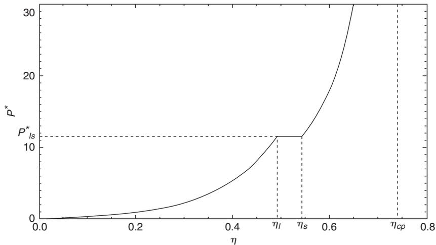
**FIGURE 16.3** Sketch of the equilibrium phase diagram for hard spheres in three dimensions. The horizontal axis is the volume fraction  $\eta = \pi n D^3 / 6$  and the vertical axis is the scaled pressure  $P^* = P D^3 / kT$ . There are two equilibrium phases: a low-density fluid phase for  $0 < \eta < \eta_l$  and a high-density solid phase for  $\eta_s < \eta < \eta_{cp}$ .
