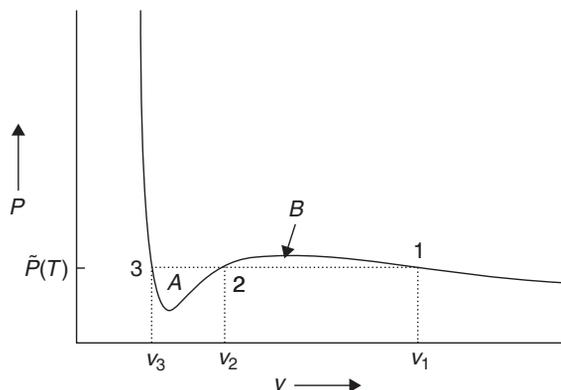
**FIGURE 12.2** An unphysical isotherm corrected with the help of the Maxwell construction; the horizontal line is such that the areas  $A$  and  $B$  are equal. The “corrected” isotherm corresponds to a phase transition, taking place at pressure  $\bar{P}(T)$ , with densities  $v_1^{-1}$  and  $v_3^{-1}$  of the respective phases.
