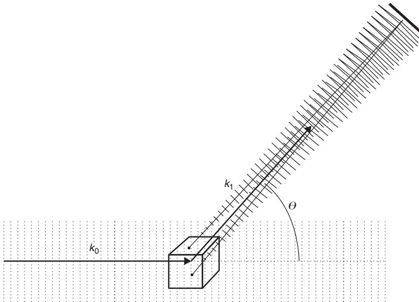
**FIGURE 10.7** Scattering from two particles. The incident wavevector is  $\mathbf{k}_0$ , the scattered wavevector toward the detector is  $\mathbf{k}_1$ , and the wavevector transfer is  $\mathbf{k} = \mathbf{k}_1 - \mathbf{k}_0$ . Since  $|\mathbf{k}_1| = |\mathbf{k}_0|$  for quasielastic scattering, the magnitude of the wavevector transfer is  $k = 2k_0 \sin(\theta/2)$ , where  $\theta$  is the angle between  $\mathbf{k}_0$  and  $\mathbf{k}_1$ .
