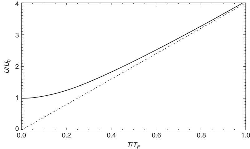
**FIGURE 8.9** Scaled internal energy ( $U/U_0$ ) versus scaled temperature ( $T/T_F$ ) for an ideal Fermi gas in a harmonic trap from equations (4) and (5). The dotted line is the corresponding classical result  $U(T) = 3NkT$ .
