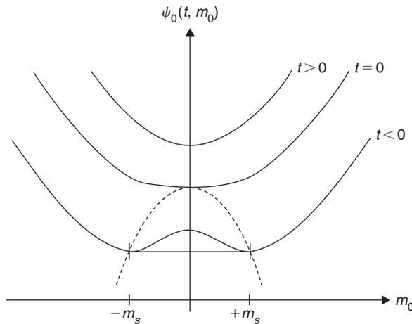
**FIGURE 12.12** The free energy  $\psi_0(t, m_0)$  of the Landau theory, shown as a function of  $m_0$ , for three different values of  $t$ . The dashed curve depicts spontaneous magnetization  $m_s(t)$ , while the horizontal line for  $t < 0$  provides the Maxwell construction.
