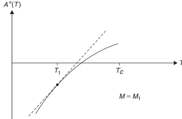
**FIGURE 12.11** The function  $A^*(T, M)$  of a magnetic system, with magnetization  $M$  fixed at  $M_1$ . The slope of this curve is  $S(T_c, 0) - S(T, M_1)$ , which is positive for all  $T \leq T_c$ .
