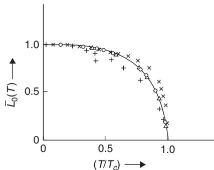
**FIGURE 12.7** The spontaneous magnetization of a Weiss ferromagnet as a function of temperature. The experimental points (after Becker) are for iron ( $\times$ ), nickel ( $\circ$ ), cobalt ( $\Delta$ ), and magnetite ( $+$ ).
