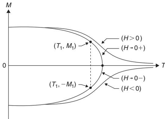
**FIGURE 12.10** Magnetization,  $M(T, H)$ , of a magnetic system for  $H > 0$ ,  $H < 0$ , and  $H \rightarrow 0$ . Here,  $M_1$  denotes the spontaneous magnetization of the system at a temperature  $T_1 < T_c$ .
