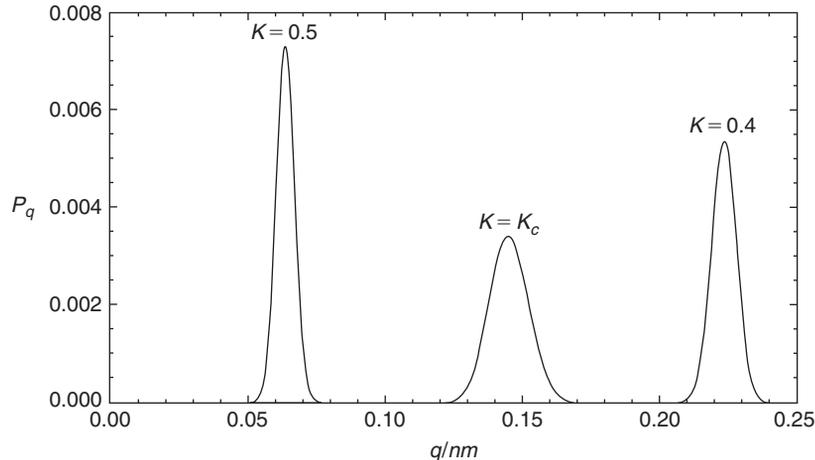
**FIGURE 13.20** The exact energy distribution  $P_q$  for the two-dimensional Ising model on a  $128 \times 128$  lattice for  $K = 0.4$ ,  $K = K_c \simeq 0.4407$ , and  $K = 0.5$ . The variance of the energy distribution is proportional to the specific heat, so is largest near  $K = K_c$ . Refer to Figure 13.17.
