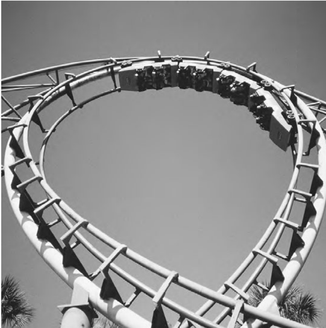
A CLOTHOID LOOP IN A ROLLER COASTER IN HAINES CITY, FLORIDA. AT THE TOP OF A LOOP, YOU FEEL LIGHTER THAN NORMAL; AT THE BOTTOM, YOU FEEL HEAVIER. ( The Purcell Team/Corbis. Reproduced by permission. )
