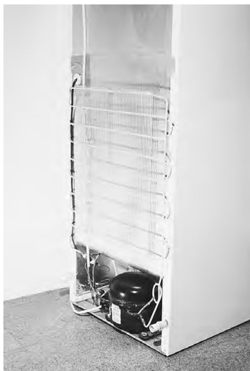
A REFRIGERATOR IS A TYPE OF REVERSE HEAT ENGINE THAT USES A COMPRESSOR, LIKE THE ONE SHOWN AT THE BACK OF THIS REFRIGERATOR, TO COOL THE REFRIGERATOR'S INTERIOR. (Ecoscene/Corbis. Reproduced by permission.)
