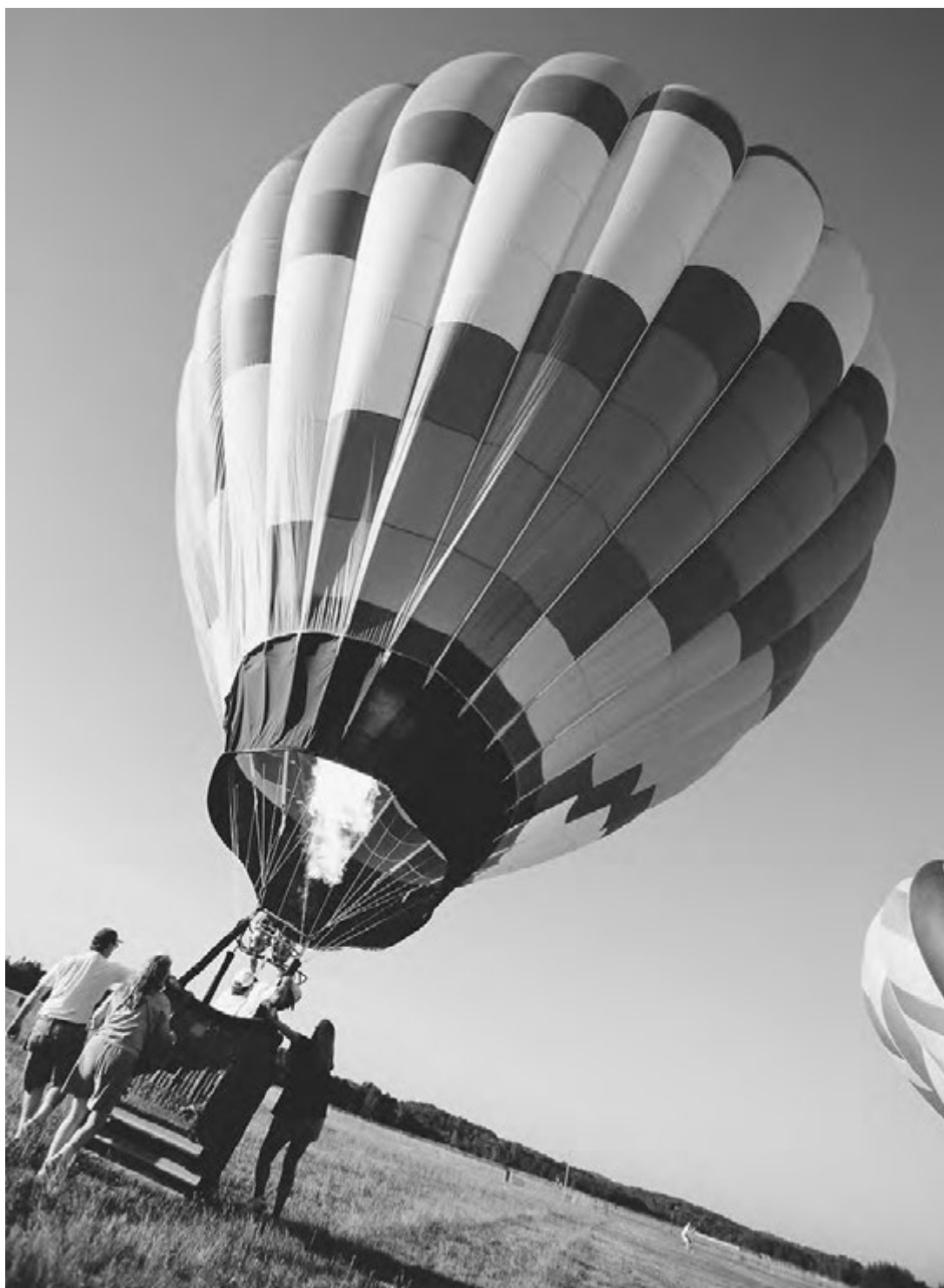
A HOT-AIR BALLOON FLOATS BECAUSE THE AIR INSIDE IT IS NOT AS DENSE THAN THE AIR OUTSIDE. THE WAY IN WHICH THE DENSITY OF THE AIR IN THE BALLOON IS REDUCED REFLECTS THE GAS LAWS. (Duomo/Corbis. Reproduced by permission.)
