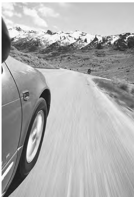
THE RAISED TREAD ON AN AUTOMOBILE'S TIRES, COUPLED WITH THE ROUGHENED ROAD SURFACE, PROVIDES SUFFICIENT FRICTION FOR THE DRIVER TO BE ABLE TO TURN THE CAR AND TO STOP. (Photograph by Martyn Goddard/Corbis. Reproduced by permission.)
