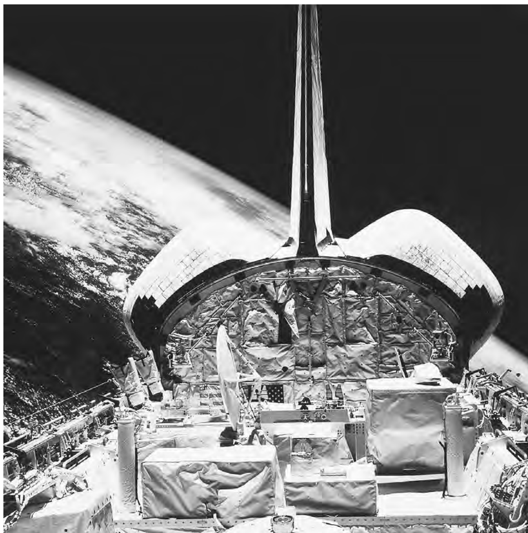
THE CARGO BAY OF THE SPACE SHUTTLE DISCOVERY, SHOWN JUST AFTER RELEASING A SATELLITE. ONCE RELEASED INTO THE FRICTIONLESS VACUUM AROUND EARTH, THE SATELLITE WILL MOVE INDEFINITELY AROUND EARTH WITHOUT NEED FOR THE MOTIVE POWER OF AN ENGINE. THE PLANET'S GRAVITY KEEPS IT AT A FIXED HEIGHT, AND AT THAT HEIGHT, IT COULD THEORETICALLY CIRCLE EARTH FOREVER. (Corbis. Reproduced by permission.)
