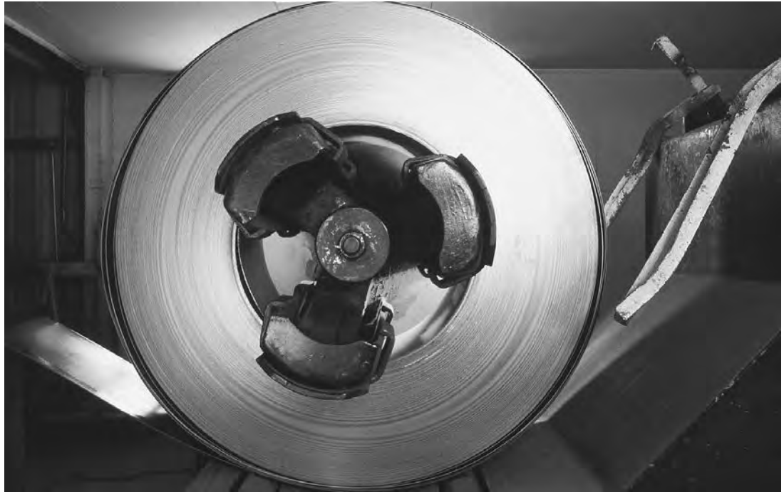
THE MACHINE PICTURED HERE ROLLS OVER STEEL IN ORDER TO BEND IT INTO PIPES. BECAUSE OF ITS ELASTIC NATURE, STEEL CAN BE BENT WITHOUT BREAKING. (Photograph by Vince Streano/Corbis. Reproduced by permission.)
