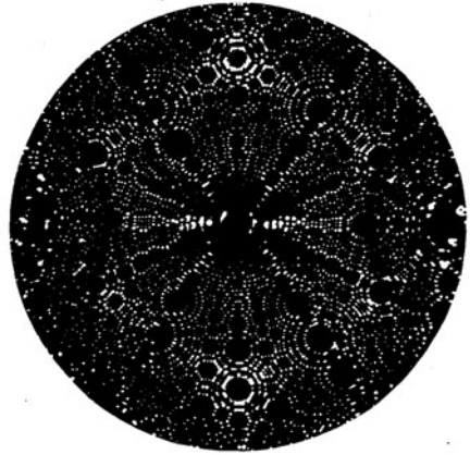
Figure 11.13. Field ion microscope image of a tungsten tip of radius \sim 400 \text{ \AA} . The original image had a magnification of 3 million. (Photo courtesy of T. Tsong.)
