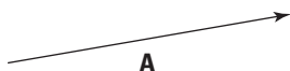
Figure 4-1: A vector, represented by an arrow, has both a direction and a magnitude.
