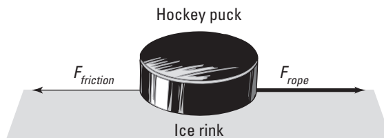
Figure 5-6: Pulling a heavy puck with a rope to exert equal force on both ends.
