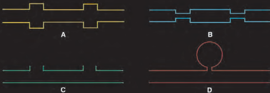
Acoustic filters typically used in air-handling systems. (A) and (B) Low-pass filters; (C) a high-pass filter; (D) a band-pass filter, which actually filters out vibrations within a narrow frequency range. Encyclopædia Britannica, Inc.
