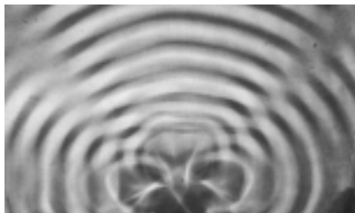
(c) A pretty good simulation of the single-slit pattern of figure (a), made by using three motors to produce overlapping ripples from three neighboring points in the water.
