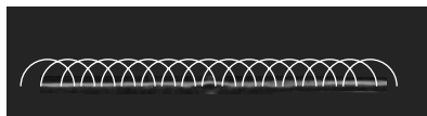
(c) If it was by itself, each of the parts would spread out as a circular ripple.
