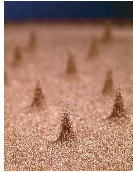
Figure 120 Oscillons formed by shaken bronze balls; horizontal size is about 2 cm (© Paul Umbanhowar)
