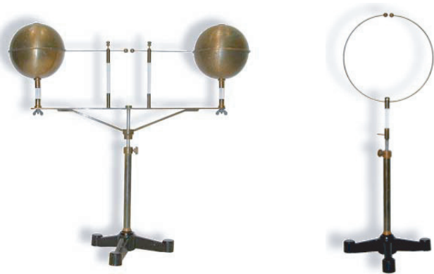
Figure 236 The first transmitter (left) and receiver (right) of electromagnetic (micro-) waves
