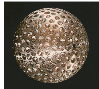
Figure 177 The Lageos satellites: metal spheres with a diameter of 60 cm, a mass of 407 kg and covered with 426 retroreflectors
