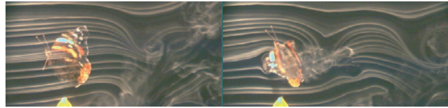
Figure 347 Vortices around a butterfly wing
