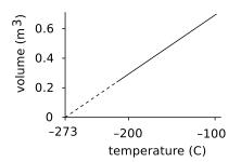
i / The volume of 1 kg of neon gas as a function of temperature (at standard pressure). Although neon would actually condense into a liquid at some point, extrapolating the graph to zero volume gives the same temperature as for any other gas: absolute zero. consistent with each other than gases in general. Continuing to search for consistency, we find that noble gases are more consistent with each other when their pressure is very low.
