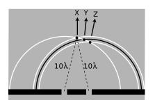
m / Constructive interference along the center-line.
