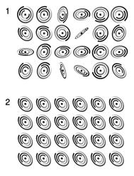
z / A schematic representation of an unmagnetized material, 1, and a magnetized one, 2.
