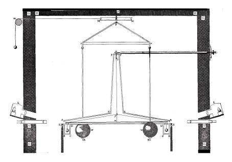
o / Cavendish's apparatus. The two large balls are fixed in place, but the rod from which the two small balls hang is free to twist under the influence of the gravitational forces.
