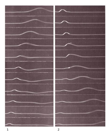
d/1. A wave in the lighter spring, where the wave speed is greater, travels to the left and is then partly reflected and partly transmitted at the boundary with the heavier coil spring, which has a lower wave speed. The reflection is inverted. 2. A wave moving to the right in the heavier spring is partly reflected at the boundary with the lighter spring. The reflection is uninverted.
