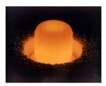
g / A pellet of plutonium-238 glows with its own heat. Its nuclear potential energy is being converted into heat, a form of kinetic energy. Pellets of this type are used as power supplies on some space probes.
