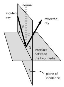
The two angles can be defined either with respect to the normal, like angles B and C in the figure, or with respect to the reflecting surface, like angles A and D. There is a convention of several hundred years' standing that one measures the angles with respect to the normal, but the rule about equal angles can logically be stated either as B=C or as A=D.
