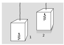
h / 1. A ray of light is emitted upward from the floor of the elevator. The elevator accelerates upward. 2. By the time the light is detected at the ceiling, the elevator has changed its velocity, so the light is detected with a Doppler shift.
