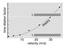
s / Time dilation measured with an atomic clock at low The theoretical curve. speeds. shown with a dashed line, is calculated from  $\chi = 1/\sqrt{1 - (v/c)^2}$ ; at these small velocities, the approximation of example 2 is an excellent one, so  $v \approx 1 + v^2/2c^2$ . and the graph is indistinguishable from a parabola. This graph corresponds to an extreme close-up view of the lower left corner of figure o. The error bars on the experimental points are about the same size as the dots.
