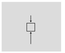
c / This does happen. The sum of the forces from the surrounding parts of the fluid is upward, canceling the downward force of gravity.
