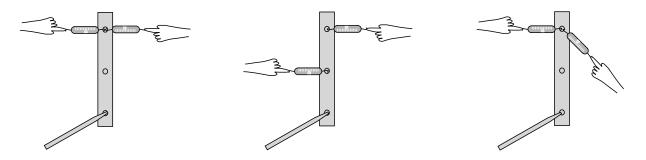
While one person holds the pencil which forms the axle for the ruler, the other members of the group pull on the scale and take readings. In each case, calculate the total torque on the ruler, and find out whether it equals zero to roughly within the accuracy of the experiment. Finish the calculations for each part before moving on to the next one.
