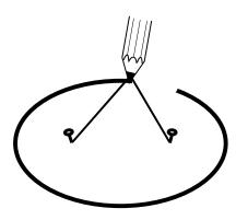
e / An ellipse can be constructed by tying a string to two pins and drawing like this with the pencil stretching the string taut. Each pin constitutes one focus of the ellipse.
