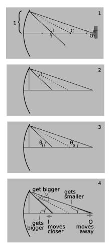
a / The relationship between the object's position and the image's can be expressed in terms of the angles  $\theta_o$  and  $\theta_i$ .
