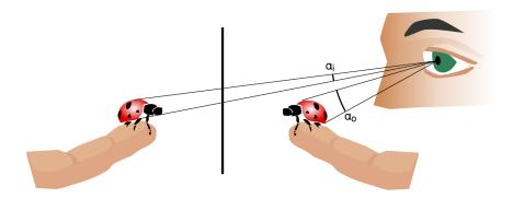
k / The person uses a mirror to get a view of both sides of the ladybug. Although the flat mirror has M = 1, it doesn't give an angular magnification of 1. The image is farther from the eye than the object, so the angular magnification  $M_a = \alpha_i / \alpha_o$  is less than one.
