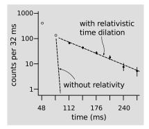
u / Example 4: Muons accelerated to nearly *c* undergo radioactive decay much more slowly than they would according to an observer at rest with respect to the muons. The first two data-points (unfilled circles) were subject to large systematic errors.
