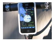
a / This Global Positioning System (GPS) system, running on a smartphone attached to a bike's handlebar, depends on Einstein's theory of relativity. Time flows at a different rates aboard a GPS satellite than it does on the bike, and the GPS software has to take this into account.
