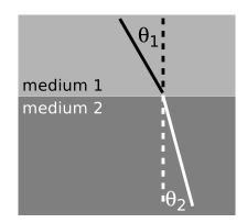
e / The angles  $\theta_1$  and  $\theta_2$  are related to each other, and also depend on the properties of the two media. Because refraction is time-reversal symmetric, there is no need to label the rays with arrowheads.
