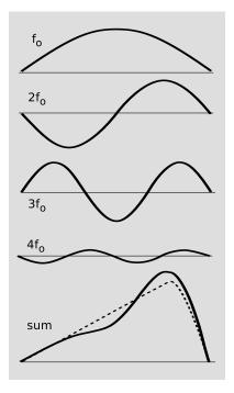
t / Using the sum of four sine waves to approximate the triangular initial shape of a plucked guitar string.
