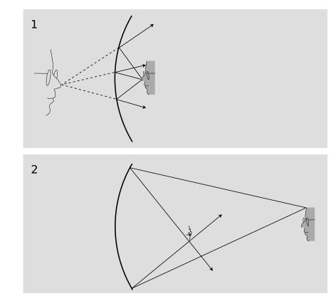
Here's what's happened. The mirror bends light rays inward, but when the object is very close to it, as in g/1, the rays coming from a
