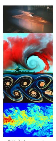
q / Fluid friction depends on the fluid's pattern of flow, so it is more complicated than friction between solids, and there are no simple, universally applicable formulas to calculate it. From top to bottom: supersonic wind tunnel, vortex created by a crop duster, series of vortices created by a single object, turbulence.
