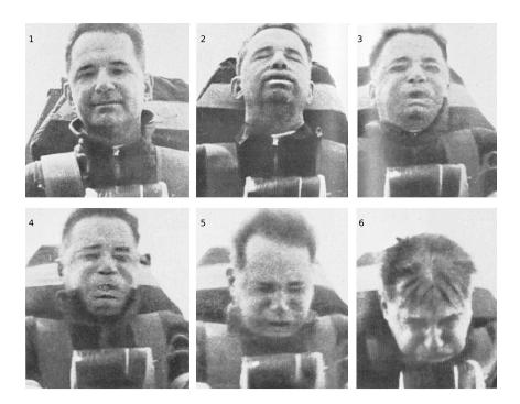
u / This Air Force doctor volunteered to ride a rocket sled as a medical experiment. The obvious effects on his head and face are not because of the sled's speed but because of its rapid *changes* in speed: increasing in 2 and 3, and decreasing in 5 and 6. In 4 his speed is greatest, but because his speed is not increasing or decreasing very much at this moment, there is little effect on him.
