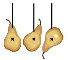
e / No matter what point you hang the pear from, the string lines up with the pear's center of mass. The center of mass can therefore be defined as the intersection of all the lines made by hanging the pear in this way. Note that the X in the figure should not be interpreted as implying that the center of mass is on the surface — it is actually inside the pear.
