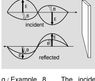
q / Example 8. The incident and reflected waves are drawn offset from each other for clarity, but are actually on top of each other so that their fields superpose.
