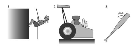
o / 1. The cliff's normal force on the climber's feet. 2. The track's static frictional force on the wheel of the accelerating dragster. 3. The ball's normal force on the bat.
