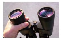
m / Seen from this angle, the optical coating on the lenses of these binoculars appears purple and green. (The color varies depending on the angle from which the coating is viewed, and the angle varies across the faces of the lenses because of their curvature.)
