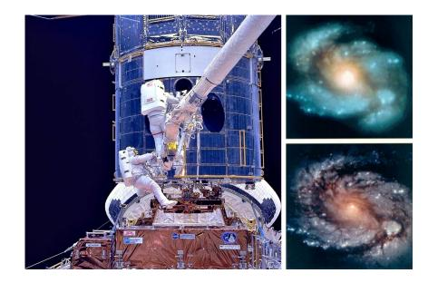
I/ The Hubble Space Telescope was placed into orbit with faulty optics in 1990. Its main mirror was supposed to have been nearly parabolic, since it is an astronomical telescope, meant for producing images of objects at infinity. However, contractor Perkin Elmer had delivered a faulty mirror, which produced aberrations. The large photo shows astronauts putting correcting mirrors in place in 1993. The two small photos show images produced by the telescope before and after the fix.
