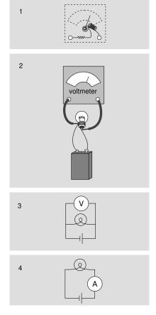
u / 1. A simplified diagram of how a voltmeter works. 2. Measuring the voltage difference across a lightbulb. 3. The same setup drawn in schematic form. 4. The setup for measuring current is different.
