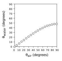
g / The relationship between the angles in refraction.
