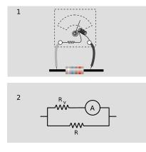
z / A voltmeter is really an ammeter with an internal resistor. When we measure the voltage difference across a resistor, 1, we are really constructing a parallel resistance circuit, 2.
