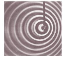
v / The pattern of waves made by a point source moving to the right across the water. Note the shorter wavelength of the forward-emitted waves and the longer wavelength of the backward-going ones. forward-emitted waves is shortened by an amount  $v_s T$  equal to the distance traveled by the source over the course of one period. Using the definition f = 1/T and the equation  $v = f\lambda$ , we find for the wavelength of the Doppler-shifted wave the equation
