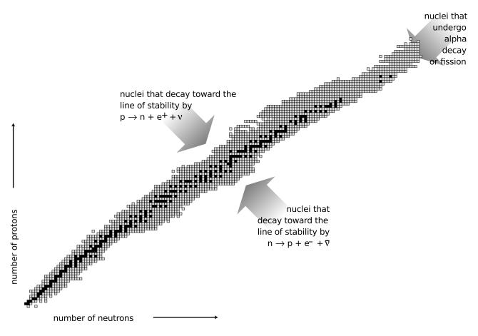
ac / The known nuclei, represented on a chart of proton number versus neutron number. Note the two nuclei in the bottom row with zero protons.
