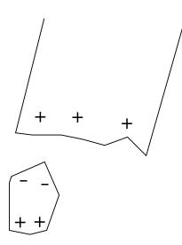
c / The paper has zero total charge, but it does have charged particles in it that can move.
