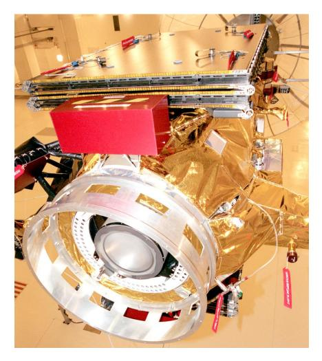
a / The ion drive engine of the NASA Deep Space 1 probe, shown under construction (left) and being tested in a vacuum chamber (right) prior to its October 1998 launch. Intended mainly as a test vehicle for new technologies, the craft nevertheless carried out a successful scientific program that included a flyby of a comet.
