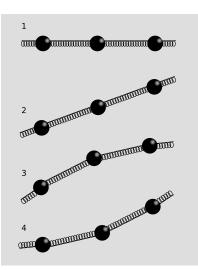
m / A continuous string can be modeled as a series of discrete masses connected by springs.
