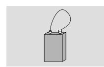
a / Short-circuiting а battery. Warning: you can burn yourself this way or start a fire! If you want to try this, try making the connection only very briefly, use a low-voltage battery, and avoid touching the battery or the wire, both of which will get hot.
