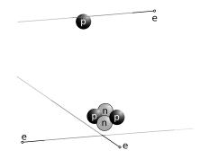
w / Examples of the construction of atoms: hydrogen (top) and helium (bottom). On this scale, the electrons' orbits would be the size of a college campus.
