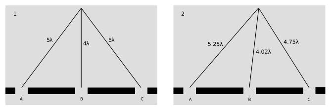
u / 1. There is a bright central maximum. 2. At this point just off the central maximum, the path lengths traveled by the three waves have changed.
