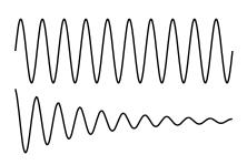
b / Friction has the effect of pinching the x - t graph of a vibrating object.
