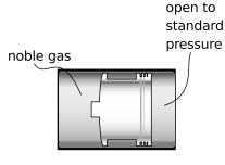
h / A simplified version of an ideal gas thermometer. The whole instrument is allowed to come into thermal equilibrium with the substance whose temperature is to be measured, and the mouth of the cylinder is left open to standard pressure. The volume of the noble gas gives an indication of temperature.
