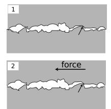
j / A model that correctly explains many properties of friction. The microscopic bumps and holes in two surfaces dig into each other.
