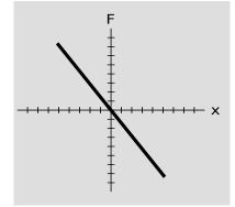
g / The force exerted by an ideal spring, which behaves exactly according to Hooke's law.
