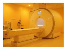
m / A medical MRI scanner, which uses superconductors.
