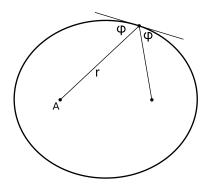
ad / Proof that the two angles labeled  $\phi$  are in fact equal: The definition of an ellipse is that the sum of the distances from the two foci stays constant. If we move a small distance  $\ell$  along the ellipse, then one distance shrinks by an amount  $\ell \cos \phi_1$ , while the other grows by  $\ell \cos \phi_2$ . These are equal, so  $\phi_1 = \phi_2$ .
