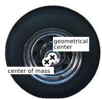
h / An improperly balanced wheel has a center of mass that is not at its geometric center. When you get a new tire, the mechanic clamps little weights to the rim to balance the wheel.
