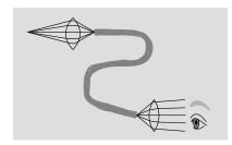
I/A simplified drawing of a surgical endoscope. The first lens forms a real image at one end of a bundle of optical fibers. The light is transmitted through the bundle, and is finally magnified by the eyepiece.
