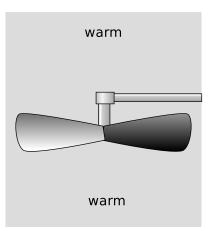
I / If the temperature of the air is first allowed to become uniform, then no mechanical energy can be extracted. The same amount of heat energy is present, but it is no longer accessible for doing mechanical work.
