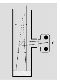
h / A Newtonian telescope being used with a camera.
