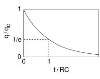
o / Over a time interval RC, the charge on the capacitor is reduced by a factor of e.
