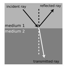
d / The incident, reflected, and transmitted (refracted) rays all lie in a plane that includes the normal (dashed line).
