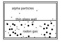
m / A simplified version of Rutherford's 1908 experiment, showing that alpha particles were doubly ionized helium atoms.
