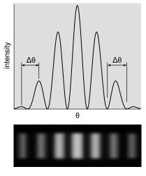
r / Interpretation of the angular spacing  $\Delta \theta$  in example 3. It can be defined either from maximum to maximum or from minimum to minimum. Either way, the result is the same. It does not make sense to try to interpret  $\Delta \theta$ as the width of a fringe; one can see from the graph and from the image below that it is not obvious either that such a thing is well defined or that it would be the same for all fringes.
