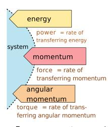
n / Energy, momentum, and angular momentum can be transferred. The rates of transfer are called power, force, and torque. It is possible to have a zero total torque with a nonzero total force. An airplane with four jet engines, o, would be designed so that their forces are balanced on the left and right. Their forces are all in the same direction, but the clockwise torques of two of the engines are canceled by the counterclockwise torques of the other two, giving zero total torque.
