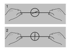
When the circuit is iny / 1. complete, no current flows through the wire, and the magnet is unaffected. It points in the direction of the Earth's magnetic field. 2. The circuit is completed, and current flows through the wire. The wire has a strong effect on the magnet, which turns almost perpendicular to it. If the earth's field could be removed entirely, the compass would point exactly perpendicular to the wire; this is the direction of the wire's field.
