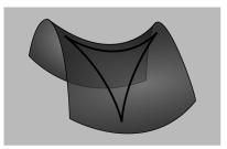
e / A triangle in a space with negative curvature has angles that add to less than  $180^\circ.$
