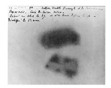
I / Becquerel's photographic plate. In the exposure at the bottom of the image, he has found that he could absorb the radiations, casting the shadow of a Maltese cross that was placed between the plate and the uranium salts. traveled in a straight line., so that it must have been some kind of ray rather than, e.g., the seepage of chemicals through the paper. He used the word "radiations," since the effect radiated out from the uranium salt.
