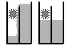
q / Entropy can be understood using the metaphor of a water wheel. Letting the water levels equalize is like letting the entropy maximize. Taking water from the high side and putting it into the low side increases the entropy. Water levels in this metaphor correspond to temperatures in the actual definition of entropy. Entropy is additive.
