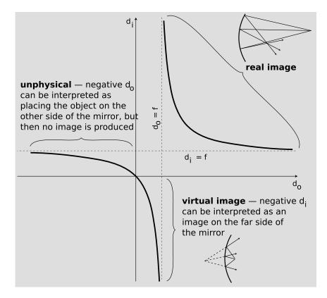
To analyze the distance equation, let's look at a graph of  $d_i$  as a function of  $d_o$ . The branch on the upper right corresponds to the case of a real image. Strictly speaking, this is the only part of the graph that we've proven corresponds to reality, since we never did any geometry for other cases, such as virtual images. As discussed in the previous section, making  $d_o$  bigger causes  $d_i$  to become smaller, and vice-versa.
