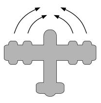
o / The plane's four engines produce zero total torque but not zero total force.
