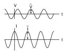
$q\,/\,In$  a capacitor, the current is  $90^\circ$  ahead of the voltage in phase.
