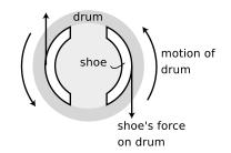
k / Because the force is in the opposite direction compared to the motion, the brake shoe does negative work on the drum, i.e., accepts energy from it in the form of heat.
