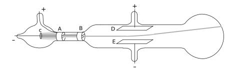
the angle through which the charged plates bent the beam. The electric force acting on a cathode ray particle while it was between the plates was
