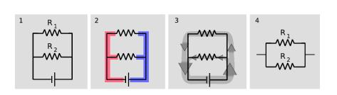
x / 1. Two resistors in parallel. 2. There are two constant-voltage areas. 3. The current that comes out of the battery splits between the two resistors, and later reunites. 4. The two resistors in parallel can be treated as a single resistor with a smaller resistance value.
