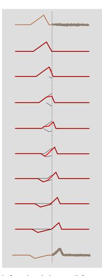
j / A pulse being partially reflected and partially transmitted at the boundary between two strings in which the speed of waves is different. The top drawing shows the pulse heading to the right, toward the heavier string. For clarity, all but the first and last drawings are schematic. Once the reflected pulse begins to emerge from the boundary, it adds together with the trailing parts of the incident pulse. Their sum, shown as a wider line, is what is actually observed.
