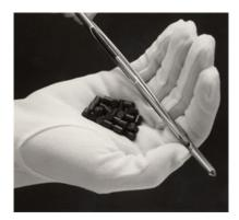
n / These pellets of uranium fuel will be inserted into the metal fuel rod and used in a nuclear reactor. The pellets emit alpha and beta radiation, which the gloves are thick enough to stop.
