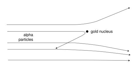
q / Alpha particles being scattered by a gold nucleus. On this scale, the gold atom is the size of a car, so all the alpha particles shown here are ones that just happened to come unusually close to the nucleus. For these exceptional alpha particles, the forces from the electrons are unimportant, because they are so much more distant than the nucleus.
