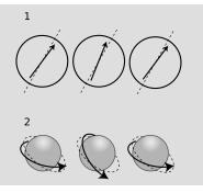
h / Example 14. 1. A compass needle vibrates about the equilibrium position under the influence of the earth's magnetic forces. 2. The orientation of a proton's spin vibrates around its equilibrium direction under the influence of the magnetic forces coming from the surrounding electrons and nuclei.
