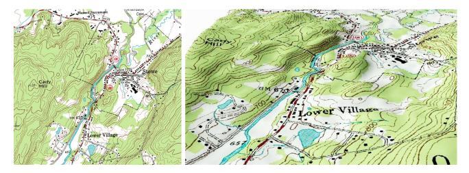
t / Left: A topographical map of Stowe, Vermont. From one constant-height line to the next is a height difference of 200 feet. Lines far apart, as in the lower village, indicate relatively flat terrain, while lines close together, like the ones to the west of the main town, represent a steep slope. Streams flow downhill, perpendicular to the constant-height lines. Right: The same map has been redrawn in perspective, with shading to suggest relief.
