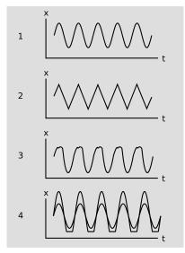
f / Sinusoidal and non-sinusoidal vibrations.
