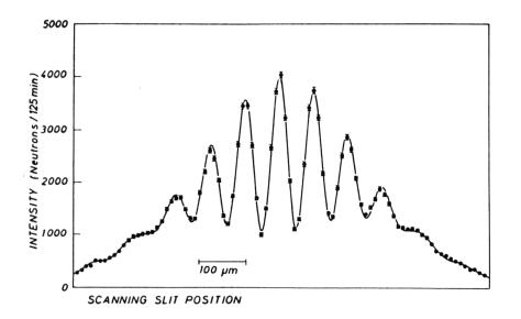
a / A double-slit interference pattern made with neutrons. (A. Zeilinger, R. Gähler, C.G. Shull, W. Treimer, and W. Mampe, Reviews of Modern Physics, Vol. 60, 1988.)
