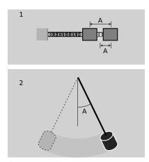
e / 1. The amplitude of the vibrations of the mass on a spring could be defined in two different ways. It would have units of distance. 2. The amplitude of a swinging pendulum would more naturally be defined as an angle.
