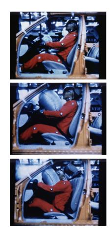
m / The airbag increases  $\Delta t$  so as to reduce  $F = \Delta p / \Delta t$ .
