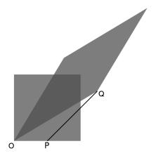
w / At event O, the source and the receiver are on top of each other, so as the source emits a wave crest, it is received without any time delay. At P, the source emits another wave crest, and at Q the receiver receives it.
