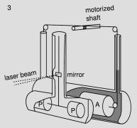
A balance that meaar / 1. sures the gravitational attraction between masses M and m. (See section 10.5 for a more detailed description.) When the two masses M are inserted, the fiber twists. 2. A simplified diagram of Kreuzer's modification. The moving teflon mass is submerged in a liquid with nearly the same Kreuzer's actual density. 3. apparatus.
