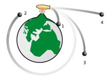
k / An imaginary cannon able to shoot cannonballs at very high speeds is placed on top of an imaginary, very tall mountain that reaches up above the atmosphere. Depending on the speed at which the ball is fired, it may end up in a tightly curved elliptical orbit, 1, a circular orbit, 2, a bigger elliptical orbit, 3, or a nearly straight hyperbolic orbit, 4.
