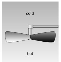
k / The temperature difference between the hot and cold parts of the air can be used to extract mechanical energy, for example with a fan blade that spins because of the rising hot air currents.
