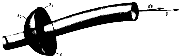
Figure 2.28. Geometry for deriving the point form of Ampere's law (Maxwell's equation).
