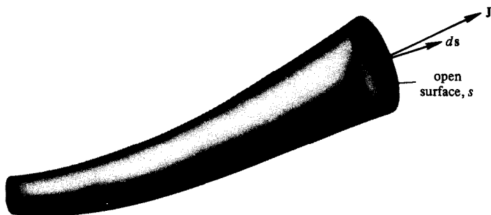
Figure 2.17. General current density \mathbf{J} over a cross section (open surface) s .
