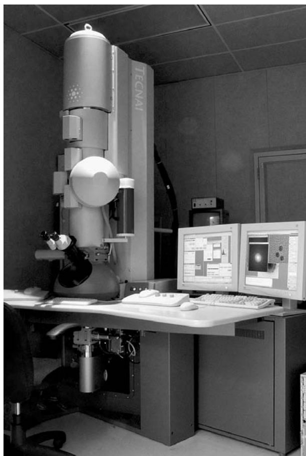
The National Center for Electron Microscopy houses this microscope with a 2048x2048 CCD camera.
