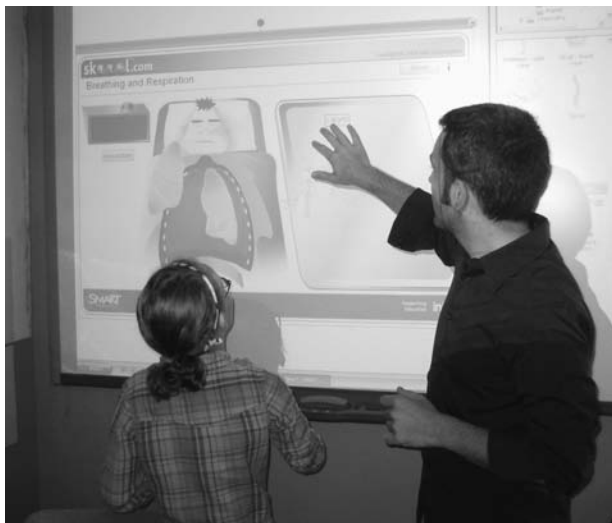
A projector displays video output on the SMART board, which acts as a large touch screen.
