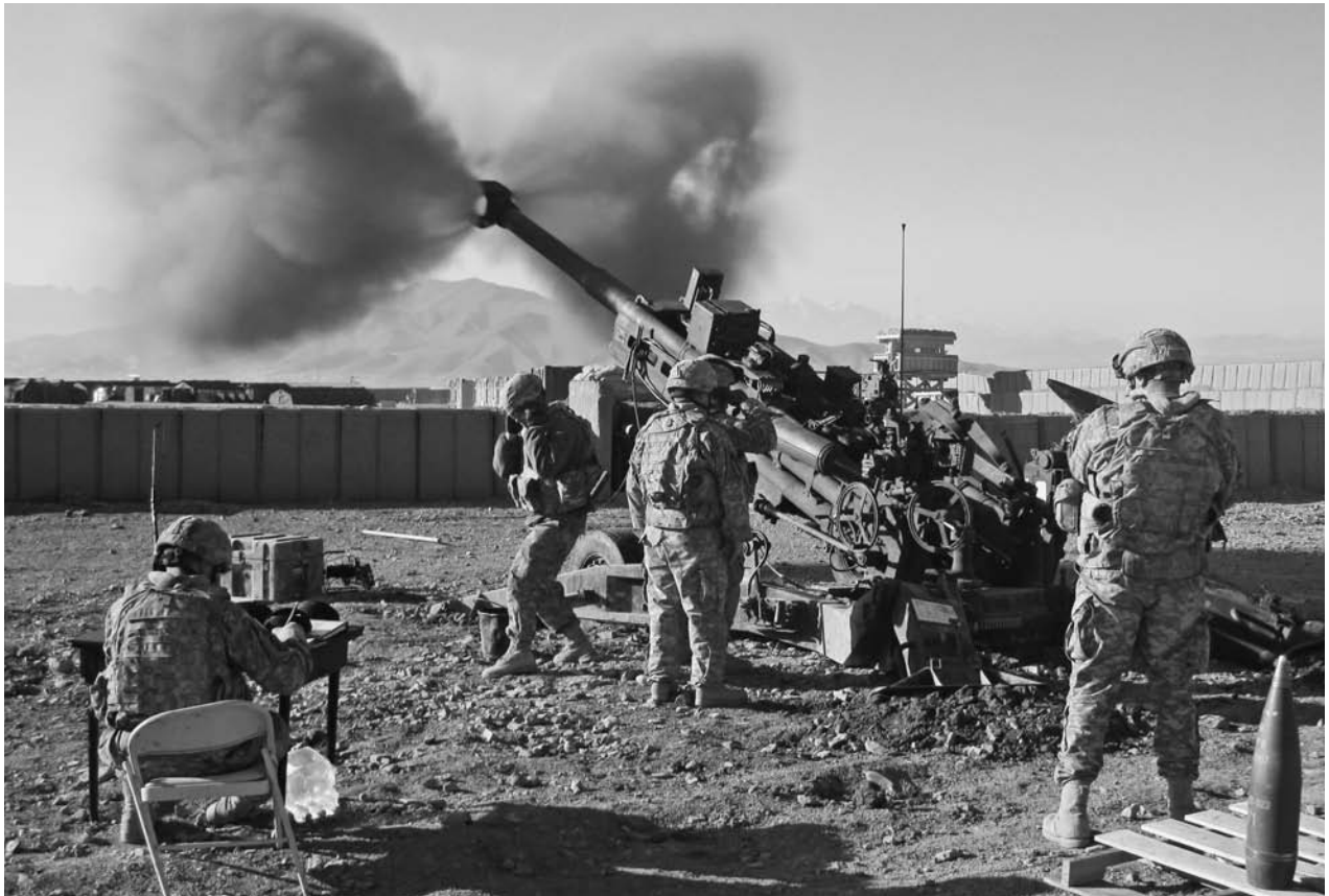
A U.S. M777 Light Towed Howitzer being fired in 2009 in Afghanistan. Howitzers have relatively short barrels and are used to shoot projectiles at high trajectories with a steep angle of descent.
