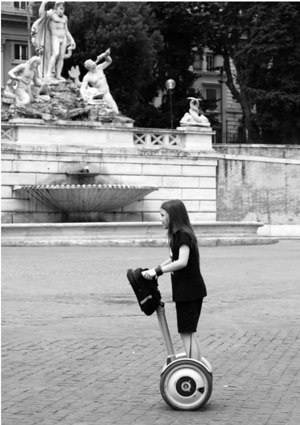
Riders lean forward to make the wheels move forward and lean back to stop the Segway.
