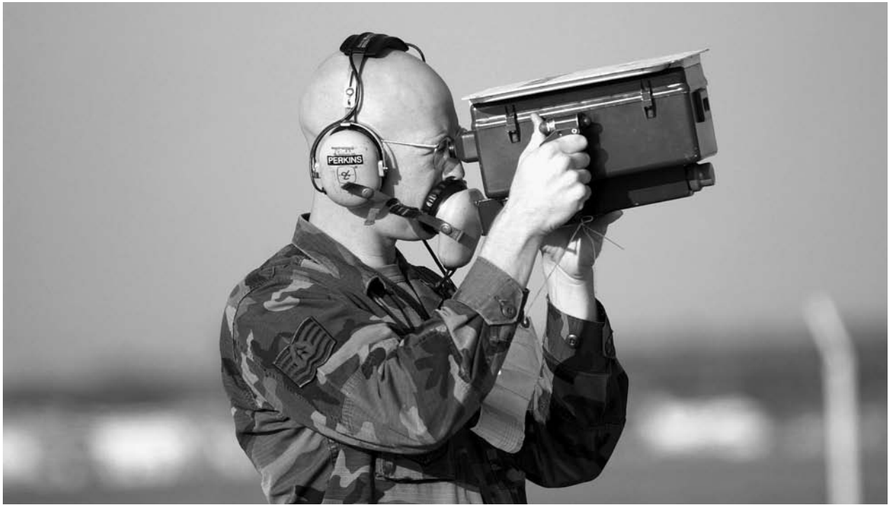
Scientists such as Luis Alvarez helped create the Identification Friend or Foe (IFF) radar camera, shown above, and improved antenna systems to identify friendly aircraft without using visual confirmation.
