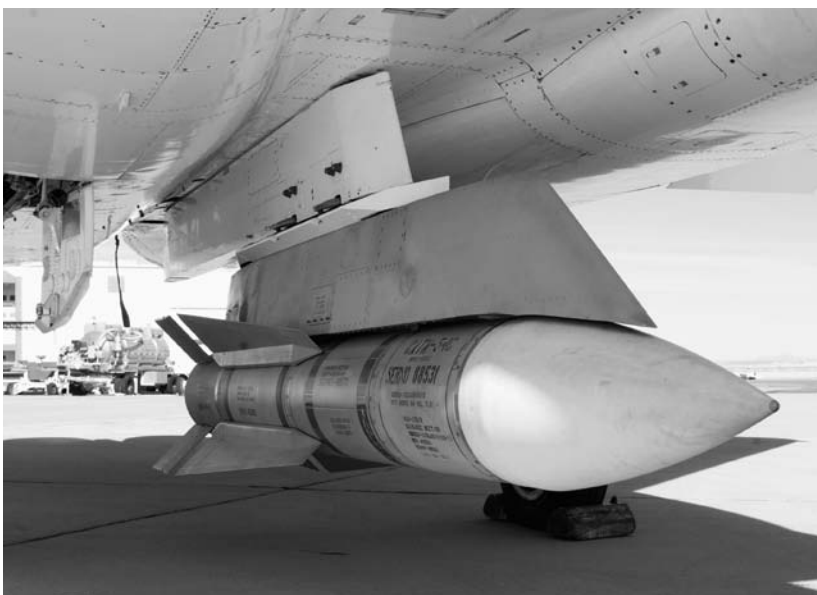
Surplus Phoenix missiles like this one mounted on NASA's F-15B research aircraft can be used to gather hypersonic flight test data.
