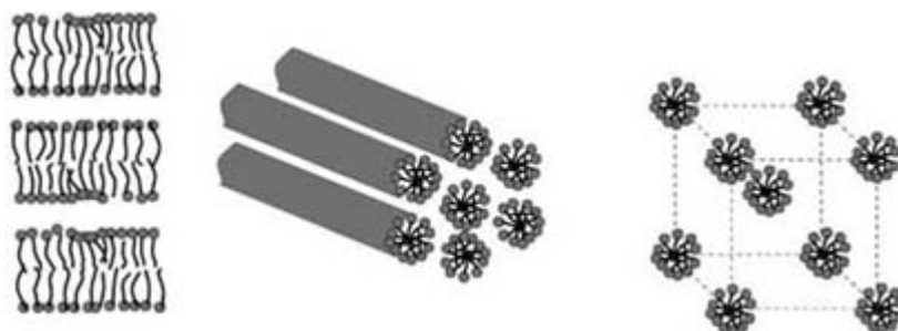
Figure B3.6.4. Illustration of three structured phases in a mixture of amphiphile and water. (a) Lamellar phase: the hydrophilic heads shield the hydrophobic tails from the water by forming a bilayer. The amphiphilic heads of different bilayers face each other and are separated by a thin water layer. (b) Hexagonal phase: the amphiphiles assemble into a rod-like structure where the tails are shielded in the interior from the water and the heads are on the outside. The rods arrange on a hexagonal lattice. (c) Cubic phase: amphiphilic micelles with a hydrophobic centre order on a BCC lattice.
