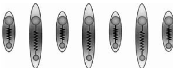
Figure B1.2.2. Schematic representation of the polarizability of a diatomic molecule as a function of vibrational coordinate. Because the polarizability changes during vibration, Raman scatter will occur in addition to Rayleigh scattering.
