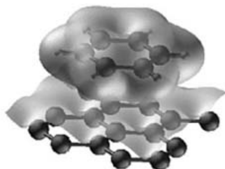
Figure B3.2.9. A benzene molecule on a graphite surface [90]. The geometry and the charge density (indicated by the surfaces of constant density) have been obtained using the PAW method. (Figure by Professor P E Blöchl.)
