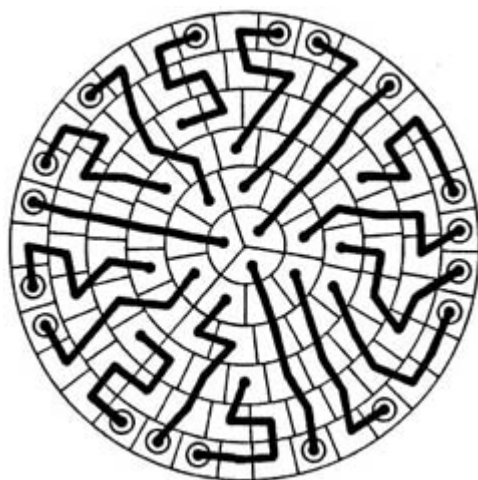
Figure C2.3.2. Two-dimensional radial lattice representation of micelle structure using the approach of Dill and Flory [6]. Each lattice site is considered to be equal in volume to the others. Reproduced by permission from [6].
