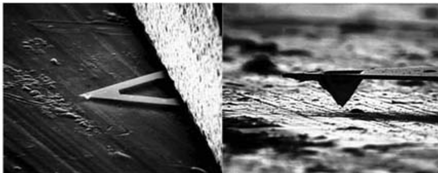
Figure B1.19.17. Commercially produced, microfabricated, V-shaped \text{Si}_3\text{N}_4 cantilever and tip for AFM (Taken from [215].)
