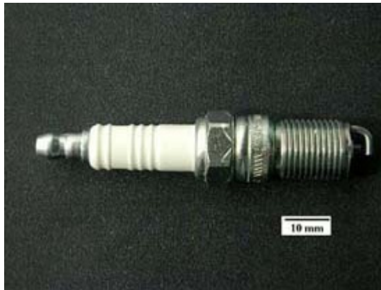
Figure C2.11.4. A commercial spark plug with its electrically insulating ceramic body comprised of alumina and glass (white portion).
