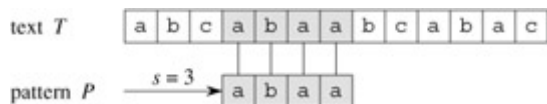
Figure 32.1: The string-matching problem. The goal is to find all occurrences of the pattern P = abaa in the text T = abcabaabcabac . The pattern occurs only once in the text, at shift s = 3 . The shift s = 3 is said to be a valid shift. Each character of the pattern is connected by a vertical line to the matching character in the text, and all matched characters are shown shaded.
