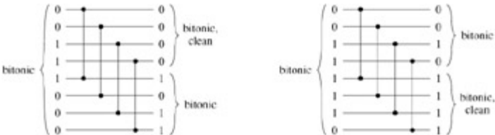
Figure 27.7: The comparison network HALF-CLEANER[8]. Two different sample zero-one input and output values are shown. The input is assumed to be bitonic. A half-cleaner ensures that every output element of the top half is at least as small as every output element of the bottom half. Moreover, both halves are bitonic, and at least one half is clean.
