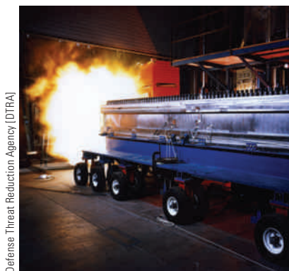
Figure 19.1 Rail guns launch projectiles at high speed using magnetic force. Larger versions could send payloads into space or be used as thrusters to move metal-rich asteroids from deep space to Earth orbit. In this photo a rail gun at Sandia National Laboratories in Albuquerque, New Mexico, fires a projectile at over three kilometers per second. (For more information on this, see Applying Physics 20.2 on pages 698–699.)
