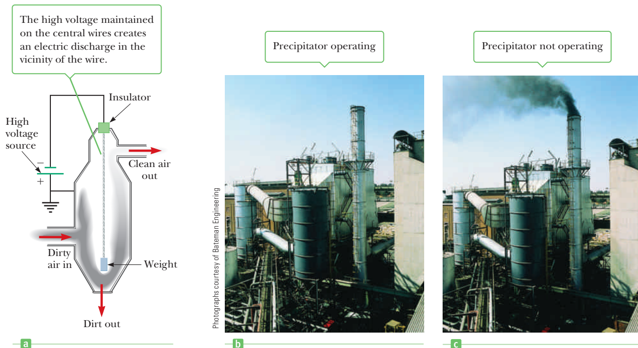
Figure 16.12 (a) A schematic diagram of an electrostatic precipitator. Compare the air pollution when the precipitator is (b) operating and (c) turned off.
