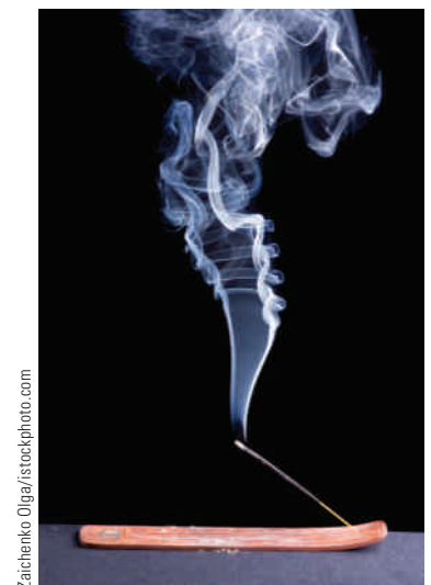
Figure 9.28 Hot gases made visible by smoke particles. The smoke first moves in laminar flow at the bottom and then in turbulent flow above.
