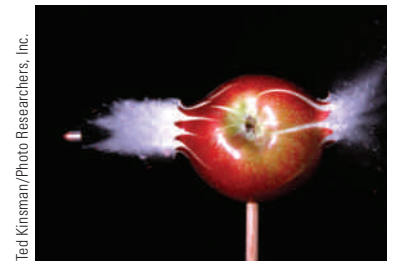
Figure 6.2 An apple being pierced by a 30-caliber bullet traveling at a supersonic speed of 900 m/s. This collision was photographed with a microflash stroboscope using an exposure time of 0.33 \mu\text{s} . Shortly after the photograph was taken, the apple disintegrated completely. Note that the points of entry and exit of the bullet are visually explosive.
