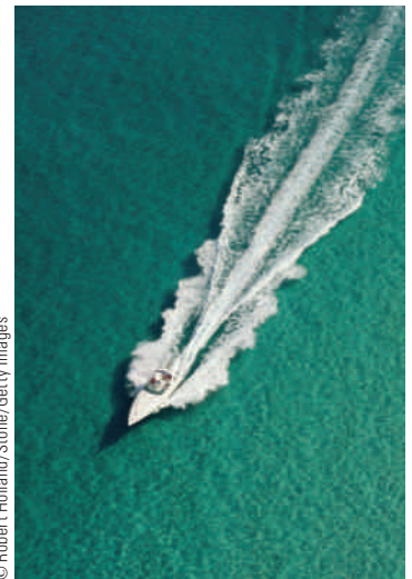
Figure 14.12 The V-shaped bow wave of a boat is formed because the boat travels at a speed greater than the speed of the water waves. A bow wave is analogous to a shock wave formed by an airplane traveling faster than sound.
