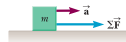
Figure 4.5 The second law of motion. For the block of mass m , the net force \Sigma \vec{F} acting on the block equals the mass m times the acceleration vector \vec{a} .
