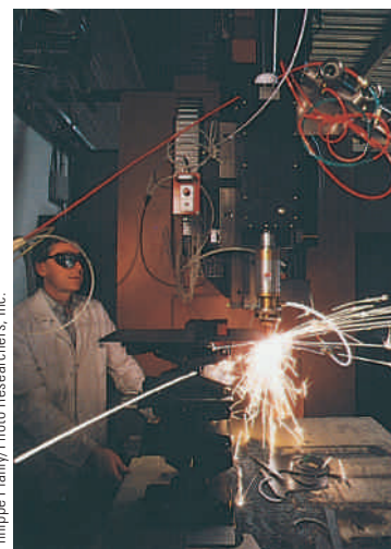
Scientist checking the performance of an experimental laser-cutting device mounted on a robot arm. The laser is being used to cut through a metal plate.
