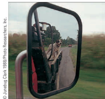
Figure 23.14 A convex side-view mirror on a vehicle produces an upright image that is smaller than the object. The smaller image means that the object is closer than its apparent distance as observed in the mirror.
