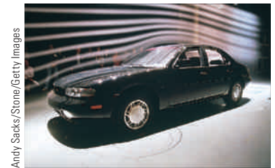
Figure 9.27 An illustration of streamline flow around an automobile in a test wind tunnel. The streamlines in the airflow are made visible by smoke particles.
