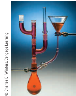
Figure 9.13 This photograph illustrates the fact that the pressure in a liquid is the same at all points lying at the same elevation. Note that the shape of the vessel does not affect the pressure.
