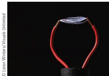
Figure 16.25 Dielectric breakdown in air. Sparks are produced when a large alternating voltage is applied across the wires by a high-voltage induction coil power supply.
