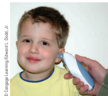
Figure 11.14 A radiation thermometer measures a patient's temperature by monitoring the intensity of infrared radiation leaving the ear.
