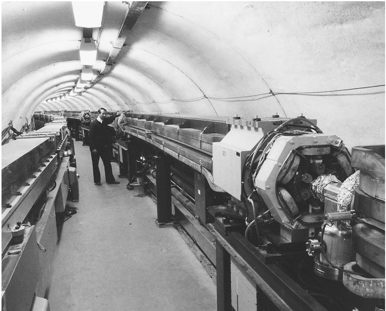
View inside the tunnel for CESR. The booster synchrotron is on the left, the storage ring on the right. CREDIT: COURTESY OF CORNELL UNIVERSITY.
