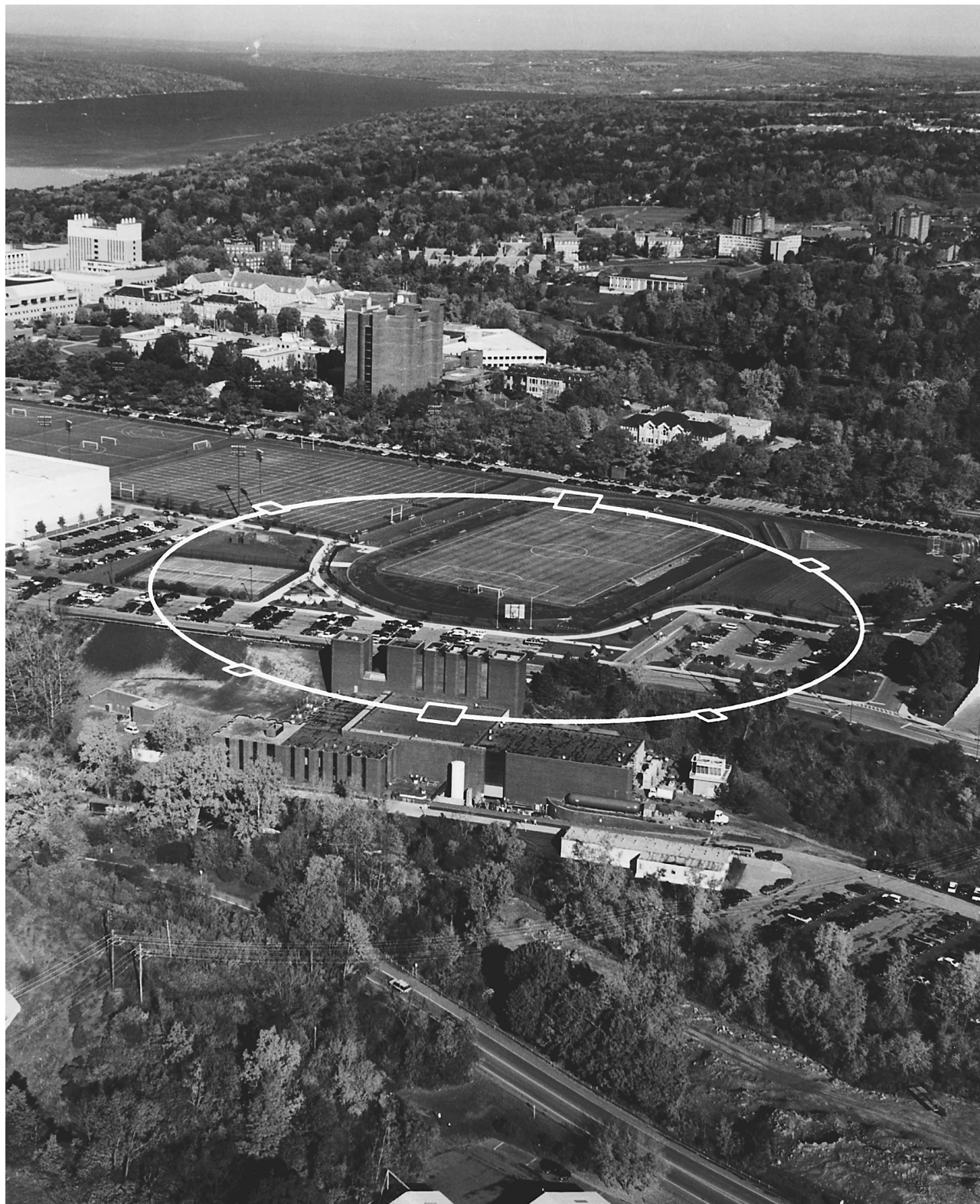
The superimposed oval shows the location of the Cornell Electron-Positron Storage Ring in a tunnel about 40 feet underground. The brick building at the near side of the oval is the Wilson Laboratory building, housing most of the laboratory facilities. CREDIT: COURTESY OF KARL BERKELMAN, CORNELL UNIVERSITY.
