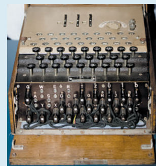
This is an Enigma machine used by the Germans in World War II to send coded messages.
