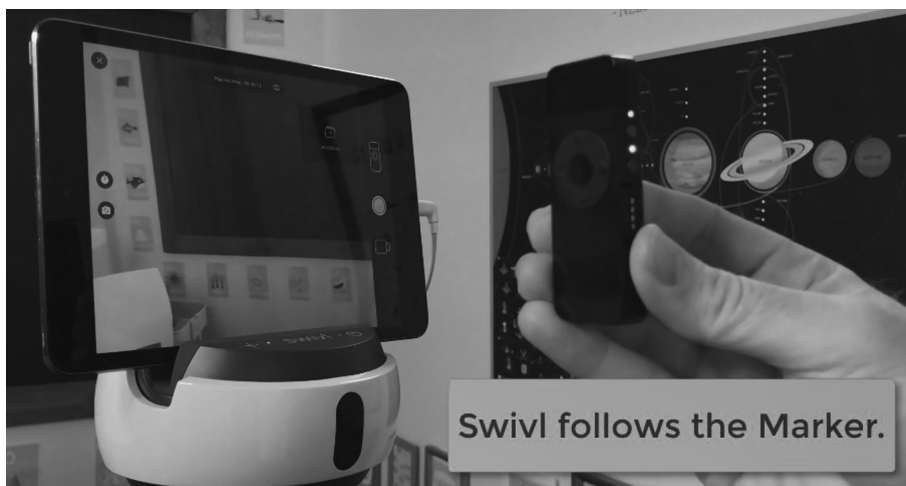
FIGURE 5.5 Swivl system for tracking lectures, image from their homepage ( www.swivl.com/how-to-use/ ). Note the instructor can see what is being recorded in the iPad screen, and the system follows the tracker in real-time.
