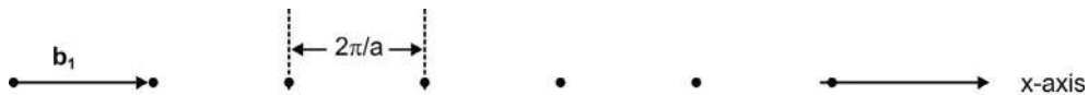
FIG. 2.3 Reciprocal lattice of a monatomic one-dimensional crystal having primitive lattice vector \mathbf{a}_1 such that |\mathbf{a}_1| = a . Here, dots represent the reciprocal lattice points and \mathbf{b}_1 = (2\pi/a)\hat{\mathbf{i}}_1 is the primitive reciprocal lattice vector.
