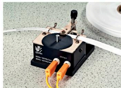
▲ Figure 7.1.3 This ticker timer is driven by a low voltage alternating supply at the mains frequency of 50 Hz. It produces 50 dots a second on the ticker tape.
