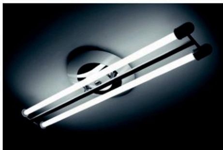
▲ Figure 7.9.8 A fluorescent lamp provides additional visible white light by converting invisible ultraviolet light into visible light. This is achieved by the phosphor coating on the inside of the glass tube.
