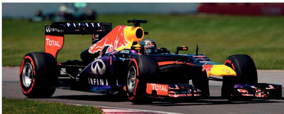
▲ Figure 4.4.5 The design of a racing car requires both a low centre of gravity and a wide wheel base for improved stability. This makes the car less likely to turn over.
