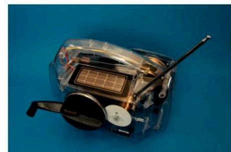
▲ Figure 7.9.11 Wind-up radio. This radio can be used anywhere in the world and requires neither a mains electricity nor a disposable battery supply. It can be used day and night. In the day time it uses solar cells to keep internal rechargeable batteries topped up and, when there is not enough light, energy can be supplied by winding up a spring that stores potential energy. This stored energy drives a small dynamo to charge up the batteries. In the photo you can see both the solar cells and the handle for winding up the spring.
