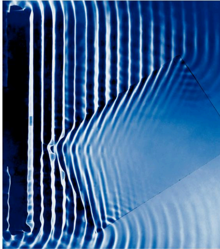
▲ Figure 11.3.6 Waves in a ripple tank being deflected by a straight barrier
