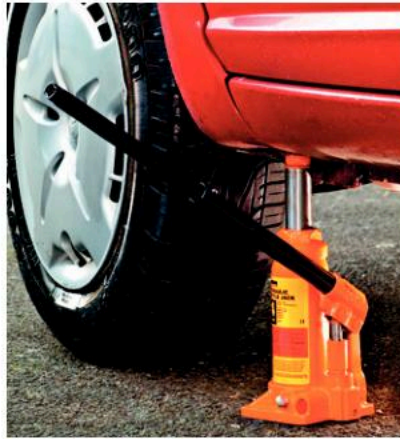
▲ Figure 6.2.5 This hydraulic jack is being used to lift a car in Kingston, Jamaica.
