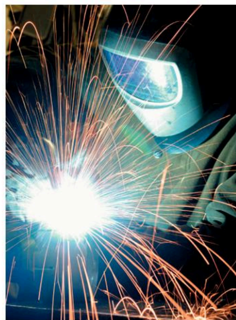
▲ Figure 12.4.3 The welder must wear a protective mask to provide protection from the ultraviolet light as well as physical protection against sparks. The high temperature of the welding flame produces a lot of ultraviolet light.
