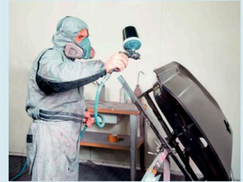
▲ Figure 13.4.5 Paint spraying equipment required to give an even coating of fine paint particles on a car body often uses electrostatic charges to control and direct the distribution of paint. Paint particles pick up charges from the spray gun nozzles and are attracted to the oppositely charged metal bodywork of the car. The paint particles, following the electric field lines, end up on the car body and not on the floor or wall behind.
