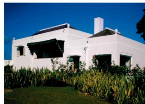
▲ Figure 15.3.4 This Caribbean home has white-painted walls and shades over the windows to keep the sunlight out. Both of these features help keep the house cool.
