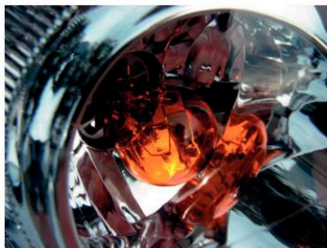
▲ Figure 9.5.6 The mirrors fitted behind a torch bulb or car head lamp are concave and are shaped to produce a near parallel beam of light. The best shape for this is a concave parabolic mirror.
