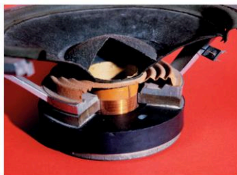
◀ Figure 18.1.6 This cut-away image of a moving-coil loudspeaker shows the following details. The permanent magnet is black and at the base of the construction. The moving copper wire voice coil is in the centre. The flexible, corrugated circular structure holds the moving coil in place. The upper, grey diaphragm is attached to the moving coil and produces sound waves in the air when the coil moves.
