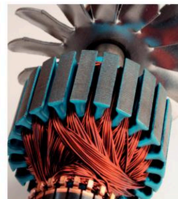
▲ Figure 18.2.2 Small electric motor with multiple coils of wire and multiple sets of brushes to connect to the power supply
