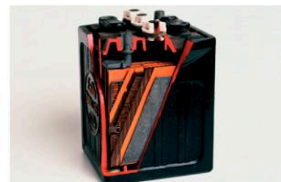
▲ Figure 14.9.2 A 12V car battery is made from six 2V cells. Each cell has lead plates in sulfuric acid.
