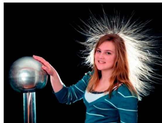
▲ Figure 13.2.3 The positive charge on the Van de Graaff generator flows onto the person. Because all their hairs have a positive charge, they all repel each other, so stand on end.
