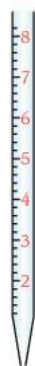
▲ Figure 2.1.11 Reading the scale on the pipette gives the volume of liquid contained in the pipette.
