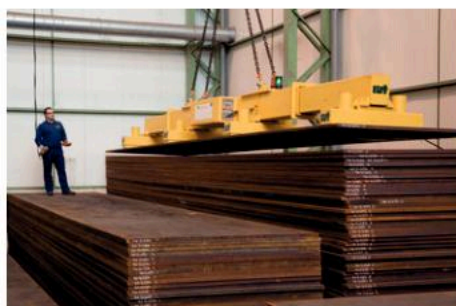
▲ Figure 17.4.2 An array of electromagnets provides an effective way of lifting single sheets of iron or steel. No hooks or chains are needed and the sheet metal can be released just by switching off the current.
