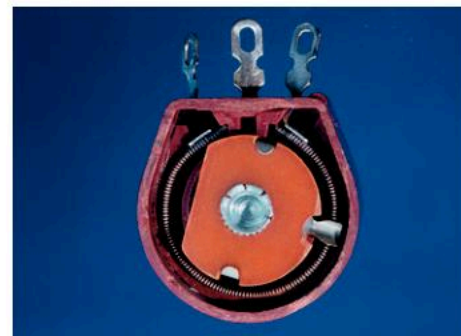
▲ Figure 14.6.4 The circular type of variable resistor shown here with its back removed has a curved, wire-wound track, which may be from about 2 cm to 4 cm in diameter. A knob is fitted to the other end of the central shaft. This device is often used as a volume control on hi-fi equipment and radios.
