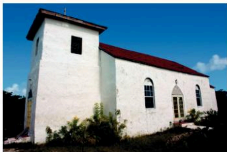
▲ Figure 8.4.11 Buildings in hot countries are often painted white because this helps them keep cool. White is best at reflecting visible and infrared radiation from the Sun.
