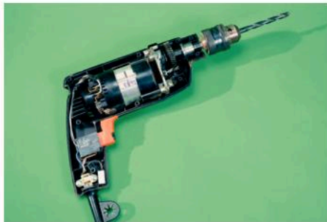
▲ Figure 18.2.4 The inside of an electric drill shows the brushes and commutator on the left of the rotor coils. The gears that reduce the speed of revolution of the drill are on the right.
