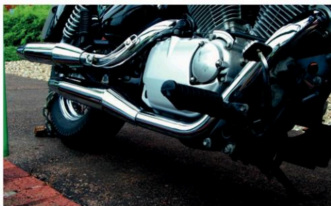
▲ Figure 8.4.10 It is important to cool a motor cycle engine efficiently. Attaching metal fins greatly increases the surface area and allows more cooling air to come into contact with the hot engine. A black surface radiates heat most efficiently.
