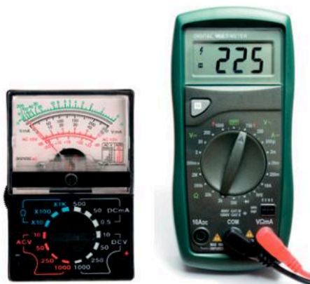
▲ Figure 14.5.4 An analogue or digital multimeter can be used to measure current or voltage.
