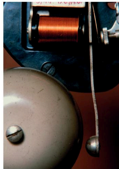
▲ Figure 17.4.8 The inside of a battery-powered doorbell
