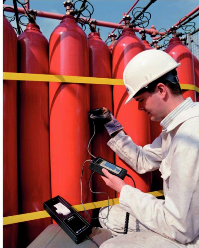
▲ Figure 11.5.8 Ultrasonic testing of the walls of high-pressure gas cylinders. An ultrasound narrow beam transducer is held against the wall of a cylinder and passes a high-frequency sound column wave through the metal walls. Echoes will be produced by any defects in the metal and the thickness of the wall can also be measured.
