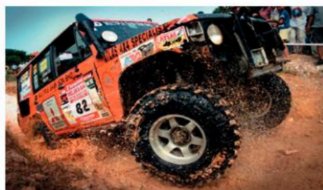
▲ Figure 7.5.14 As the wheels spin, mud flies out backwards at a tangent to the wheels. The soft mud fails to provide the forward force required for the wheels to grip and the vehicle to move forwards.
