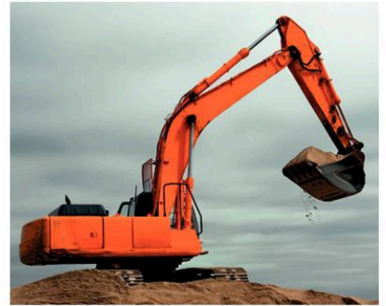
▲ Figure 6.2.6 The pistons that operate this hydraulic digger have a large cross-sectional area and so provide a large output force.
