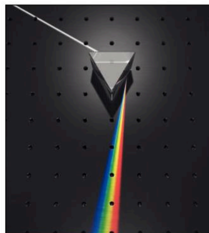
Figure 3.6.4 A prism can be used to disperse white light.
