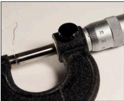
Figure 1.2.1 This micrometer is being used to measure the gauge of a wire.
