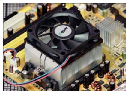
Figure 2.12.4 A heat sink mounted on a microprocessor
