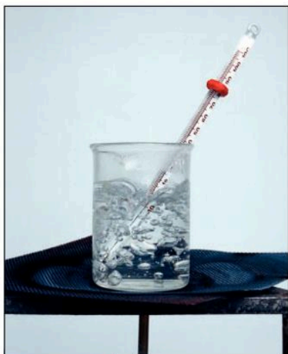
Figure 2.7.1 The temperature will stay at 100°C until all of the water has turned to gas.
