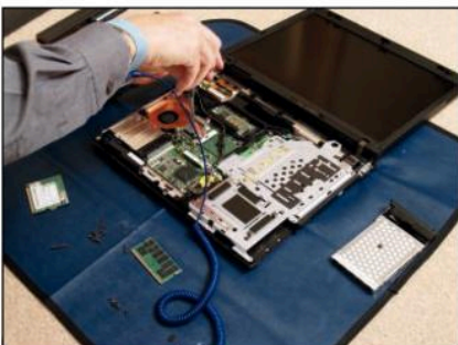
Figure 4.3.2 This electronic engineer is connected to the Earth through a wristband as he repairs a computer. Any static build-up in his body will discharge through the lead instead of damaging the delicate circuitry.
