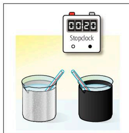
Figure 2.11.2 Investigating the effect of the colour of a surface on the rate of cooling
