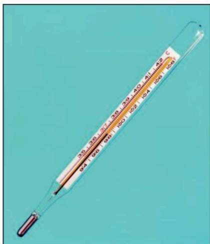
Figure 2.2.2 A clinical thermometer follows the same basic principles as a liquid-in-glass thermometer.
