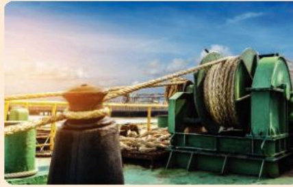
▲ This winch converts a rotational force into a linear force
