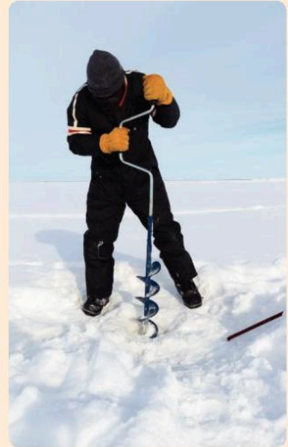
▲ An auger is used to drill through the ice
