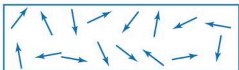
▲ In this magnetic substance, all the domains are misaligned. As a result, the individual magnetic fields each act against each other and so there is no overall magnetic field
