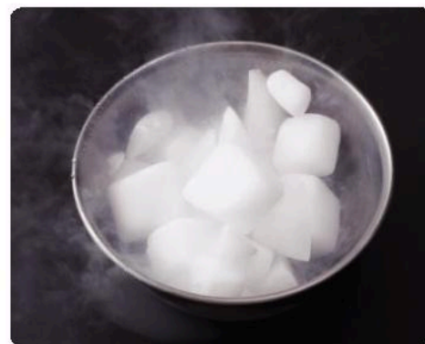
▲ This solid carbon dioxide sublimates from a solid straight into a gas
