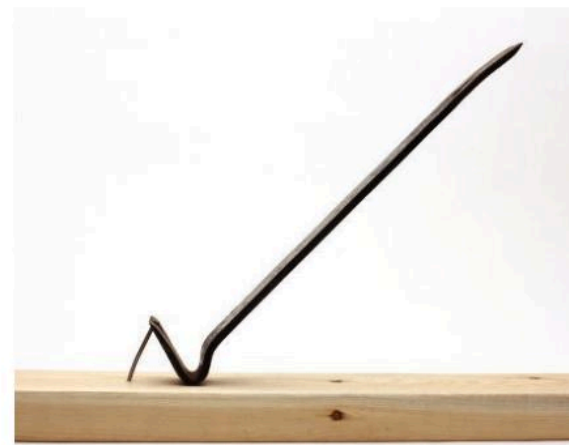
▲ A crowbar makes removing a nail much easier
