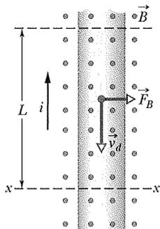
**Fig. 28-15** A close-up view of a section of the wire of Fig. 28-14b. The current direction is upward, which means that electrons drift downward. A magnetic field that emerges from the plane of the page causes the electrons and the wire to be deflected to the right.
