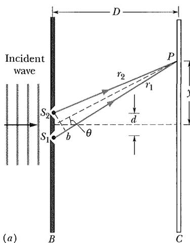
**Fig. 35-10** (a) Waves from slits  $S_1$  and  $S_2$  (which extend into and out of the page) combine at  $P$ , an arbitrary point on screen  $C$  at distance  $y$  from the central axis. The angle  $\theta$  serves as a convenient locator for  $P$ . (b) For  $D \gg d$ , we can approximate rays  $r_1$  and  $r_2$  as being parallel, at angle  $\theta$  to the central axis.
