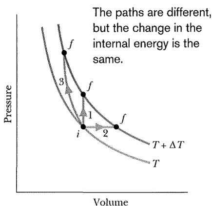
**Fig. 19-10** Three paths representing three different processes that take an ideal gas from an initial state  $i$  at temperature  $T$  to some final state  $f$  at temperature  $T + \Delta T$ . The change  $\Delta E_{\text{int}}$  in the internal energy of the gas is the same for these three processes and for any others that result in the same change of temperature.
