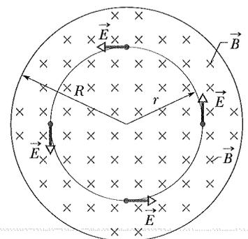
**Fig. 32-6** A uniform magnetic field  $\vec{B}$  in a circular region. The field, directed into the page, is increasing in magnitude. The electric field  $\vec{E}$  induced by the changing magnetic field is shown at four points on a circle concentric with the circular region. Compare this situation with that of Fig. 32-5b.
