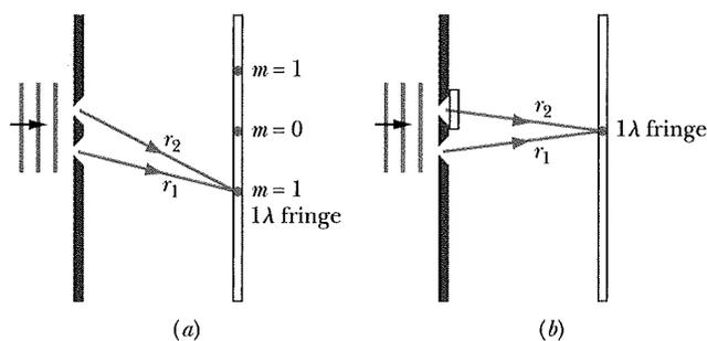
**Fig. 35-11** (a) Arrangement for two-slit interference (not to scale). The locations of three bright fringes (or maxima) are indicated. (b) A strip of plastic covers the top slit. We want the  $1\lambda$  fringe to be at the center of the pattern.
