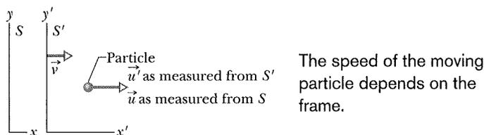
**Fig. 37-11** Reference frame  $S'$  moves with velocity  $\vec{v}$  relative to frame  $S$ . A particle has velocity  $\vec{u}'$  relative to reference frame  $S'$  and velocity  $\vec{u}$  relative to reference frame  $S$ .
