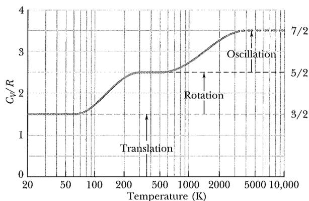
**Fig. 19-14**  $C_V/R$  versus temperature for (diatomic) hydrogen gas. Because rotational and oscillatory motions begin at certain energies, only translation is possible at very low temperatures. As the temperature increases, rotational motion can begin. At still higher temperatures, oscillatory motion can begin.
