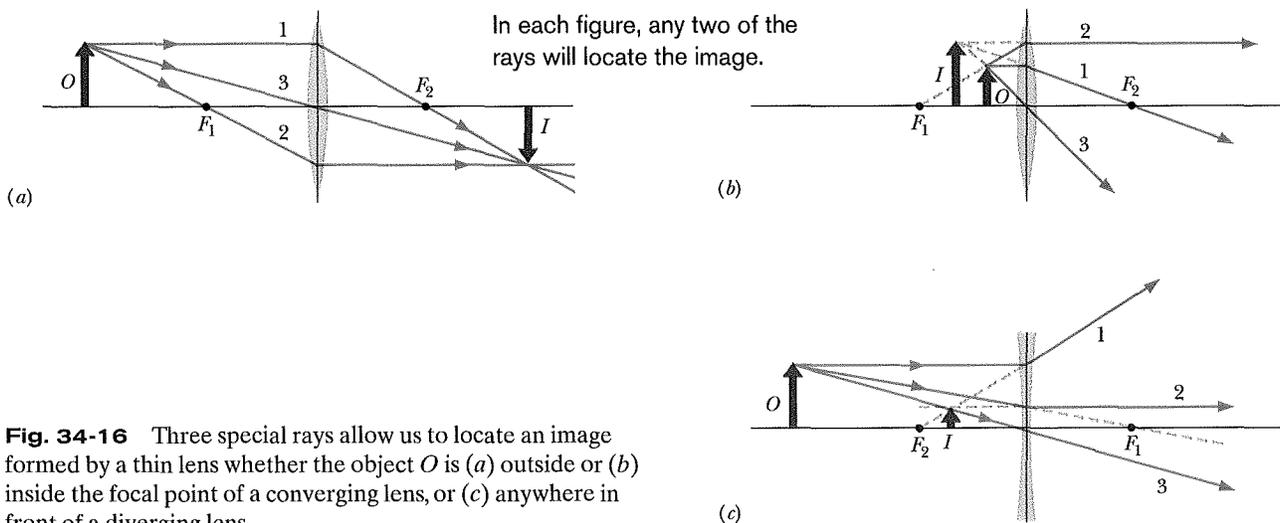
**Fig. 34-16** Three special rays allow us to locate an image formed by a thin lens whether the object  $O$  is (a) outside or (b) inside the focal point of a converging lens, or (c) anywhere in front of a diverging lens.
