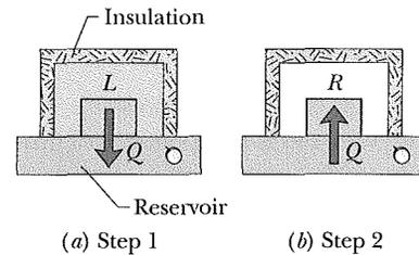
**Fig. 20-6** The blocks of Fig. 20-5 can proceed from their initial state to their final state in a reversible way if we use a reservoir with a controllable temperature (a) to extract heat reversibly from block  $L$  and (b) to add heat reversibly to block  $R$ .
