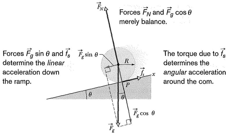
**Fig. 11-8** A round uniform body of radius  $R$  rolls down a ramp. The forces that act on it are the gravitational force  $\vec{F}_g$ , a normal force  $\vec{F}_N$ , and a frictional force  $\vec{f}_s$  pointing up the ramp. (For clarity, vector  $\vec{F}_N$  has been shifted in the direction it points until its tail is at the center of the body.)
