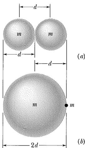
**Fig. 19-6** (a) A collision occurs when the centers of two molecules come within a distance  $d$  of each other,  $d$  being the molecular diameter. (b) An equivalent but more convenient representation is to think of the moving molecule as having a *radius*  $d$  and all other molecules as being points. The condition for a collision is unchanged.
