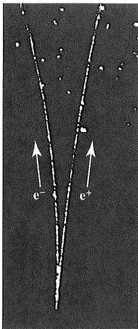
**Fig. 21-11** A photograph of trails of bubbles left in a bubble chamber by an electron and a positron. The pair of particles was produced by a gamma ray that entered the chamber directly from the bottom. Being electrically neutral, the gamma ray did not generate a telltale trail of bubbles along its path, as the electron and positron did. (Courtesy Lawrence Berkeley Laboratory)
