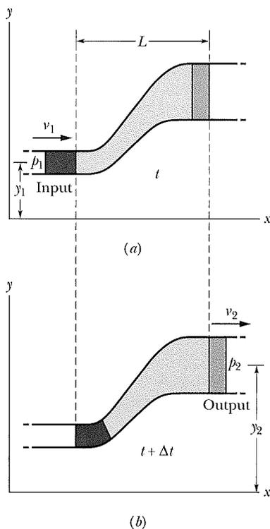
**Fig. 14-19** Fluid flows at a steady rate through a length  $L$  of a tube, from the input end at the left to the output end at the right. From time  $t$  in (a) to time  $t + \Delta t$  in (b), the amount of fluid shown in purple enters the input end and the equal amount shown in green emerges from the output end.
