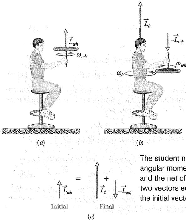
**Fig. 11-20** (a) A student holds a bicycle wheel rotating around a vertical axis. (b) The student inverts the wheel, setting himself into rotation. (c) The net angular momentum of the system must remain the same in spite of the inversion.
