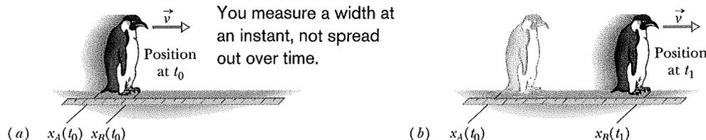
Let  $L_0$  be the length of a rod that you measure when the rod is stationary (meaning you and it are in the same reference frame, the rod's rest frame). If, instead, there is relative motion at speed  $v$  between you and the rod *along the length of the rod*, then with simultaneous measurements you obtain a length  $L$  given by
