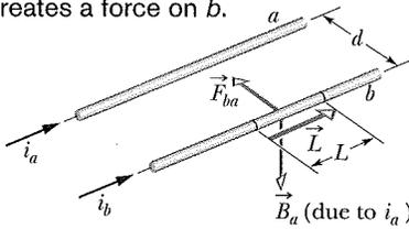
**Fig. 29-9** Two parallel wires carrying currents in the same direction attract each other.  $\vec{B}_a$  is the magnetic field at wire  $b$  produced by the current in wire  $a$ .  $\vec{F}_{ba}$  is the resulting force acting on wire  $b$  because it carries current in  $\vec{B}_a$ .
