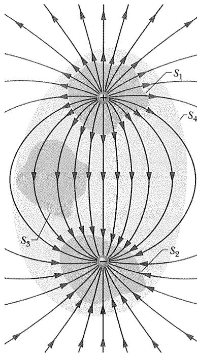
**Fig. 23-6** Two point charges, equal in magnitude but opposite in sign, and the field lines that represent their net electric field. Four Gaussian surfaces are shown in cross section. Surface  $S_1$  encloses the positive charge. Surface  $S_2$  encloses the negative charge. Surface  $S_3$  encloses no charge. Surface  $S_4$  encloses both charges and thus no net charge.
