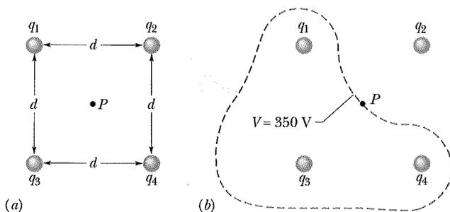
**Fig. 24-8** (a) Four point charges are held fixed at the corners of a square. (b) The closed curve is a cross section, in the plane of the figure, of the equipotential surface that contains point  $P$ . (The curve is drawn only roughly.)
