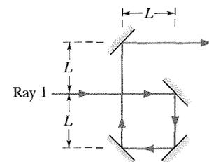
••12 In Fig. 35-34, two light rays go through different paths by reflecting from the various flat surfaces shown. The light waves have a wavelength of 420.0 nm and are initially in phase. What are the (a) smallest and (b) second smallest
