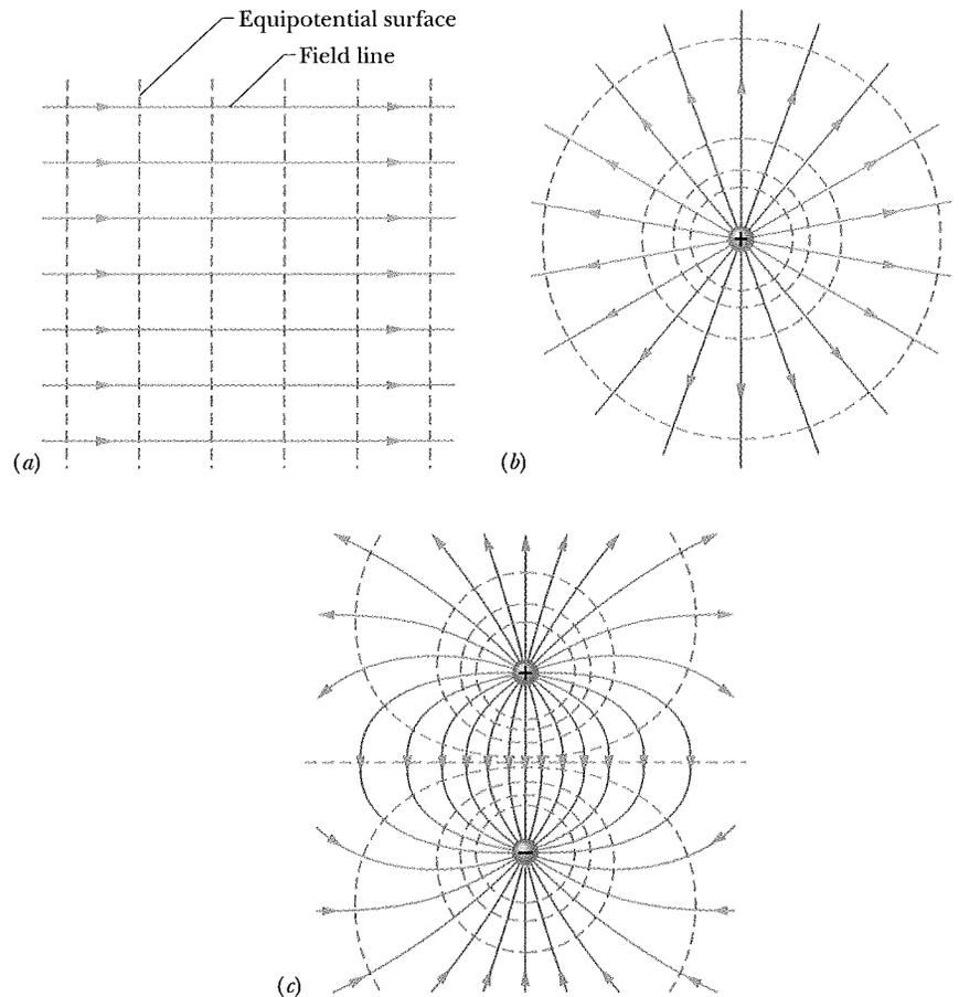
**Fig. 24-3** Electric field lines (purple) and cross sections of equipotential surfaces (gold) for (a) a uniform electric field, (b) the field due to a point charge, and (c) the field due to an electric dipole.
