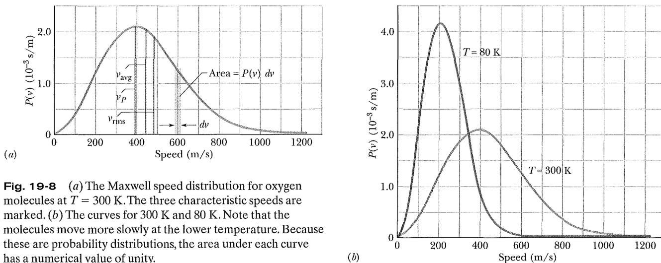
**Fig. 19-8** (a) The Maxwell speed distribution for oxygen molecules at  $T = 300 \text{ K}$ . The three characteristic speeds are marked. (b) The curves for  $300 \text{ K}$  and  $80 \text{ K}$ . Note that the molecules move more slowly at the lower temperature. Because these are probability distributions, the area under each curve has a numerical value of unity.
