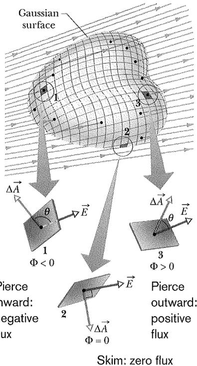
**Fig. 23-3** A Gaussian surface of arbitrary shape immersed in an electric field. The surface is divided into small squares of area  $\Delta A$ . The electric field vectors  $\vec{E}$  and the area vectors  $\Delta\vec{A}$  for three representative squares, marked 1, 2, and 3, are shown.
