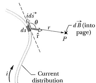
**Fig. 29-1** A current-length element  $i d\vec{s}$  produces a differential magnetic field  $d\vec{B}$  at point  $P$ . The green  $\times$  (the tail of an arrow) at the dot for point  $P$  indicates that  $d\vec{B}$  is directed *into* the page there.
