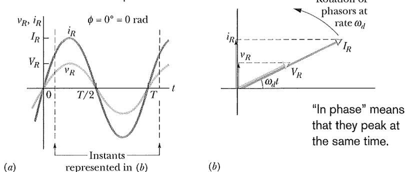
**Fig. 31-9** (a) The current  $i_R$  and the potential difference  $v_R$  across the resistor are plotted on the same graph, both versus time  $t$ . They are in phase and complete one cycle in one period  $T$ . (b) A phasor diagram shows the same thing as (a).
