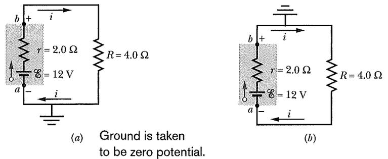
**Fig. 27-7** (a) Point  $a$  is directly connected to ground. (b) Point  $b$  is directly connected to ground.
