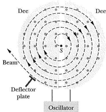
**Fig. 28-13** The elements of a cyclotron, showing the particle source  $S$  and the dees. A uniform magnetic field is directed up from the plane of the page. Circulating protons spiral outward within the hollow dees, gaining energy every time they cross the gap between the dees.
