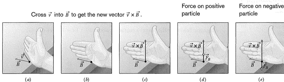
**Fig. 28-2** (a)–(c) The right-hand rule (in which  $\vec{v}$  is swept into  $\vec{B}$  through the smaller angle  $\phi$  between them) gives the direction of  $\vec{v} \times \vec{B}$  as the direction of the thumb. (d) If  $q$  is positive, then the direction of  $\vec{F}_B = q\vec{v} \times \vec{B}$  is in the direction of  $\vec{v} \times \vec{B}$ . (e) If  $q$  is negative, then the direction of  $\vec{F}_B$  is opposite that of  $\vec{v} \times \vec{B}$ .
