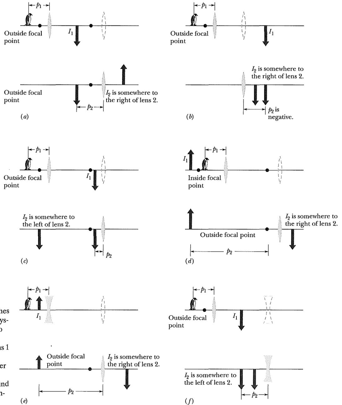
**Fig. 34-17** Several sketches (not to scale) of a two-lens system in which an object sits to the left of lens 1. In step 1 of the solution, we consider lens 1 and ignore lens 2 (shown in dashes). In step 2, we consider lens 2 and ignore lens 1 (no longer shown). We want to find the final image, that is, the image produced by lens 2.
