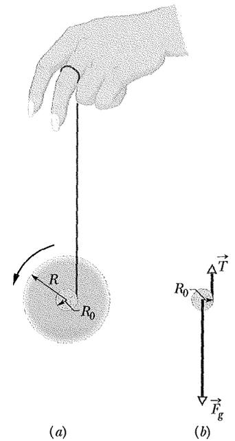
**Fig. 11-9** (a) A yo-yo, shown in cross section. The string, of assumed negligible thickness, is wound around an axle of radius  $R_0$ . (b) A free-body diagram for the falling yo-yo. Only the axle is shown.
