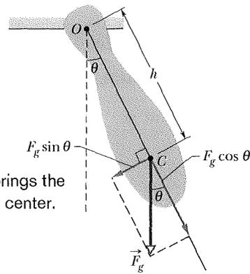
**Fig. 15-10** A physical pendulum. The restoring torque is  $hF_g \sin \theta$ . When  $\theta = 0$ , center of mass  $C$  hangs directly below pivot point  $O$ .
