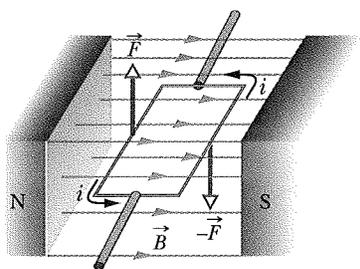
**Fig. 28-18** The elements of an electric motor. A rectangular loop of wire, carrying a current and free to rotate about a fixed axis, is placed in a magnetic field. Magnetic forces on the wire produce a torque that rotates it. A commutator (not shown) reverses the direction of the current every half-revolution so that the torque always acts in the same direction.
