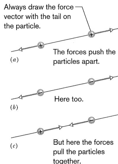
**Fig. 21-6** Two charged particles repel each other if they have the same sign of charge, either (a) both positive or (b) both negative. (c) They attract each other if they have opposite signs of charge.
