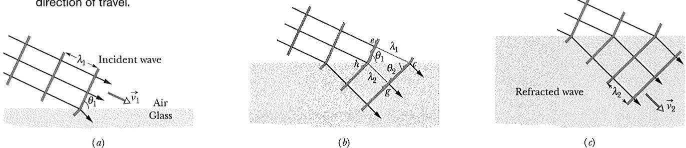
**Fig. 35-3** The refraction of a plane wave at an air–glass interface, as portrayed by Huygens' principle. The wavelength in glass is smaller than that in air. For simplicity, the reflected wave is not shown. Parts (a) through (c) represent three successive stages of the refraction.
