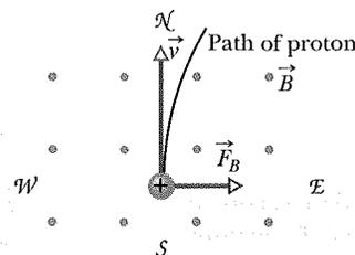
**Fig. 28-6** An overhead view of a proton moving from south to north with velocity  $\vec{v}$  in a chamber. A magnetic field is directed vertically upward in the chamber, as represented by the array of dots (which resemble the tips of arrows). The proton is deflected toward the east.
