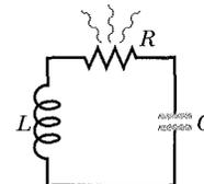
**Fig. 31-5** A series *RLC* circuit. As the charge contained in the circuit oscillates back and forth through the resistance, electromagnetic energy is dissipated as thermal energy, damping (decreasing the amplitude of) the oscillations.
