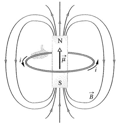
**Fig. 29-21** A current loop produces a magnetic field like that of a bar magnet and thus has associated north and south poles. The magnetic dipole moment  $\vec{\mu}$  of the loop, its direction given by a curled–straight right-hand rule, points from the south pole to the north pole, in the direction of the field  $\vec{B}$  within the loop.
