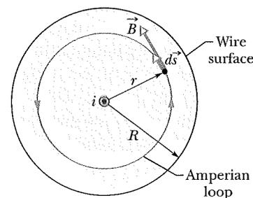
**Fig. 29-14** Using Ampere's law to find the magnetic field that a current  $i$  produces inside a long straight wire of circular cross section. The current is uniformly distributed over the cross section of the wire and emerges from the page. An Amperian loop is drawn inside the wire.
