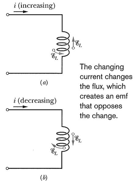
**Fig. 30-14** (a) The current  $i$  is increasing, and the self-induced emf  $\mathcal{E}_L$  appears along the coil in a direction such that it opposes the increase. The arrow representing  $\mathcal{E}_L$  can be drawn along a turn of the coil or alongside the coil. Both are shown. (b) The current  $i$  is decreasing, and the self-induced emf appears in a direction such that it opposes the decrease.
