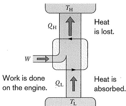
**Fig. 20-14** The elements of a refrigerator. The two black arrowheads on the central loop suggest the working substance operating in a cycle, as if on a  $p$ - $V$  plot. Energy is transferred as heat  $Q_L$  to the working substance from the low-temperature reservoir. Energy is transferred as heat  $Q_H$  to the high-temperature reservoir from the working substance. Work  $W$  is done on the refrigerator (on the working substance) by something in the environment.
