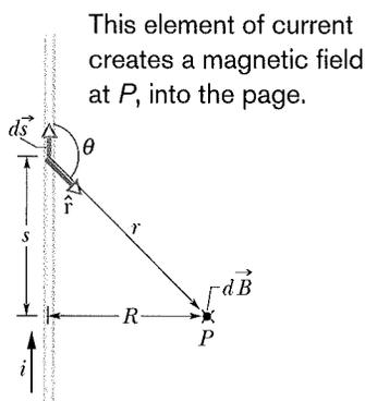
**Fig. 29-5** Calculating the magnetic field produced by a current  $i$  in a long straight wire. The field  $d\vec{B}$  at  $P$  associated with the current-length element  $i d\vec{s}$  is directed into the page, as shown.
