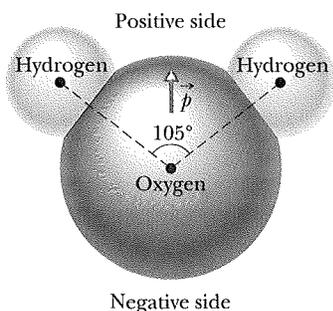
**Fig. 22-18** A molecule of  $\text{H}_2\text{O}$ , showing the three nuclei (represented by dots) and the regions in which the electrons can be located. The electric dipole moment  $\vec{p}$  points from the (negative) oxygen side to the (positive) hydrogen side of the molecule.
