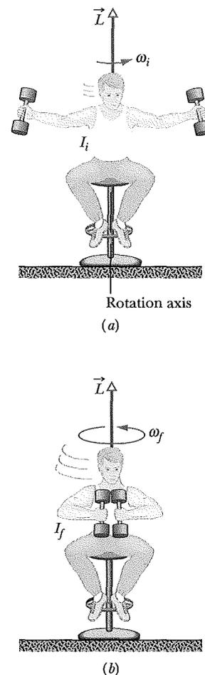
**Fig. 11-16** (a) The student has a relatively large rotational inertia about the rotation axis and a relatively small angular speed. (b) By decreasing his rotational inertia, the student automatically increases his angular speed. The angular momentum  $\vec{L}$  of the rotating system remains unchanged.
