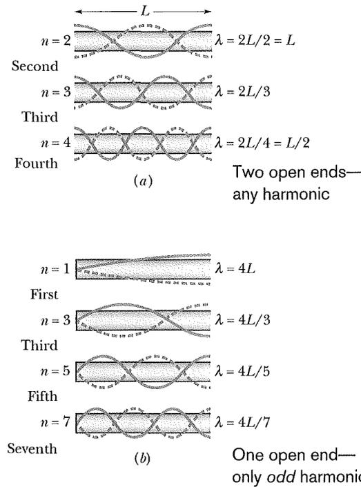
**Fig. 17-14** Standing wave patterns for string waves superimposed on pipes to represent standing sound wave patterns in the pipes. (a) With both ends of the pipe open, any harmonic can be set up in the pipe. (b) With only one end open, only odd harmonics can be set up.
