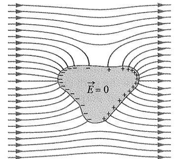
**Fig. 24-20** An uncharged conductor is suspended in an external electric field. The free electrons in the conductor distribute themselves on the surface as shown, so as to reduce the net electric field inside the conductor to zero and make the net field at the surface perpendicular to the surface.
