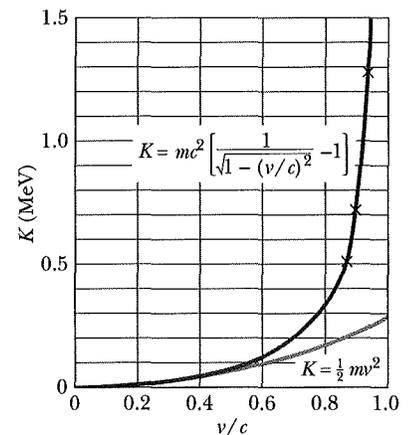
**Fig. 37-13** The relativistic (Eq. 37-52) and classical (Eq. 37-51) equations for the kinetic energy of an electron, plotted as a function of  $v/c$ , where  $v$  is the speed of the electron and  $c$  is the speed of light. Note that the two curves blend together at low speeds and diverge widely at high speeds. Experimental data (at the  $\times$  marks) show that at high speeds the relativistic curve agrees with experiment but the classical curve does not.
