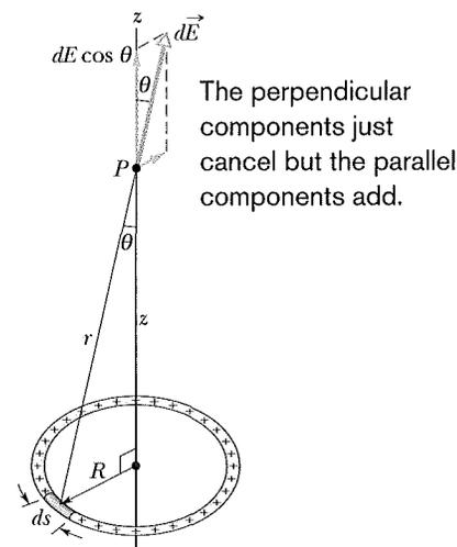
**Fig. 22-10** A ring of uniform positive charge. A differential element of charge occupies a length  $ds$  (greatly exaggerated for clarity). This element sets up an electric field  $d\vec{E}$  at point  $P$ . The component of  $d\vec{E}$  along the central axis of the ring is  $dE \cos \theta$ .
