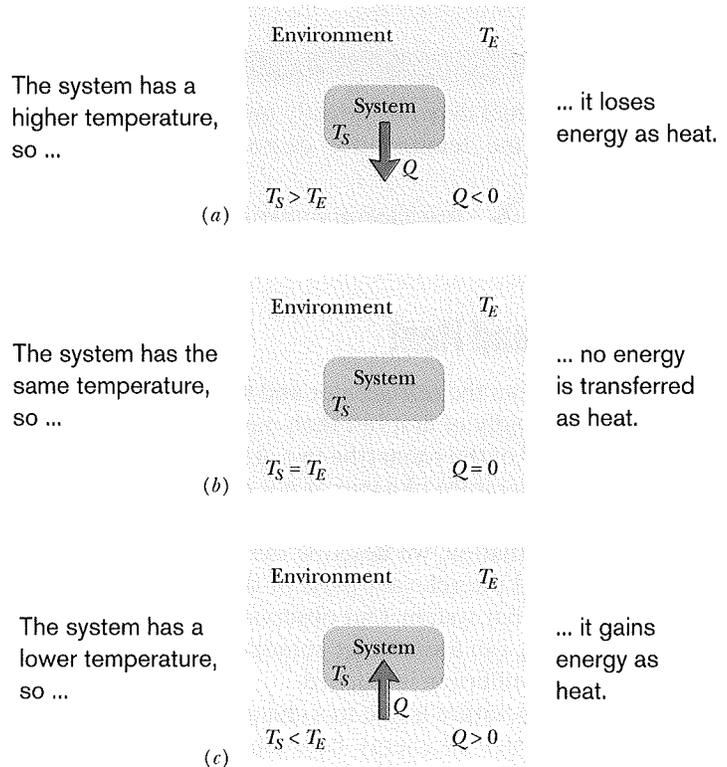
**Fig. 18-12** If the temperature of a system exceeds that of its environment as in (a), heat  $Q$  is lost by the system to the environment until thermal equilibrium (b) is established. (c) If the temperature of the system is below that of the environment, heat is absorbed by the system until thermal equilibrium is established.
