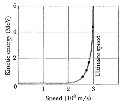
**Fig. 37-2** The dots show measured values of the kinetic energy of an electron plotted against its measured speed. No matter how much energy is given to an electron (or to any other particle having mass), its speed can never equal or exceed the ultimate limiting speed  $c$ . (The plotted curve through the dots shows the predictions of Einstein's special theory of relativity.)
