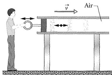
**Fig. 16-2** A sound wave is set up in an air-filled pipe by moving a piston back and forth. Because the oscillations of an element of the air (represented by a dot) are parallel to the direction in which the wave travels, the wave is a *longitudinal wave*.
