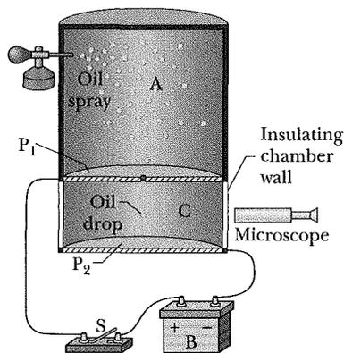
**Fig. 22-14** The Millikan oil-drop apparatus for measuring the elementary charge  $e$ . When a charged oil drop drifted into chamber C through the hole in plate  $P_1$ , its motion could be controlled by closing and opening switch S and thereby setting up or eliminating an electric field in chamber C. The microscope was used to view the drop, to permit timing of its motion.
