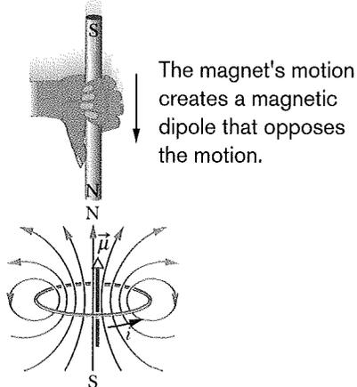
**Fig. 30-4** Lenz's law at work. As the magnet is moved toward the loop, a current is induced in the loop. The current produces its own magnetic field, with magnetic dipole moment  $\vec{\mu}$  oriented so as to oppose the motion of the magnet. Thus, the induced current must be counterclockwise as shown.
