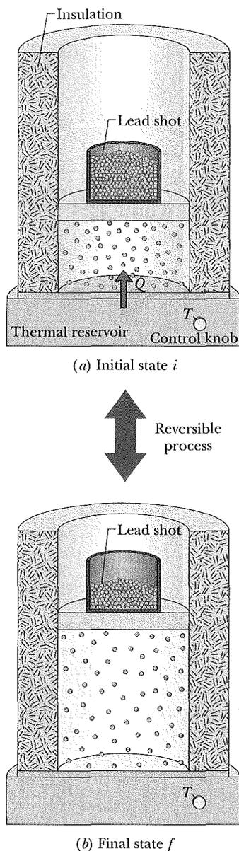
**Fig. 20-3** The isothermal expansion of an ideal gas, done in a reversible way. The gas has the same initial state  $i$  and same final state  $f$  as in the irreversible process of Figs. 20-1 and 20-2.
