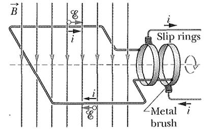
**Fig. 31-6** The basic mechanism of an alternating-current generator is a conducting loop rotated in an external magnetic field. In practice, the alternating emf induced in a coil of many turns of wire is made accessible by means of slip rings attached to the rotating loop. Each ring is connected to one end of the loop wire and is electrically connected to the rest of the generator circuit by a conducting brush against which the ring slips as the loop (and it) rotates.
