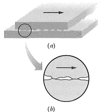
**Fig. 6-2** The mechanism of sliding friction. (a) The upper surface is sliding to the right over the lower surface in this enlarged view. (b) A detail, showing two spots where cold-welding has occurred. Force is required to break the welds and maintain the motion.
