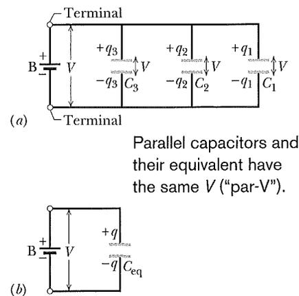
**Fig. 25-8** (a) Three capacitors connected in parallel to battery B. The battery maintains potential difference  $V$  across its terminals and thus across *each* capacitor. (b) The equivalent capacitor, with capacitance  $C_{\text{eq}}$ , replaces the parallel combination.
