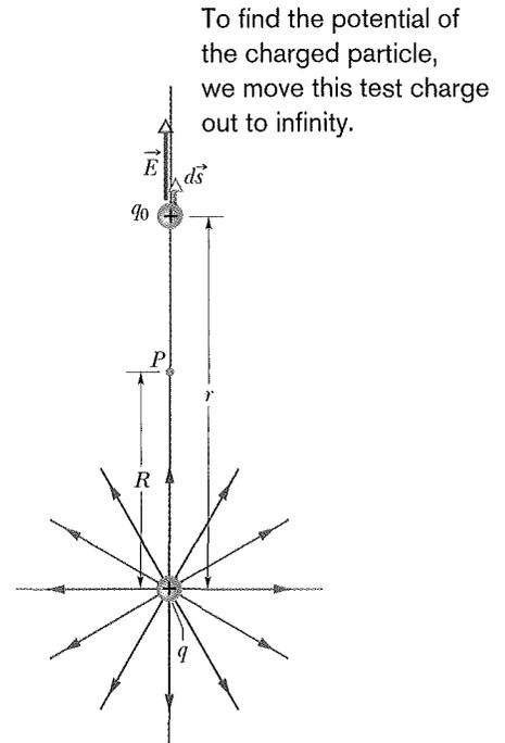
**Fig. 24-6** The positive point charge  $q$  produces an electric field  $\vec{E}$  and an electric potential  $V$  at point  $P$ . We find the potential by moving a test charge  $q_0$  from  $P$  to infinity. The test charge is shown at distance  $r$  from the point charge, during differential displacement  $d\vec{s}$ .
