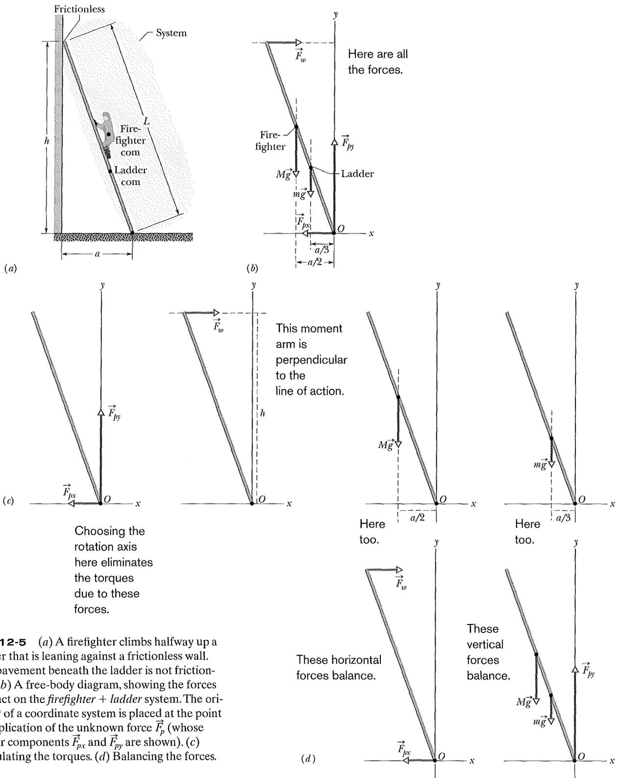
**Fig. 12-5** (a) A firefighter climbs halfway up a ladder that is leaning against a frictionless wall. The pavement beneath the ladder is not frictionless. (b) A free-body diagram, showing the forces that act on the *firefighter + ladder* system. The origin  $O$  of a coordinate system is placed at the point of application of the unknown force  $\vec{F}_p$  (whose vector components  $\vec{F}_{px}$  and  $\vec{F}_{py}$  are shown). (c) Calculating the torques. (d) Balancing the forces.
