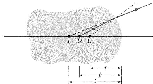
**Fig. 34-13** A piece of amber with a mosquito from the Jurassic period, with the head buried at point  $O$ . The spherical refracting surface at the right end, with center of curvature  $C$ , provides an image  $I$  to an observer intercepting rays from the object at  $O$ .
