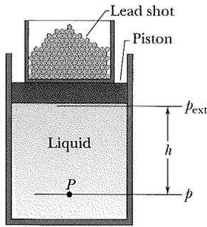
**Fig. 14-7** Lead shot (small balls of lead) loaded onto the piston create a pressure  $p_{\text{ext}}$  at the top of the enclosed (incompressible) liquid. If  $p_{\text{ext}}$  is increased, by adding more lead shot, the pressure increases by the same amount at all points within the liquid.
