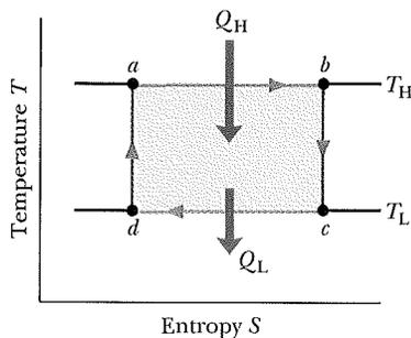
**Fig. 20-10** The Carnot cycle of Fig. 20-9 plotted on a temperature–entropy diagram. During processes  $ab$  and  $cd$  the temperature remains constant. During processes  $bc$  and  $da$  the entropy remains constant.
