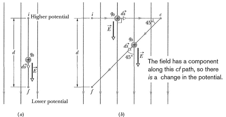
**Fig. 24-5** (a) A test charge  $q_0$  moves in a straight line from point  $i$  to point  $f$ , along the direction of a uniform external electric field. (b) Charge  $q_0$  moves along path  $icf$  in the same electric field.
