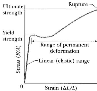
**Fig. 12-12** A stress–strain curve for a steel test specimen such as that of Fig. 12-11. The specimen deforms permanently when the stress is equal to the *yield strength* of the specimen's material. It ruptures when the stress is equal to the *ultimate strength* of the material.
