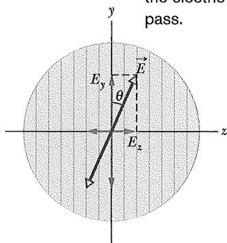
**Fig. 33-12** Polarized light approaching a polarizing sheet. The electric field  $\vec{E}$  of the light can be resolved into components  $E_y$  (parallel to the polarizing direction of the sheet) and  $E_z$  (perpendicular to that direction). Component  $E_y$  will be transmitted by the sheet; component  $E_z$  will be absorbed.
