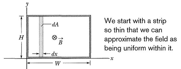
**Fig. 30-7** A closed conducting loop, of width  $W$  and height  $H$ , lies in a nonuniform, varying magnetic field that points directly into the page. To apply Faraday's law, we use the vertical strip of height  $H$ , width  $dx$ , and area  $dA$ .
