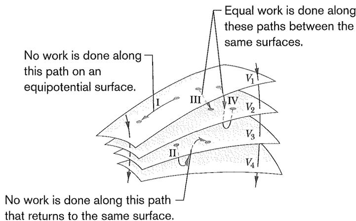
**Fig. 24-2** Portions of four equipotential surfaces at electric potentials  $V_1 = 100$  V,  $V_2 = 80$  V,  $V_3 = 60$  V, and  $V_4 = 40$  V. Four paths along which a test charge may move are shown. Two electric field lines are also indicated.
