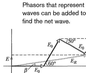
Phasors that represent waves can be added to find the net wave.
