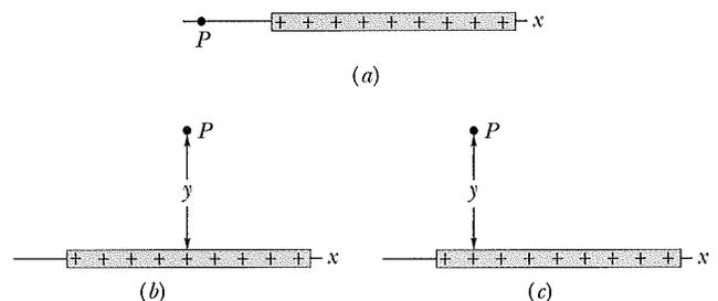
**Fig. 22-12** (a) Point  $P$  is on an extension of the line of charge. (b)  $P$  is on a line of symmetry of the line of charge, at perpendicular distance  $y$  from that line. (c) Same as (b) except that  $P$  is not on a line of symmetry.
