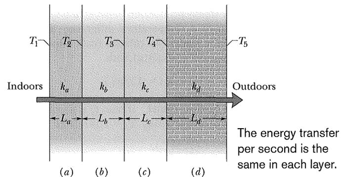
Fig. 18-22 Steady-state heat transfer through a wall.
