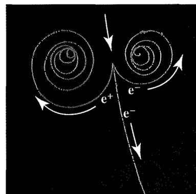
**Fig. 28-3** The tracks of two electrons ( $e^-$ ) and a positron ( $e^+$ ) in a bubble chamber that is immersed in a uniform magnetic field that is directed out of the plane of the page. (Lawrence Berkeley Laboratory/Photo Researchers)
