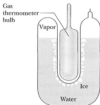
**Fig. 18-4** A triple-point cell, in which solid ice, liquid water, and water vapor coexist in thermal equilibrium. By international agreement, the temperature of this mixture has been defined to be 273.16 K. The bulb of a constant-volume gas thermometer is shown inserted into the well of the cell.
