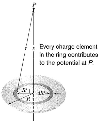
**Fig. 24-13** A plastic disk of radius  $R$ , charged on its top surface to a uniform surface charge density  $\sigma$ . We wish to find the potential  $V$  at point  $P$  on the central axis of the disk.
