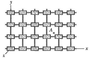
**Fig. 37-3** One section of a three-dimensional array of clocks and measuring rods by which an observer can assign spacetime coordinates to an event, such as a flash of light at point  $A$ . The event's space coordinates are approximately  $x = 3.6$  rod lengths,  $y = 1.3$  rod lengths, and  $z = 0$ . The time coordinate is whatever time appears on the clock closest to  $A$  at the instant of the flash.
