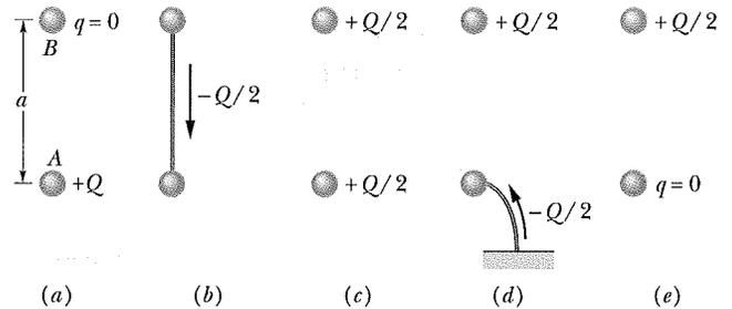
**Fig. 21-10** Two small conducting spheres *A* and *B*. (a) To start, sphere *A* is charged positively. (b) Negative charge is transferred from *B* to *A* through a connecting wire. (c) Both spheres are then charged positively. (d) Negative charge is transferred through a grounding wire to sphere *A*. (e) Sphere *A* is then neutral.
