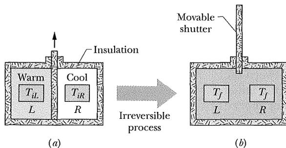
**Fig. 20-5** (a) In the initial state, two copper blocks  $L$  and  $R$ , identical except for their temperatures, are in an insulating box and are separated by an insulating shutter. (b) When the shutter is removed, the blocks exchange energy as heat and come to a final state, both with the same temperature  $T_f$ .
