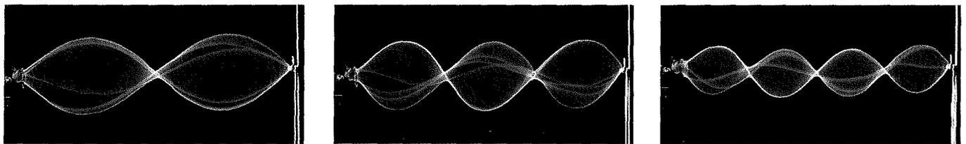
**Fig. 16-19** Stroboscopic photographs reveal (imperfect) standing wave patterns on a string being made to oscillate by an oscillator at the left end. The patterns occur at certain frequencies of oscillation. (Richard Megna/Fundamental Photographs)
