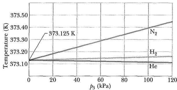
**Fig. 18-6** Temperatures measured by a constant-volume gas thermometer, with its bulb immersed in boiling water. For temperature calculations using Eq. 18-5, pressure  $p_3$  was measured at the triple point of water. Three different gases in the thermometer bulb gave generally different results at different gas pressures, but as the amount of gas was decreased (decreasing  $p_3$ ), all three curves converged to 373.125 K.
