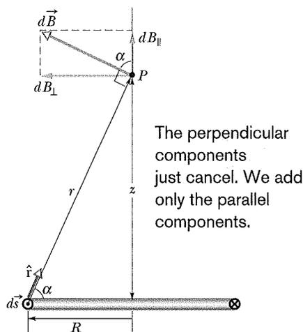
**Fig. 29-22** Cross section through a current loop of radius  $R$ . The plane of the loop is perpendicular to the page, and only the back half of the loop is shown. We use the law of Biot and Savart to find the magnetic field at point  $P$  on the central perpendicular axis of the loop.
