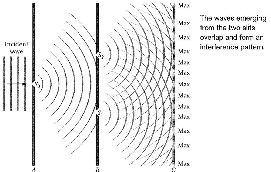
then spreads via diffraction to illuminate two slits  $S_1$  and  $S_2$  in screen  $B$ . Diffraction of the light by these two slits sends overlapping circular waves into the region beyond screen  $B$ , where the waves from one slit interfere with the waves from the other slit.
