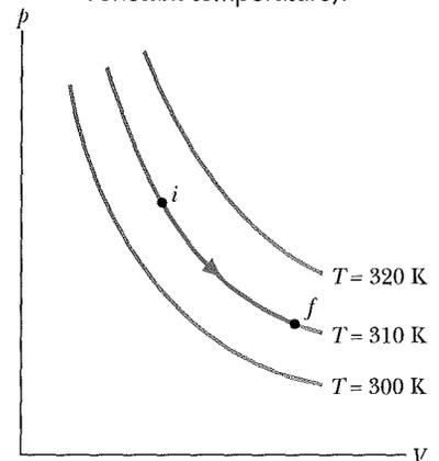
**Fig. 19-2** Three isotherms on a  $p$ - $V$  diagram. The path shown along the middle isotherm represents an isothermal expansion of a gas from an initial state  $i$  to a final state  $f$ . The path from  $f$  to  $i$  along the isotherm would represent the reverse process—that is, an isothermal compression.
