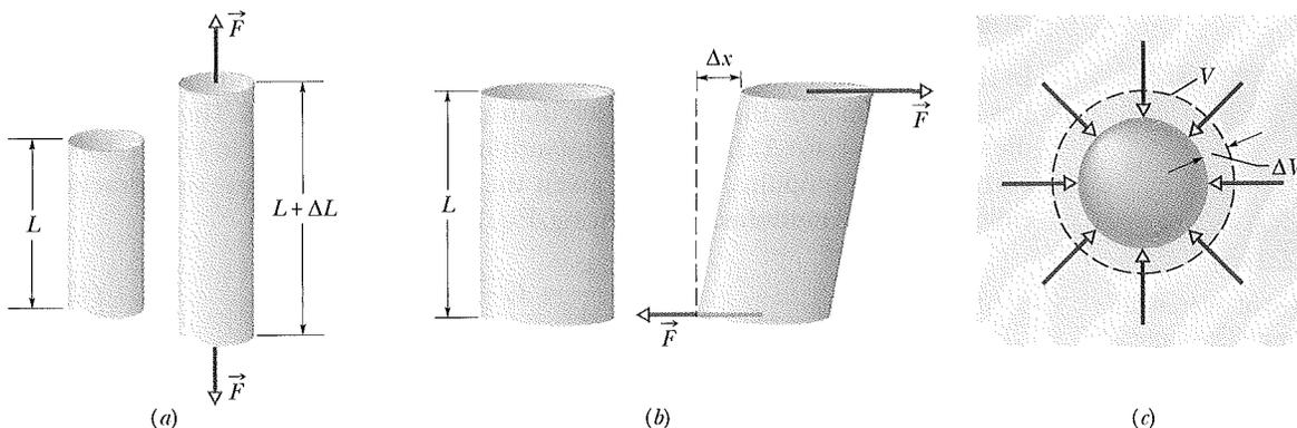
**Fig. 12-10** (a) A cylinder subject to *tensile stress* stretches by an amount  $\Delta L$ . (b) A cylinder subject to *shearing stress* deforms by an amount  $\Delta x$ , somewhat like a pack of playing cards would. (c) A solid sphere subject to uniform *hydraulic stress* from a fluid shrinks in volume by an amount  $\Delta V$ . All the deformations shown are greatly exaggerated.
