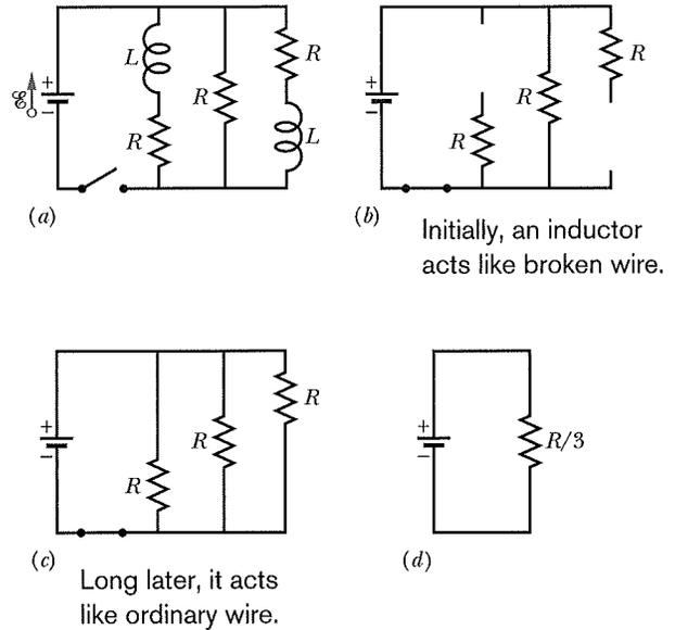
**Fig. 30-18** (a) A multiloop  $RL$  circuit with an open switch. (b) The equivalent circuit just after the switch has been closed. (c) The equivalent circuit a long time later. (d) The single-loop circuit that is equivalent to circuit (c).
