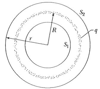
**Fig. 23-18** A thin, uniformly charged, spherical shell with total charge  $q$ , in cross section. Two Gaussian surfaces  $S_1$  and  $S_2$  are also shown in cross section. Surface  $S_2$  encloses the shell, and  $S_1$  encloses only the empty interior of the shell.
