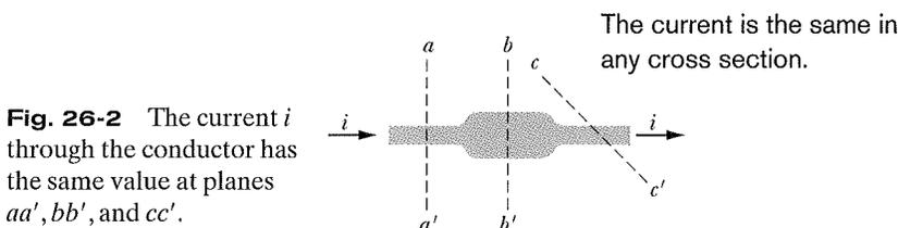
**Fig. 26-2** The current  $i$  through the conductor has the same value at planes  $aa'$ ,  $bb'$ , and  $cc'$ .
