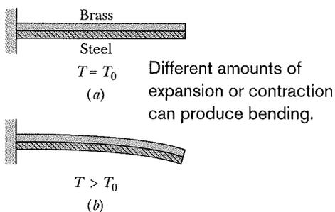
**Fig. 18-10** (a) A bimetal strip, consisting of a strip of brass and a strip of steel welded together, at temperature  $T_0$ . (b) The strip bends as shown at temperatures above this reference temperature. Below the reference temperature the strip bends the other way. Many thermostats operate on this principle, making and breaking an electrical contact as the temperature rises and falls.
