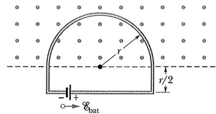
**Fig. 30-6** A battery is connected to a conducting loop that includes a half-circle of radius  $r$  lying in a uniform magnetic field. The field is directed out of the page; its magnitude is changing.
