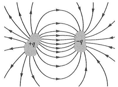
Fig. 25-2 Two conductors, isolated electrically from each other and from their surroundings, form a *capacitor*. When the capacitor is charged, the charges on the conductors, or *plates* as they are called, have the same magnitude  $q$  but opposite signs.
