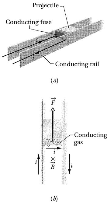
**Fig. 29-10** (a) A rail gun, as a current  $i$  is set up in it. The current rapidly causes the conducting fuse to vaporize. (b) The current produces a magnetic field  $\vec{B}$  between the rails, and the field causes a force  $\vec{F}$  to act on the conducting gas, which is part of the current path. The gas propels the projectile along the rails, launching it.
