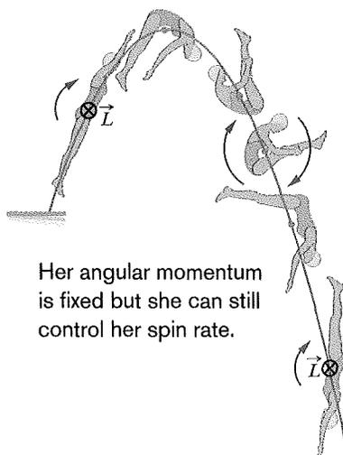
**Fig. 11-17** The diver's angular momentum  $\vec{L}$  is constant throughout the dive, being represented by the tail  $\otimes$  of an arrow that is perpendicular to the plane of the figure. Note also that her center of mass (see the dots) follows a parabolic path.
