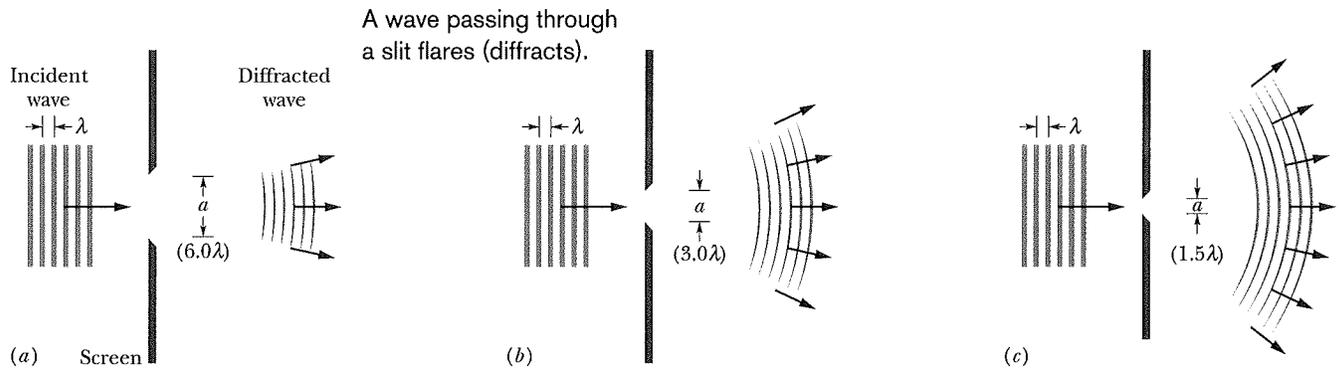
**Fig. 35-7** Diffraction represented schematically. For a given wavelength  $\lambda$ , the diffraction is more pronounced the smaller the slit width  $a$ . The figures show the cases for (a) slit width  $a = 6.0\lambda$ , (b) slit width  $a = 3.0\lambda$ , and (c) slit width  $a = 1.5\lambda$ . In all three cases, the screen and the length of the slit extend well into and out of the page, perpendicular to it.
