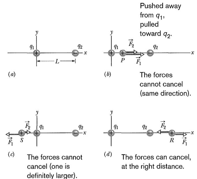
**Fig. 21-9** (a) Two particles of charges  $q_1$  and  $q_2$  are fixed in place on an  $x$  axis, with separation  $L$ . (b)–(d) Three possible locations  $P$ ,  $S$ , and  $R$  for a proton. At each location,  $\vec{F}_1$  is the force on the proton from particle 1 and  $\vec{F}_2$  is the force on the proton from particle 2.
