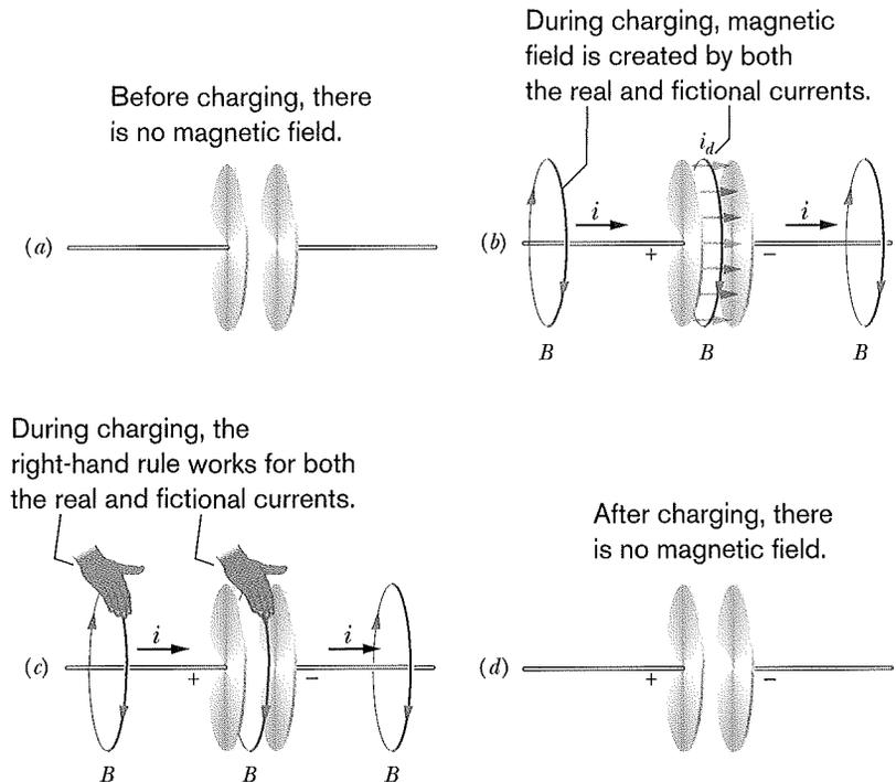
**Fig. 32-7** (a) Before and (d) after the plates are charged, there is no magnetic field. (b) During the charging, magnetic field is created by both the real current and the (fictional) displacement current. (c) The same right-hand rule works for both currents to give the direction of the magnetic field.
