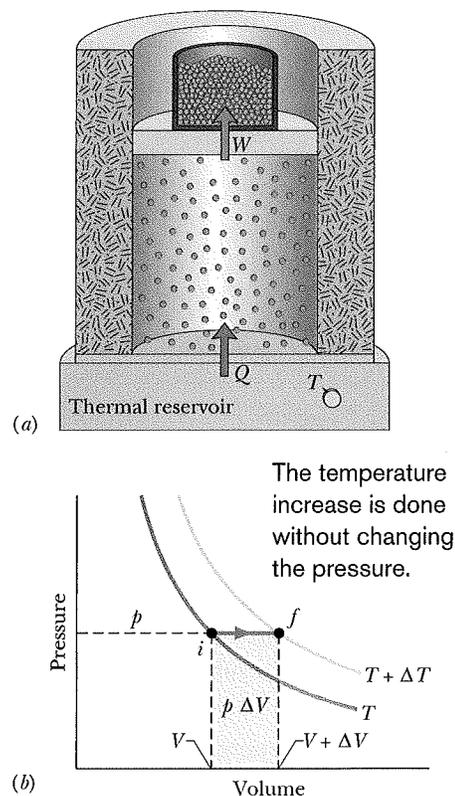
**Fig. 19-11** (a) The temperature of an ideal gas is raised from  $T$  to  $T + \Delta T$  in a constant-pressure process. Heat is added and work is done in lifting the loaded piston. (b) The process on a  $p$ - $V$  diagram. The work  $p \Delta V$  is given by the shaded area.
