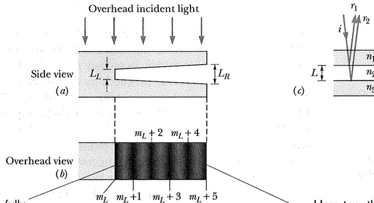
This dark fringe is due to fully destructive interference. So, the reflected rays must be *out of phase*.
