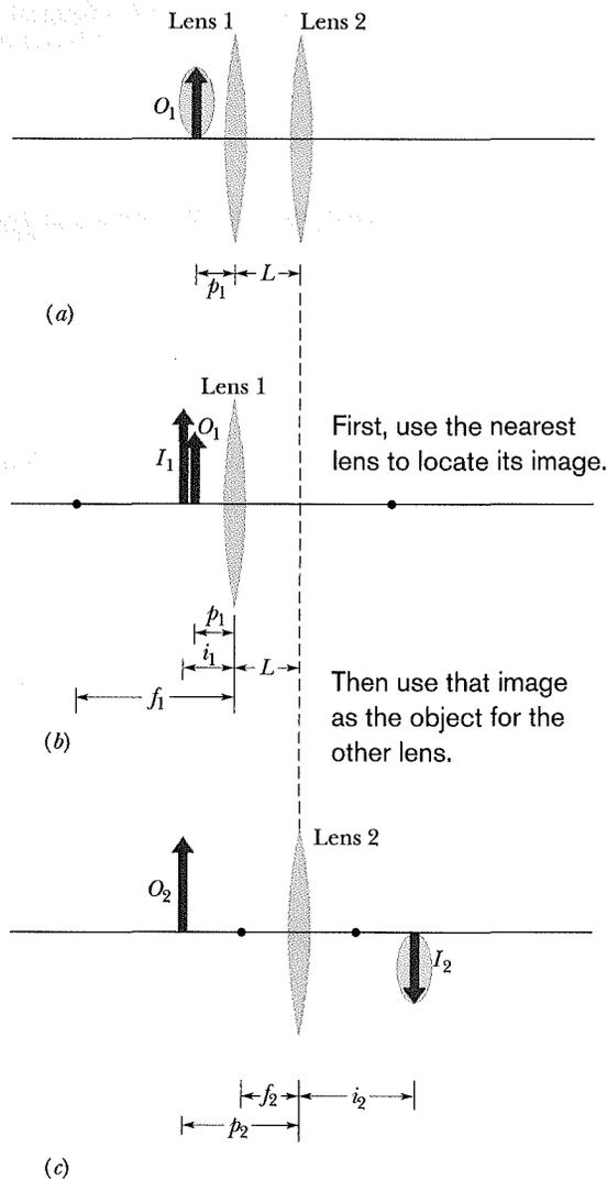
**Fig. 34-18** (a) Seed  $O_1$  is distance  $p_1$  from a two-lens system with lens separation  $L$ . We use the arrow to orient the seed. (b) The image  $I_1$  produced by lens 1 alone. (c) Image  $I_1$  acts as object  $O_2$  for lens 2 alone, which produces the final image  $I_2$ .
