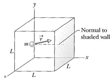
**Fig. 19-4** A cubical box of edge length  $L$ , containing  $n$  moles of an ideal gas. A molecule of mass  $m$  and velocity  $\vec{v}$  is about to collide with the shaded wall of area  $L^2$ . A normal to that wall is shown.
