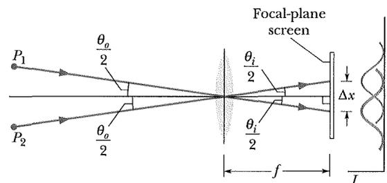
**Fig. 36-14** Light from two distant point objects  $P_1$  and  $P_2$  passes through a converging lens and forms images on a viewing screen in the focal plane of the lens. Only one representative ray from each object is shown. The images are not points but diffraction patterns, with intensities approximately as plotted at the right. The angular separation of the objects is  $\theta_o$  and that of the images is  $\theta_i$ ; the central maxima of the images have a separation  $\Delta x$ .
