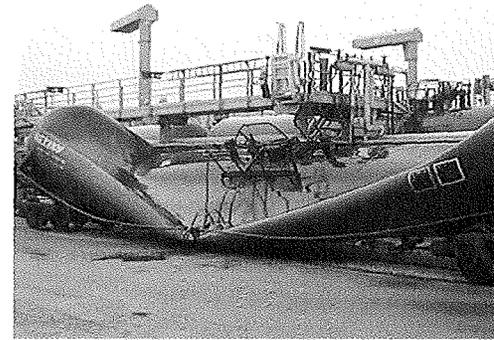
**Fig. 19-1** A railroad tank car crushed overnight. (Photo courtesy [www.Houston.RailFan.net](http://www.Houston.RailFan.net))
