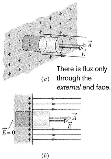
**Fig. 23-10** (a) Perspective view and (b) side view of a tiny portion of a large, isolated conductor with excess positive charge on its surface. A (closed) cylindrical Gaussian surface, embedded perpendicularly in the conductor, encloses some of the charge. Electric field lines pierce the external end cap of the cylinder, but not the internal end cap. The external end cap has area  $A$  and area vector  $\vec{A}$ .
