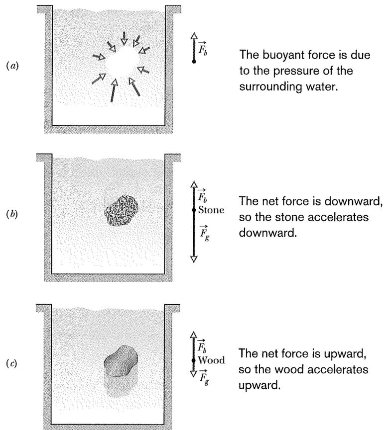
**Fig. 14-10** (a) The water surrounding the hole in the water produces a net upward buoyant force on whatever fills the hole. (b) For a stone of the same volume as the hole, the gravitational force exceeds the buoyant force in magnitude. (c) For a lump of wood of the same volume as the hole, the gravitational force is less than the buoyant force in magnitude.
