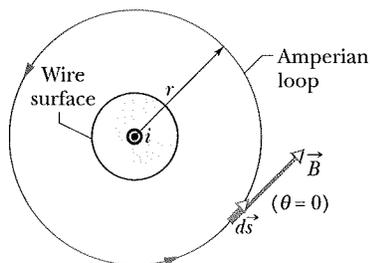
**Fig. 29-13** Using Ampere's law to find the magnetic field that a current  $i$  produces outside a long straight wire of circular cross section. The Amperian loop is a concentric circle that lies outside the wire.
