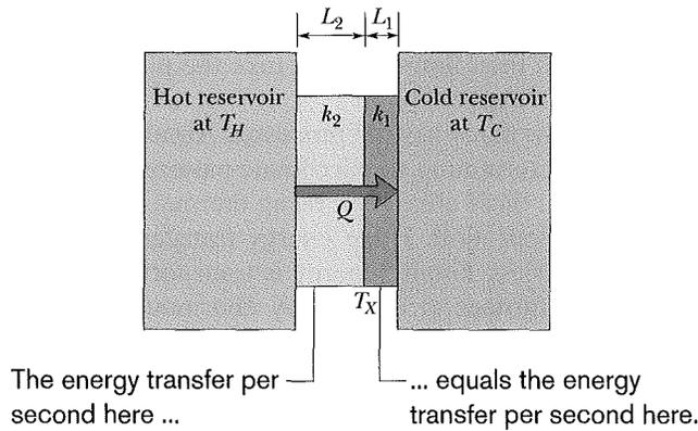
**Fig. 18-19** Heat is transferred at a steady rate through a composite slab made up of two different materials with different thicknesses and different thermal conductivities. The steady-state temperature at the interface of the two materials is  $T_X$ .
