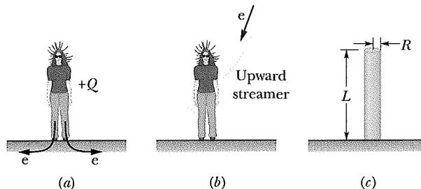
**Fig. 23-14** (a) Some of the conduction electrons in the woman's body are driven into the ground, leaving her positively charged. (b) An upward streamer develops if the air undergoes electrical breakdown, which provides a path for electrons freed from molecules in the air to move to the woman. (c) A cylinder represents the woman.
