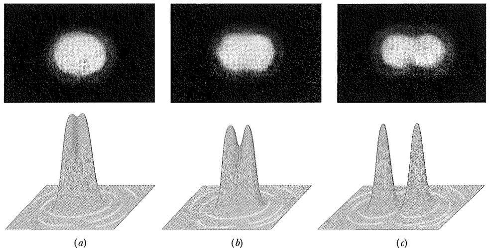
**Fig. 36-11** At the top, the images of two point sources (stars) formed by a converging lens. At the bottom, representations of the image intensities. In (a) the angular separation of the sources is too small for them to be distinguished, in (b) they can be marginally distinguished, and in (c) they are clearly distinguished. Rayleigh's criterion is satisfied in (b), with the central maximum of one diffraction pattern coinciding with the first minimum of the other.
