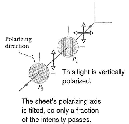
**Fig. 33-13** The light transmitted by polarizing sheet  $P_1$  is vertically polarized, as represented by the vertical double arrow. The amount of that light that is then transmitted by polarizing sheet  $P_2$  depends on the angle between the polarization direction of that light and the polarizing direction of  $P_2$  (indicated by the lines drawn in the sheet and by the dashed line).
