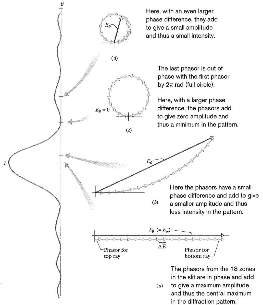
**Fig. 36-7** Phasor diagrams for  $N = 18$  phasors, corresponding to the division of a single slit into 18 zones. Resultant amplitudes  $E_\theta$  are shown for (a) the central maximum at  $\theta = 0$ , (b) a point on the screen lying at a small angle  $\theta$  to the central axis, (c) the first minimum, and (d) the first side maximum.
