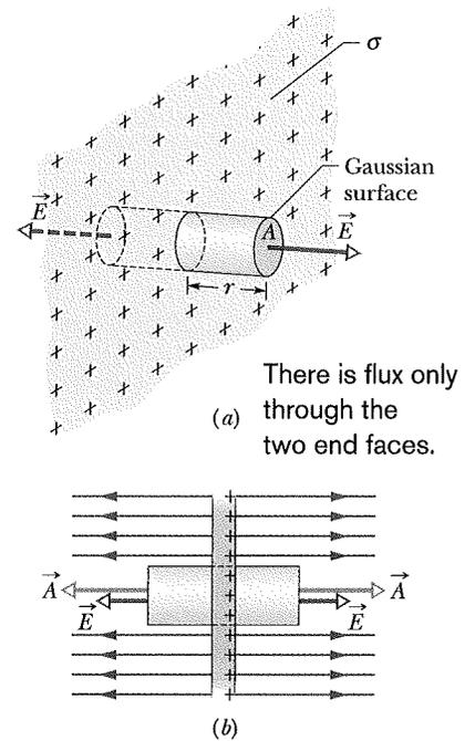
**Fig. 23-15** (a) Perspective view and (b) side view of a portion of a very large, thin plastic sheet, uniformly charged on one side to surface charge density  $\sigma$ . A closed cylindrical Gaussian surface passes through the sheet and is perpendicular to it.
