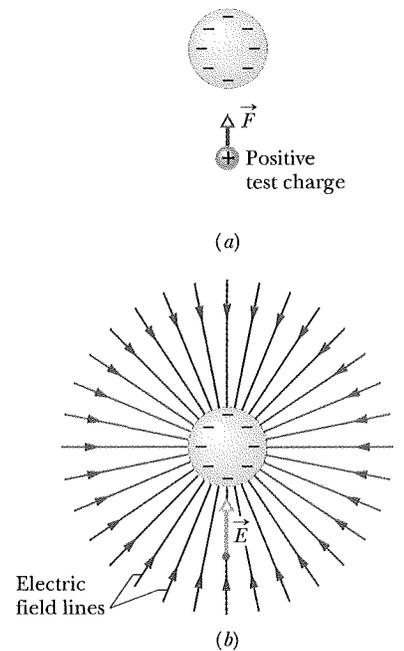
**Fig. 22-2** (a) The electrostatic force  $\vec{F}$  acting on a positive test charge near a sphere of uniform negative charge. (b) The electric field vector  $\vec{E}$  at the location of the test charge, and the electric field lines in the space near the sphere. The field lines extend *toward* the negatively charged sphere. (They originate on distant positive charges.)
