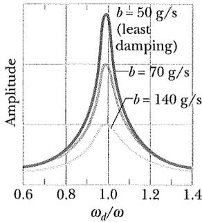
**Fig. 15-16** The displacement amplitude  $x_m$  of a forced oscillator varies as the angular frequency  $\omega_d$  of the driving force is varied. The curves here correspond to three values of the damping constant  $b$ .
