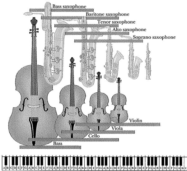
**Fig. 17-15** The saxophone and violin families, showing the relations between instrument length and frequency range. The frequency range of each instrument is indicated by a horizontal bar along a frequency scale suggested by the keyboard at the bottom; the frequency increases toward the right.
