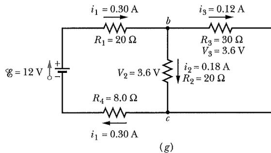
**Fig. 27-11** (a) A circuit with an ideal battery. (b) Label the currents. (c) Replacing the parallel resistors with their equivalent. (d) – (g) Working backward to find the currents through the parallel resistors.
