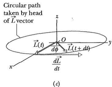
**Fig. 11-22** (a) A nonspinning gyroscope falls by rotating in an  $xz$  plane because of torque  $\vec{\tau}$ . (b) A rapidly spinning gyroscope, with angular momentum  $\vec{L}$ , precesses around the  $z$  axis. Its precessional motion is in the  $xy$  plane. (c) The change  $d\vec{L}/dt$  in angular momentum leads to a rotation of  $\vec{L}$  about  $O$ .
