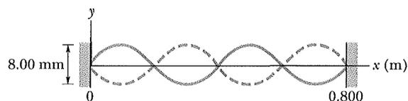
**Fig. 16-22** Resonant oscillation of a string under tension.
