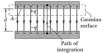
**Fig. 25-5** A charged parallel-plate capacitor. A Gaussian surface encloses the charge on the positive plate. The integration of Eq. 25-6 is taken along a path extending directly from the negative plate to the positive plate.
