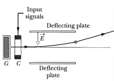
**Fig. 22-15** Ink-jet printer. Drops shot from generator  $G$  receive a charge in charging unit  $C$ . An input signal from a computer controls the charge and thus the effect of field  $\vec{E}$  on where the drop lands on the paper.
