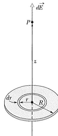
**Fig. 22-13** A disk of radius  $R$  and uniform positive charge. The ring shown has radius  $r$  and radial width  $dr$ . It sets up a differential electric field  $d\vec{E}$  at point  $P$  on its central axis.
