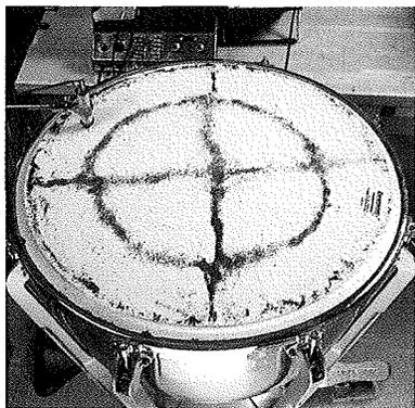
**Fig. 16-21** One of many possible standing wave patterns for a kettledrum head, made visible by dark powder sprinkled on the drumhead. As the head is set into oscillation at a single frequency by a mechanical oscillator at the upper left of the photograph, the powder collects at the nodes, which are circles and straight lines in this two-dimensional example. (Courtesy Thomas D. Rossing, Northern Illinois University)
