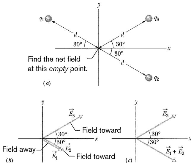
**Fig. 22-7** (a) Three particles with charges  $q_1$ ,  $q_2$ , and  $q_3$  are at the same distance  $d$  from the origin. (b) The electric field vectors  $\vec{E}_1$ ,  $\vec{E}_2$ , and  $\vec{E}_3$ , at the origin due to the three particles. (c) The electric field vector  $\vec{E}_3$  and the vector sum  $\vec{E}_1 + \vec{E}_2$  at the origin.
