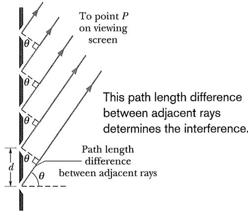
(Fig. 36-21). At such a minimum, the  $N$  rays from the  $N$  slits of the grating cancel one another. (The actual width of the central line is, of course,  $2(\Delta\theta_{hw})$ , but line widths are usually compared via half-widths.)
