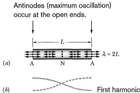
**Fig. 17-13** (a) The simplest standing wave pattern of displacement for (longitudinal) sound waves in a pipe with both ends open has an antinode (A) across each end and a node (N) across the middle. (The longitudinal displacements represented by the double arrows are greatly exaggerated.) (b) The corresponding standing wave pattern for (transverse) string waves.
