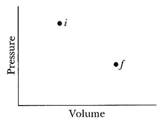
**Fig. 20-2** A *p-V* diagram showing the initial state *i* and the final state *f* of the free expansion of Fig. 20-1. The intermediate states of the gas cannot be shown because they are not equilibrium states.
