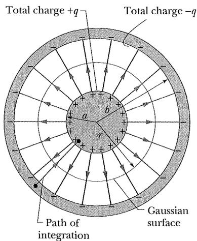
**Fig. 25-6** A cross section of a long cylindrical capacitor, showing a cylindrical Gaussian surface of radius  $r$  (that encloses the positive plate) and the radial path of integration along which Eq. 25-6 is to be applied. This figure also serves to illustrate a spherical capacitor in a cross section through its center.
