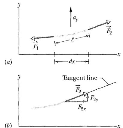
**Fig. 16-10** (a) A string element as a sinusoidal transverse wave travels on a stretched string. Forces  $\vec{F}_1$  and  $\vec{F}_2$  act at the left and right ends, producing acceleration  $\vec{a}$  having a vertical component  $a_y$ . (b) The force at the element's right end is directed along a tangent to the element's right side.
