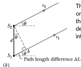
The  $\Delta L$  shifts one wave from the other, which determines the interference.
