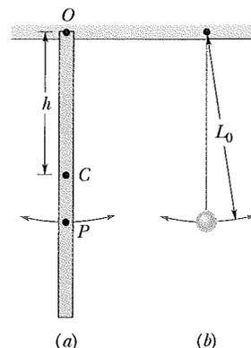
**Fig. 15-11** (a) A meter stick suspended from one end as a physical pendulum. (b) A simple pendulum whose length  $L_0$  is chosen so that the periods of the two pendulums are equal. Point  $P$  on the pendulum of (a) marks the center of oscillation.
