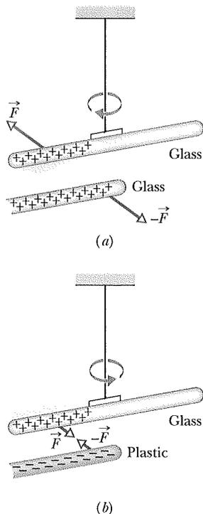
**Fig. 21-2** (a) Two charged rods of the same sign repel each other. (b) Two charged rods of opposite signs attract each other. Plus signs indicate a positive net charge, and minus signs indicate a negative net charge.
