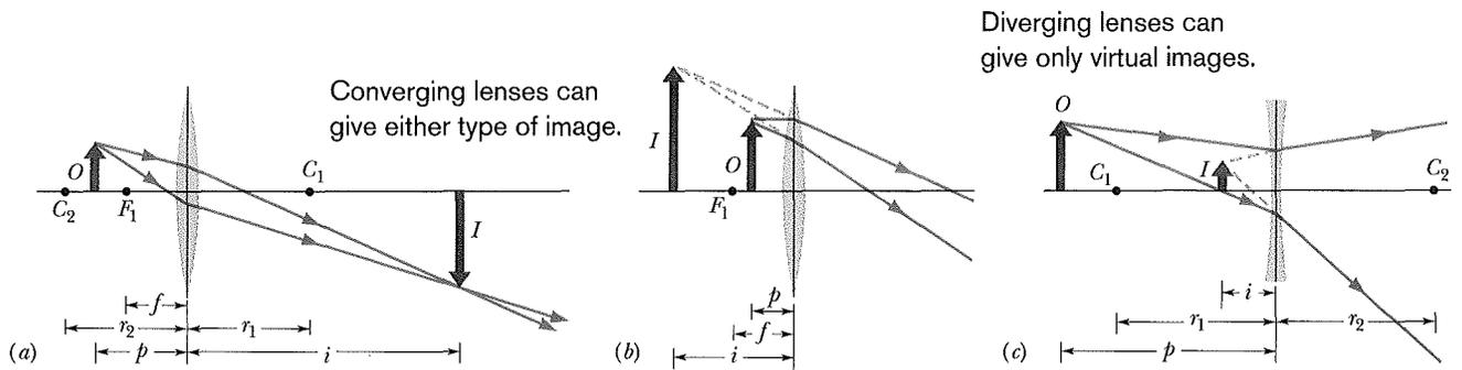
**Fig. 34-15** (a) A real, inverted image  $I$  is formed by a converging lens when the object  $O$  is outside the focal point  $F_1$ . (b) The image  $I$  is virtual and has the same orientation as  $O$  when  $O$  is inside the focal point. (c) A diverging lens forms a virtual image  $I$ , with the same orientation as the object  $O$ , whether  $O$  is inside or outside the focal point of the lens.
