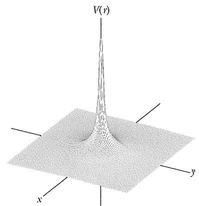
**Fig. 24-7** A computer-generated plot of the electric potential  $V(r)$  due to a positive point charge located at the origin of an  $xy$  plane. The potentials at points in the  $xy$  plane are plotted vertically. (Curved lines have been added to help you visualize the plot.) The infinite value of  $V$  predicted by Eq. 24-26 for  $r = 0$  is not plotted.
