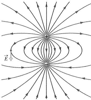
**Fig. 22-5** Field lines for a positive point charge and a nearby negative point charge that are equal in magnitude. The charges attract each other. The pattern of field lines and the electric field it represents have rotational symmetry about an axis passing through both charges in the plane of the page. The electric field vector at one point is shown; the vector is tangent to the field line through the point.
