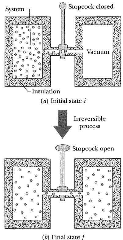
**Fig. 20-1** The free expansion of an ideal gas. (a) The gas is confined to the left half of an insulated container by a closed stopcock. (b) When the stopcock is opened, the gas rushes to fill the entire container. This process is irreversible; that is, it does not occur in reverse, with the gas spontaneously collecting itself in the left half of the container.
