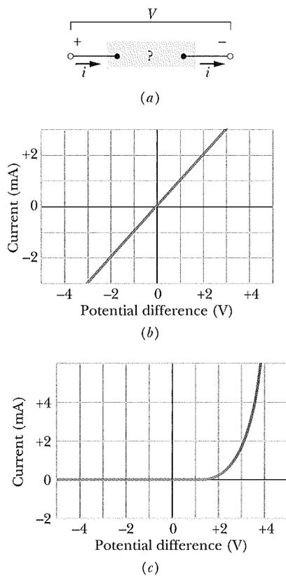
**Fig. 26-11** (a) A potential difference  $V$  is applied to the terminals of a device, establishing a current  $i$ . (b) A plot of current  $i$  versus applied potential difference  $V$  when the device is a 1000  $\Omega$  resistor. (c) A plot when the device is a semiconducting  $pn$  junction diode.
