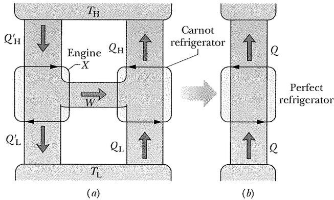
**Fig. 20-16** (a) Engine  $X$  drives a Carnot refrigerator. (b) If, as claimed, engine  $X$  is more efficient than a Carnot engine, then the combination shown in (a) is equivalent to the perfect refrigerator shown here. This violates the second law of thermodynamics, so we conclude that engine  $X$  cannot be more efficient than a Carnot engine.
