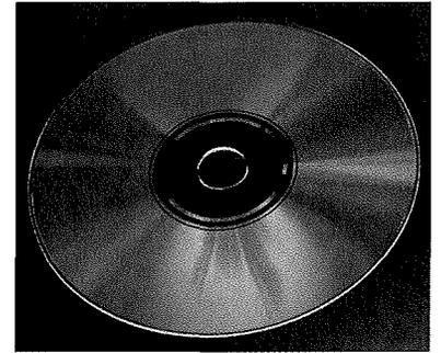
The fine rulings, each  $0.5 \mu\text{m}$  wide, on a compact disc function as a diffraction grating. When a small source of white light illuminates a disc, the diffracted light forms colored “lanes” that are the composite of the diffraction patterns from the rulings.
