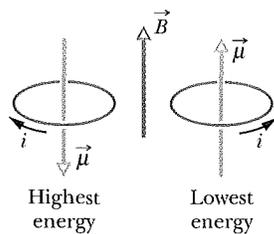
**Fig. 28-20** The orientations of highest and lowest energy of a magnetic dipole (here a coil carrying current) in an external magnetic field  $\vec{B}$ . The direction of the current  $i$  gives the direction of the magnetic dipole moment  $\vec{\mu}$  via the right-hand rule shown for  $\vec{n}$  in Fig. 28-19b.
