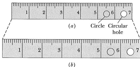
**Fig. 18-11** The same steel ruler at two different temperatures. When it expands, the scale, the numbers, the thickness, and the diameters of the circle and circular hole are all increased by the same factor. (The expansion has been exaggerated for clarity.)
