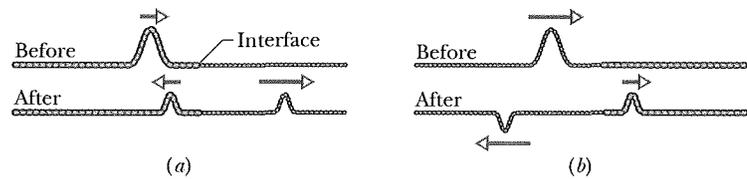
**Fig. 35-16** Phase changes when a pulse is reflected at the interface between two stretched strings of different linear densities. The wave speed is greater in the lighter string. (a) The incident pulse is in the denser string. (b) The incident pulse is in the lighter string. Only here is there a phase change, and only in the reflected wave.
