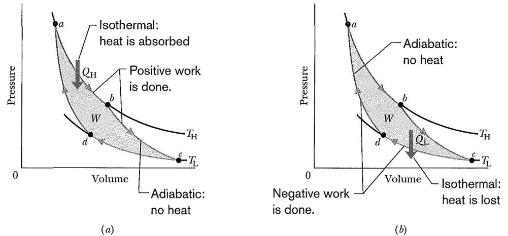
**Fig. 20-9** A pressure–volume plot of the cycle followed by the working substance of the Carnot engine in Fig. 20-8. The cycle consists of two isothermal ( $ab$  and  $cd$ ) and two adiabatic processes ( $bc$  and  $da$ ). The shaded area enclosed by the cycle is equal to the work  $W$  per cycle done by the Carnot engine.
