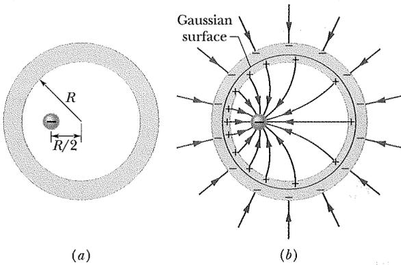
**Fig. 23-11** (a) A negative point charge is located within a spherical metal shell that is electrically neutral. (b) As a result, positive charge is nonuniformly distributed on the inner wall of the shell, and an equal amount of negative charge is uniformly distributed on the outer wall.
