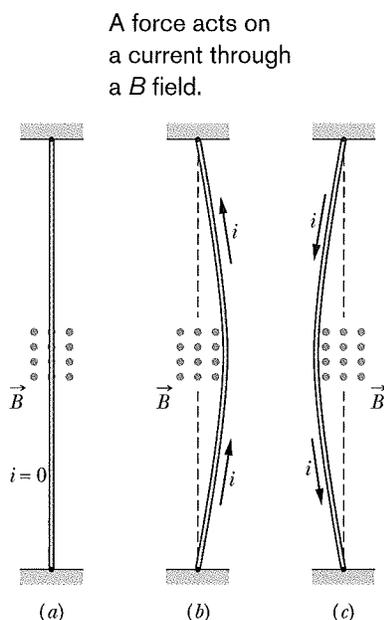
**Fig. 28-14** A flexible wire passes between the pole faces of a magnet (only the farther pole face is shown). (a) Without current in the wire, the wire is straight. (b) With upward current, the wire is deflected rightward. (c) With downward current, the deflection is leftward. The connections for getting the current into the wire at one end and out of it at the other end are not shown.
