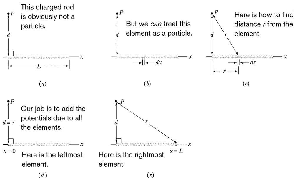
**Fig. 24-12** (a) A thin, uniformly charged rod produces an electric potential  $V$  at point  $P$ . (b) An element can be treated as a particle. (c) The potential at  $P$  due to the element depends on the distance  $r$ . We need to sum the potentials due to all the elements, from the left side (d) to the right side (e).
