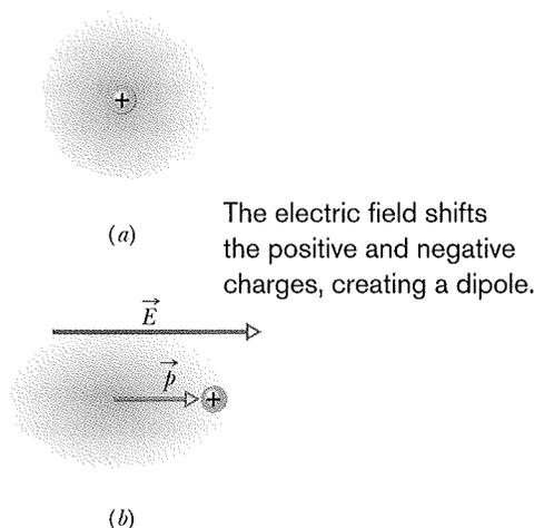
**Fig. 24-11** (a) An atom, showing the positively charged nucleus (green) and the negatively charged electrons (gold shading). The centers of positive and negative charge coincide. (b) If the atom is placed in an external electric field  $\vec{E}$ , the electron orbits are distorted so that the centers of positive and negative charge no longer coincide. An induced dipole moment  $\vec{p}$  appears. The distortion is greatly exaggerated here.
