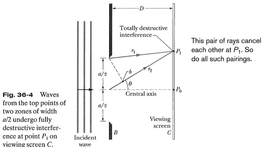
**Fig. 36-4** Waves from the top points of two zones of width  $a/2$  undergo fully destructive interference at point  $P_1$  on viewing screen  $C$ .
