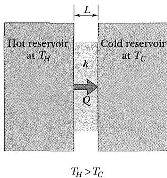
**Fig. 18-18** Thermal conduction. Energy is transferred as heat from a reservoir at temperature  $T_H$  to a cooler reservoir at temperature  $T_C$  through a conducting slab of thickness  $L$  and thermal conductivity  $k$ .
