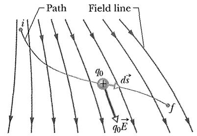
**Fig. 24-4** A test charge  $q_0$  moves from point  $i$  to point  $f$  along the path shown in a nonuniform electric field. During a displacement  $d\vec{s}$ , an electrostatic force  $q_0\vec{E}$  acts on the test charge. This force points in the direction of the field line at the location of the test charge.
