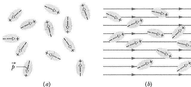
The initial electric field inside this nonpolar dielectric slab is zero.
