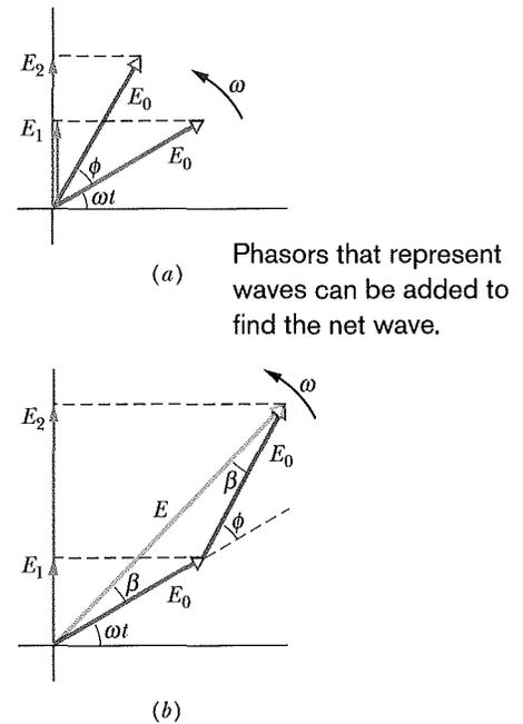
**Fig. 35-13** (a) Phasors representing, at time  $t$ , the electric field components given by Eqs. 35-20 and 35-21. Both phasors have magnitude  $E_0$  and rotate with angular speed  $\omega$ . Their phase difference is  $\phi$ . (b) Vector addition of the two phasors gives the phasor representing the resultant wave, with amplitude  $E$  and phase constant  $\beta$ .
