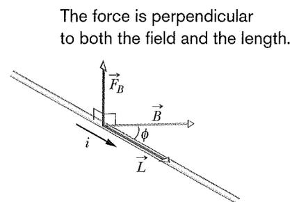
**Fig. 28-16** A wire carrying current  $i$  makes an angle  $\phi$  with magnetic field  $\vec{B}$ . The wire has length  $L$  in the field and length vector  $\vec{L}$  (in the direction of the current). A magnetic force  $\vec{F}_B = i\vec{L} \times \vec{B}$  acts on the wire.
