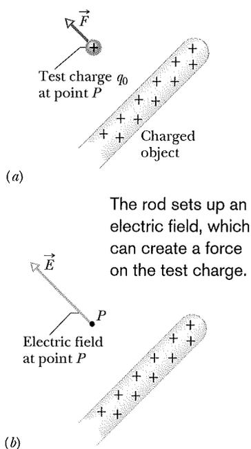
**Fig. 22-1** (a) A positive test charge  $q_0$  placed at point  $P$  near a charged object. An electrostatic force  $\vec{F}$  acts on the test charge. (b) The electric field  $\vec{E}$  at point  $P$  produced by the charged object.
