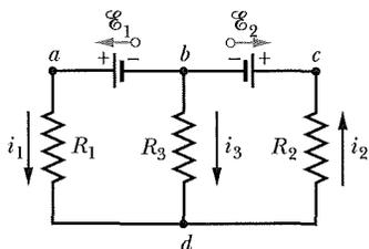
**Fig. 27-9** A multiloop circuit consisting of three branches: left-hand branch  $bad$ , right-hand branch  $bcd$ , and central branch  $bd$ . The circuit also consists of three loops: left-hand loop  $badb$ , right-hand loop  $bcd$ , and big loop  $badcb$ .
