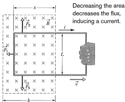
**Fig. 30-8** You pull a closed conducting loop out of a magnetic field at constant velocity  $\vec{v}$ . While the loop is moving, a clockwise current  $i$  is induced in the loop, and the loop segments still within the magnetic field experience forces  $\vec{F}_1$ ,  $\vec{F}_2$ , and  $\vec{F}_3$ .
