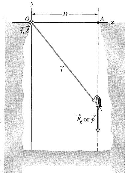
**Fig. 11-14** A penguin falls vertically from point  $A$ . The torque  $\vec{\tau}$  and the angular momentum  $\vec{\ell}$  of the falling penguin with respect to the origin  $O$  are directed into the plane of the figure at  $O$ .
