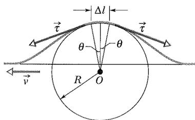
**Fig. 16-8** A symmetrical pulse, viewed from a reference frame in which the pulse is stationary and the string appears to move right to left with speed  $v$ . We find speed  $v$  by applying Newton's second law to a string element of length  $\Delta l$ , located at the top of the pulse.
