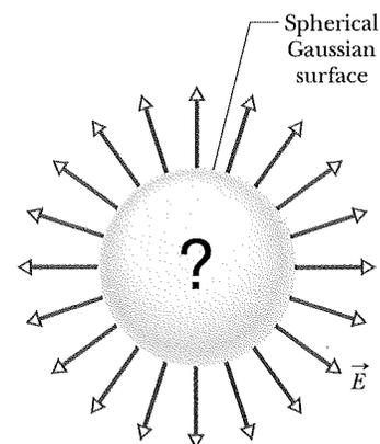
**Fig. 23-1** A spherical Gaussian surface. If the electric field vectors are of uniform magnitude and point radially outward at all surface points, you can conclude that a net positive distribution of charge must lie within the surface and have spherical symmetry.
