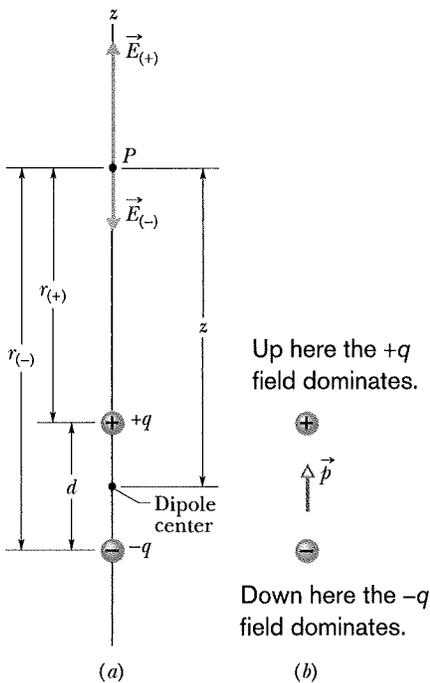
**Fig. 22-8** (a) An electric dipole. The electric field vectors  $\vec{E}_{(+)}$  and  $\vec{E}_{(-)}$  at point  $P$  on the dipole axis result from the dipole's two charges. Point  $P$  is at distances  $r_{(+)}$  and  $r_{(-)}$  from the individual charges that make up the dipole. (b) The dipole moment  $\vec{p}$  of the dipole points from the negative charge to the positive charge.
