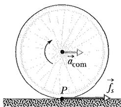
**Fig. 11-7** A wheel rolls horizontally without sliding while accelerating with linear acceleration  $\vec{a}_{\text{com}}$ . A static frictional force  $\vec{f}_s$  acts on the wheel at  $P$ , opposing its tendency to slide.
