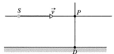
**Fig. 37-12** A light source  $S$  travels with velocity  $\vec{v}$  past a detector at  $D$ . The special theory of relativity predicts a transverse Doppler effect as the source passes through point  $P$ , where the direction of travel is perpendicular to the line extending through  $D$ . Classical theory predicts no such effect.
