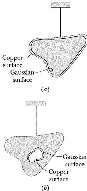
**Fig. 23-9** (a) A lump of copper with a charge  $q$  hangs from an insulating thread. A Gaussian surface is placed within the metal, just inside the actual surface. (b) The lump of copper now has a cavity within it. A Gaussian surface lies within the metal, close to the cavity surface.
