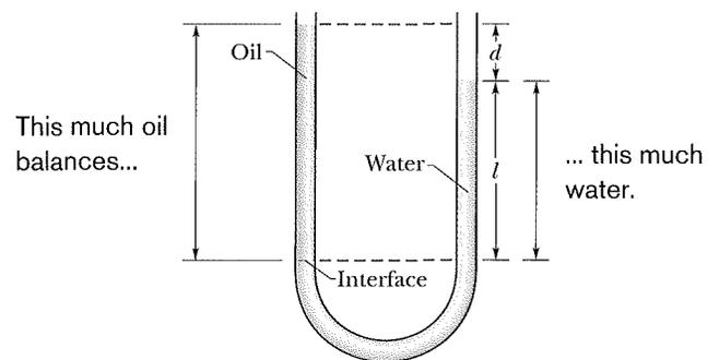
**Fig. 14-4** The oil in the left arm stands higher than the water in the right arm because the oil is less dense than the water. Both fluid columns produce the same pressure  $p_{\text{int}}$  at the level of the interface.
