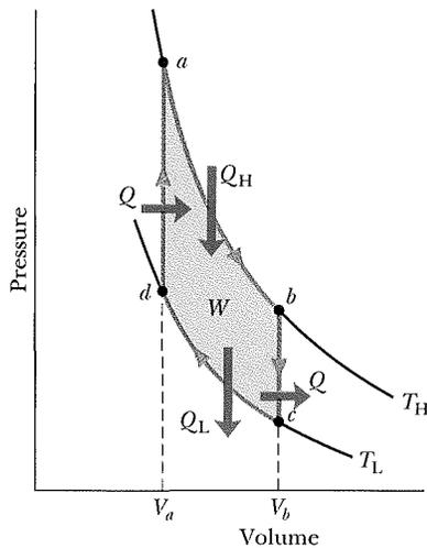
**Fig. 20-13** A  $p$ - $V$  plot for the working substance of an ideal Stirling engine, with working substance assumed for convenience to be an ideal gas.
