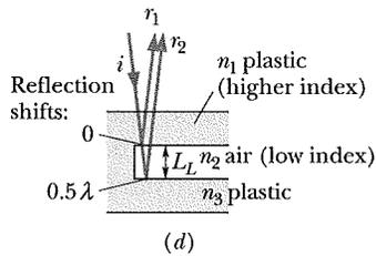
The path length difference (down and back up) is  $2L$ .
