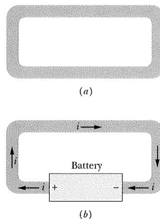
**Fig. 26-1** (a) A loop of copper in electrostatic equilibrium. The entire loop is at a single potential, and the electric field is zero at all points inside the copper. (b) Adding a battery imposes an electric potential difference between the ends of the loop that are connected to the terminals of the battery. The battery thus produces an electric field within the loop, from terminal to terminal, and the field causes charges to move around the loop. This movement of charges is a current  $i$ .
