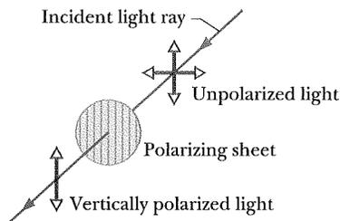
**Fig. 33-11** Unpolarized light becomes polarized when it is sent through a polarizing sheet. Its direction of polarization is then parallel to the polarizing direction of the sheet, which is represented here by the vertical lines drawn in the sheet.
