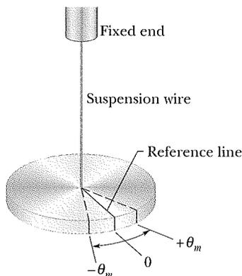
**Fig. 15-7** A torsion pendulum is an angular version of a linear simple harmonic oscillator. The disk oscillates in a horizontal plane; the reference line oscillates with angular amplitude  $\theta_m$ . The twist in the suspension wire stores potential energy as a spring does and provides the restoring torque.
