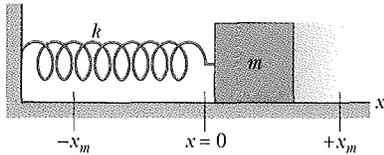
**Fig. 15-5** A linear simple harmonic oscillator. The surface is frictionless. Like the particle of Fig. 15-1, the block moves in simple harmonic motion once it has been either pulled or pushed away from the  $x = 0$  position and released. Its displacement is then given by Eq. 15-3.
