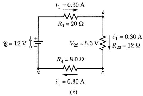
Parallel resistors and their equivalent have the same  $V$  ("par- $V$ ").
