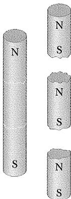
**Fig. 32-3** If you break a magnet, each fragment becomes a separate magnet, with its own north and south poles.
