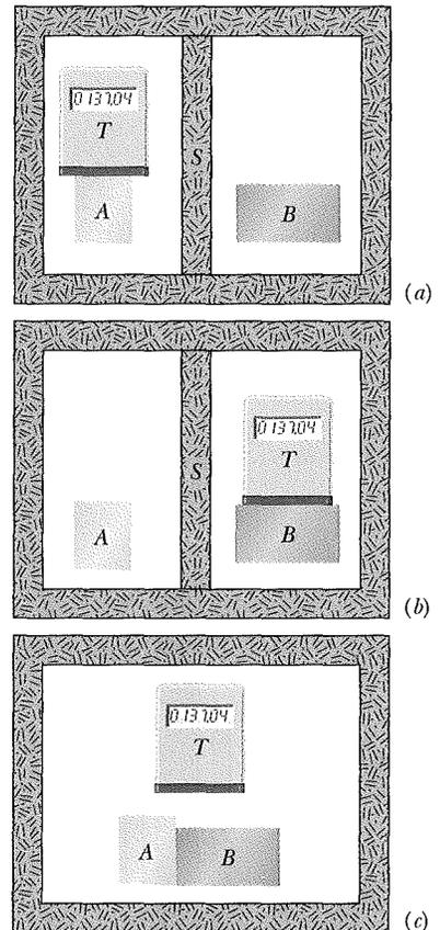
**Fig. 18-3** (a) Body  $T$  (a thermoscope) and body  $A$  are in thermal equilibrium. (Body  $S$  is a thermally insulating screen.) (b) Body  $T$  and body  $B$  are also in thermal equilibrium, at the same reading of the thermoscope. (c) If (a) and (b) are true, the zeroth law of thermodynamics states that body  $A$  and body  $B$  are also in thermal equilibrium.
