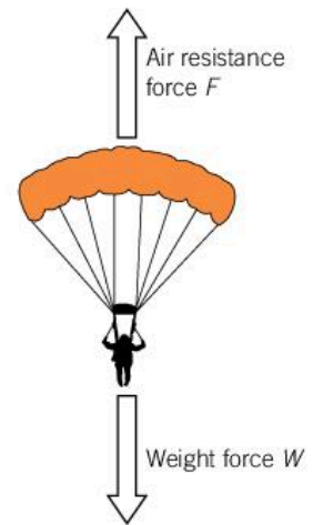
▲ Figure 4.2 The forces are balanced ( F = W ) so the parachutist falls at a constant speed
