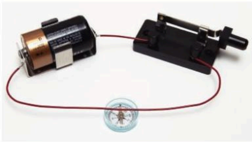
▲ Oersted's experiment showed that electricity and magnetism were linked.
