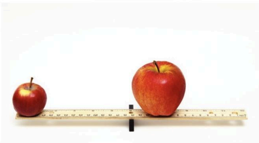
▲ These apples are in equilibrium because the clockwise moment equals the anticlockwise moment.
