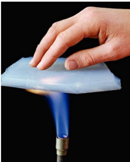
▲ This special material is called aerogel. Energy is transferred very slowly through it.
