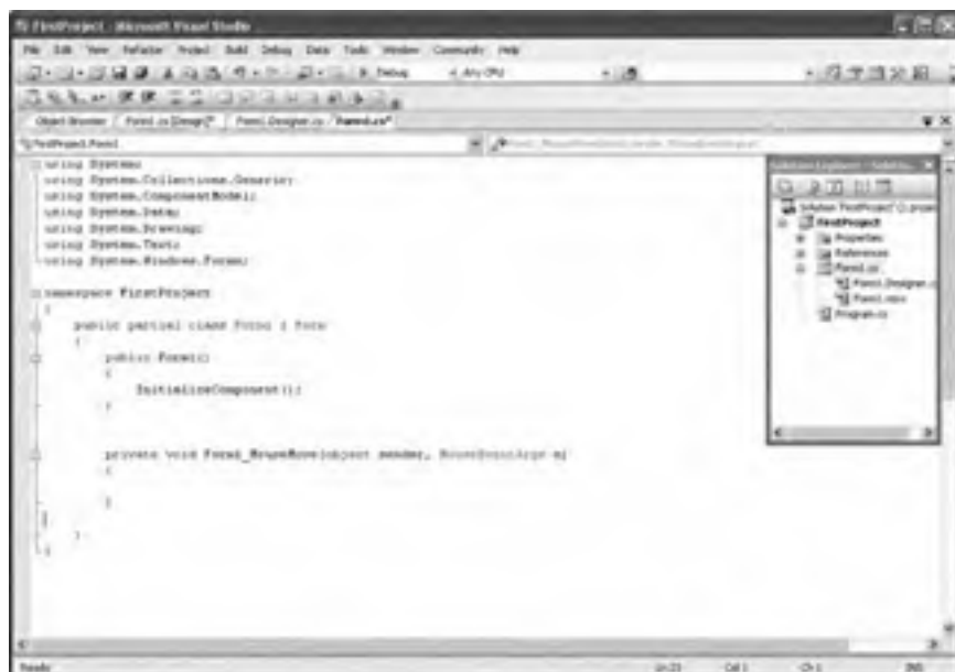
Figure 3-9 Event procedure stub for the Move event of the form.
