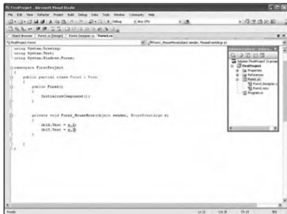
Figure 3-11 Incorrect code highlighted.
