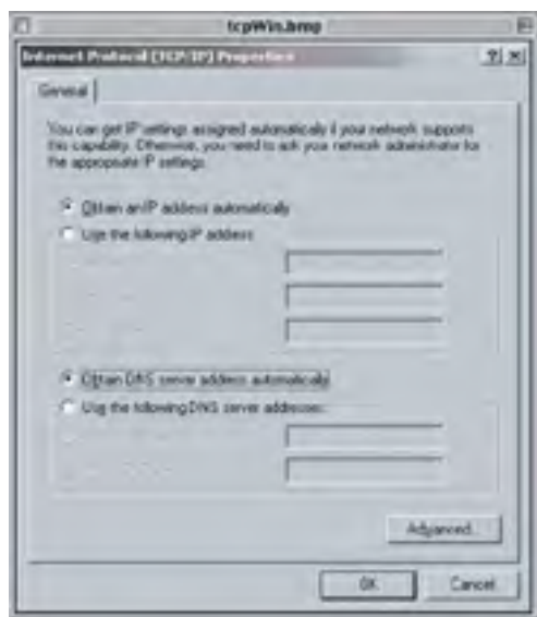
Figure 5.5: TCP/IP control panel (Windows NT)
