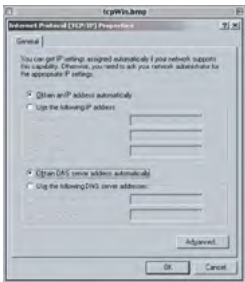
Figure 5.5: TCP/IP control panel (Windows NT)
