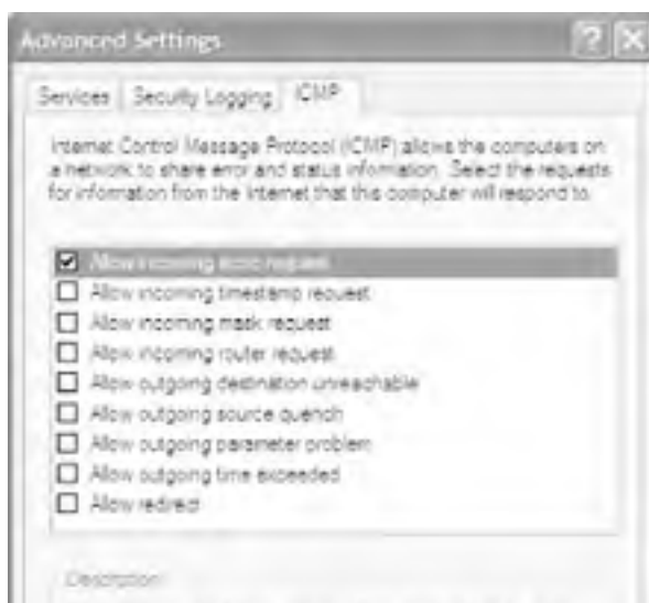
Figure 5-22. Using the ICMP tab to allow diagnostic services to bypass the ICF
