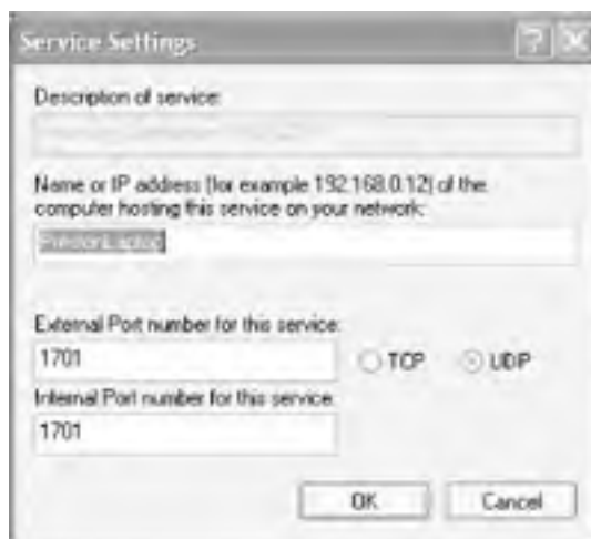
Figure 5-20. Customizing an inbound service that you want to pass through the ICF
