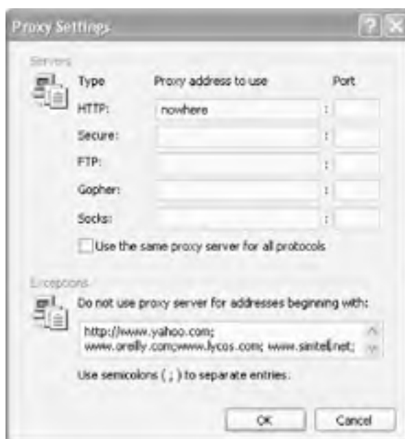
Figure 5-13. Use the Proxy Setting dialog box to limit the Web sites your PC can visit
