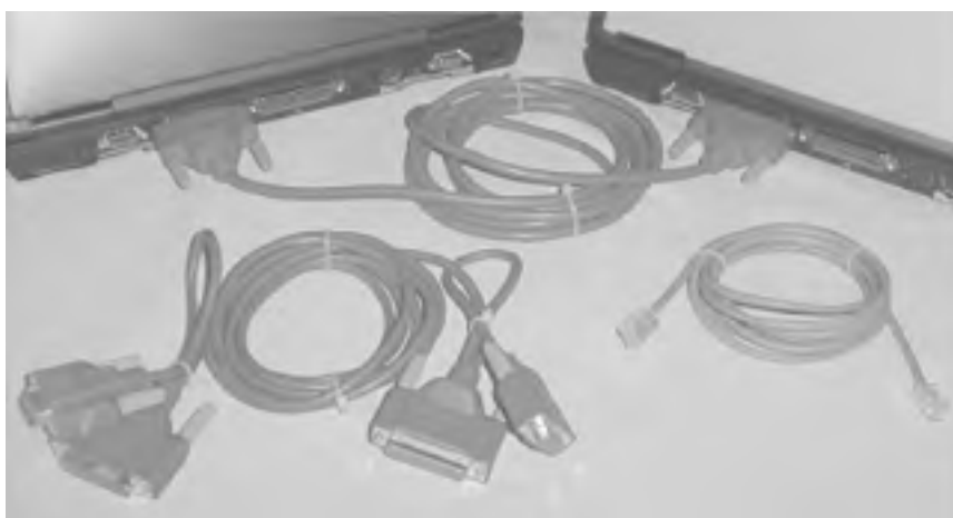
Figure 12-8. Null serial cable with DB-9 and DB-25 connectors (left), null Ethernet cable (right), and parallel data cable (back)
