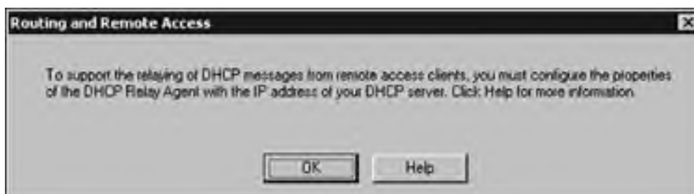
Figure 5.2. To complete the remote access process, you must configure a DHCP Relay Agent.
