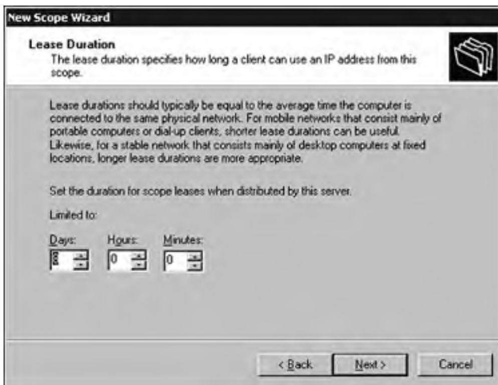
Figure 2.10. You can configure the lease duration for a scope in days, hours, and minutes.
