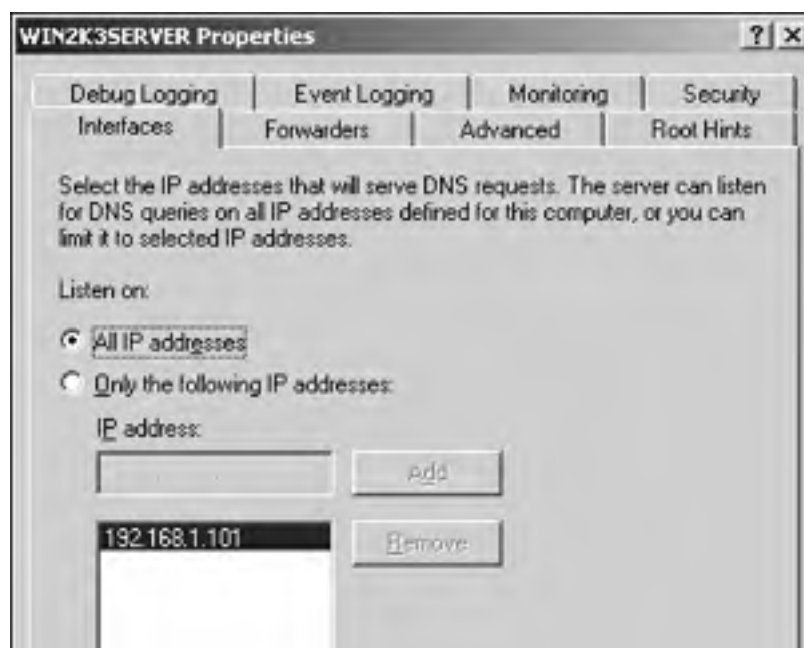
Figure 3.1. After installing the DNS service, you can configure DNS server options through the server's Properties dialog box.
