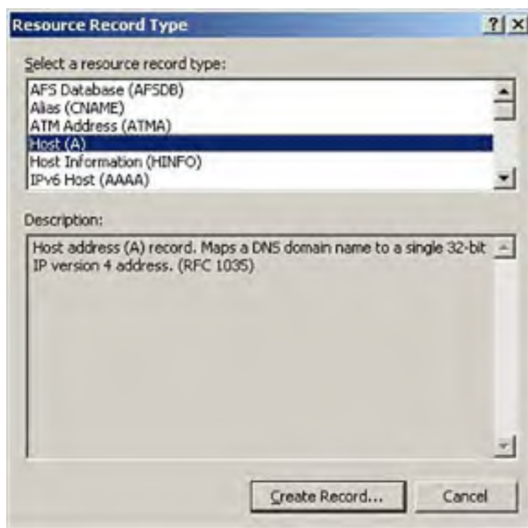
Figure 3.5. The next step in zone creation is populating the zone with DNS resource records.
