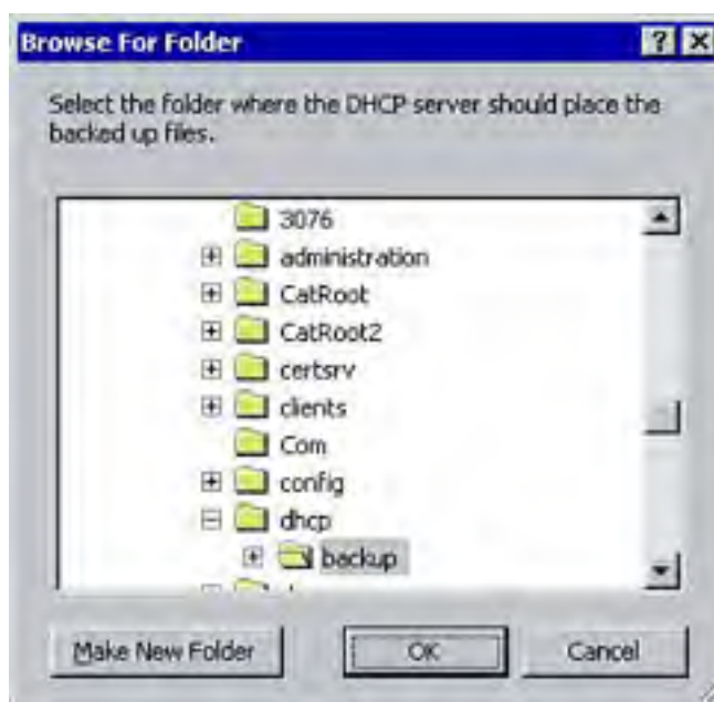
Figure 2.15. You can choose a location for the DHCP backup files via the management console.
