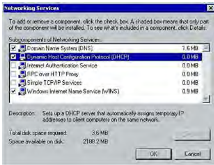
Figure 2.7. You can install DHCP through the Add or Remove Programs applet the Control Panel.
