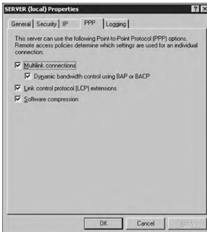
Figure 5.3. You configure PPP via the PPP tab in the Properties window of the remote access server.
