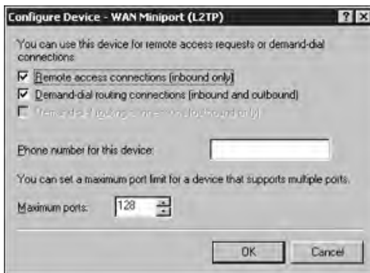
Figure 5.4. You configure ports via the Ports Properties icon on the RAS server.
