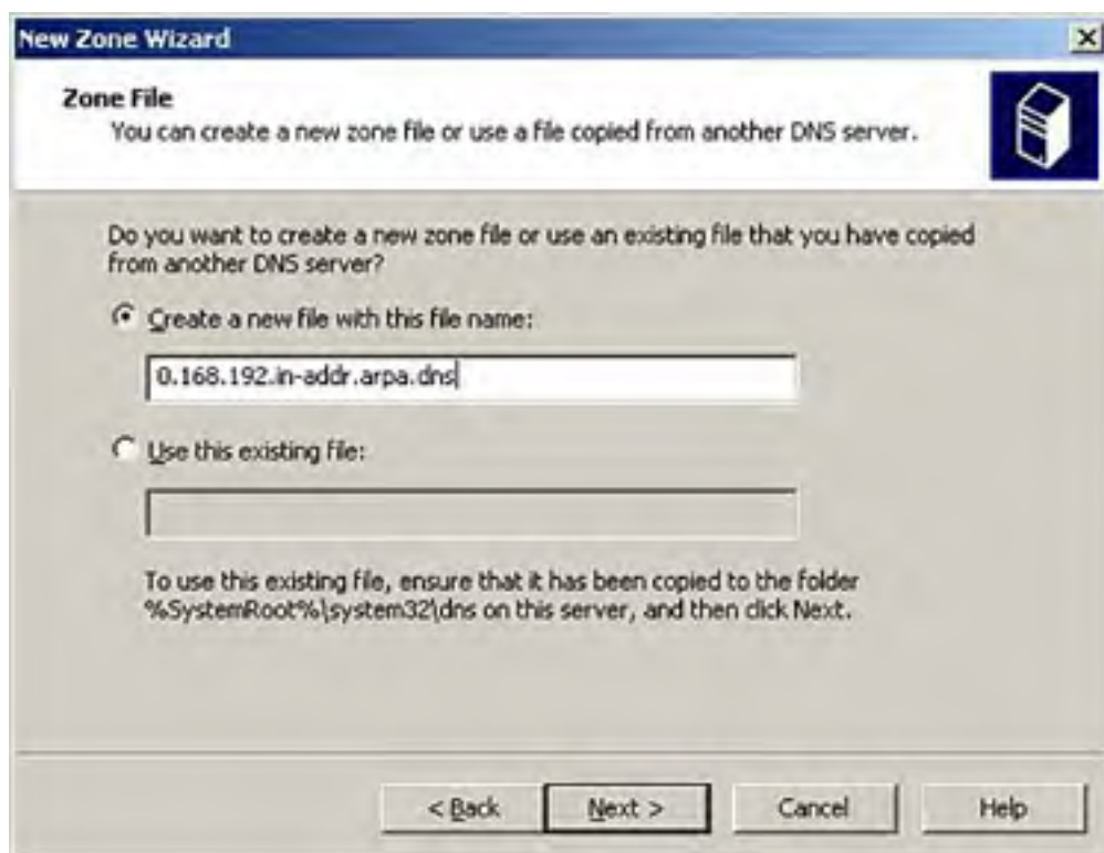
Figure 3.3. You must provide a filename for the zone file or select an existing file.
