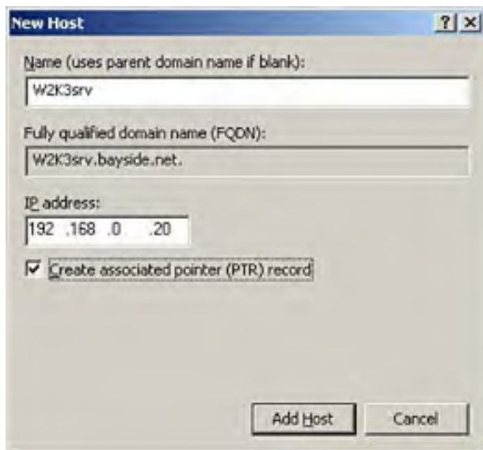
Figure 3.6. You can add a new host record via the DNS management console.
