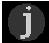
Figure 14-3: Transparent graphic with aliased edges (no halo effect)
