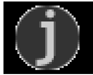
Figure 14-2: A “halo” effect created by anti-aliased edges in a transparent graphic
