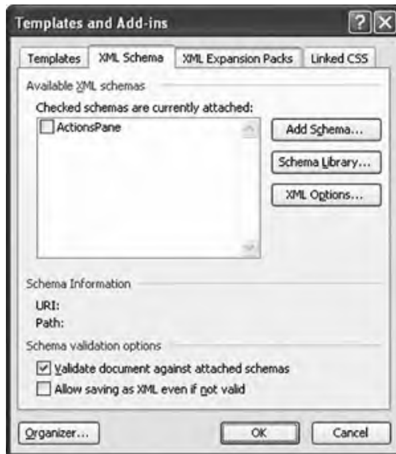
Figure 22.3. The Templates and Add-Ins dialog box with the XML Schema tab selected.
