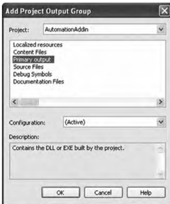
Figure 3.15. Adding the Primary output of the Automation Addin project to the setup project.
