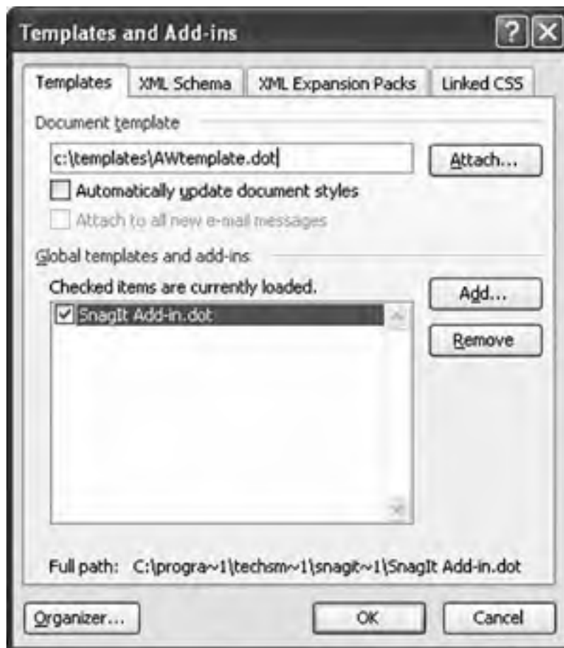
Figure 8.3. The Templates and Add-ins dialog box, showing the attached template and global templates.
