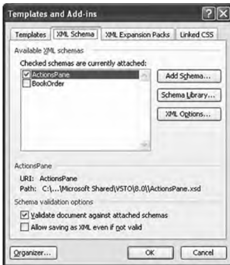
Figure 15.11. The ActionsPane solution attached to a Word document is visible in Word's Templates and Add-Ins dialog box and can be removed if ActionsPane.AutoRecover is not set to TRue.
