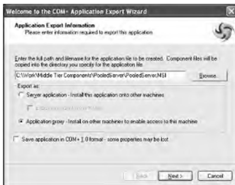
FIGURE 16.13 Generating an MSI package for installing the component's proxy on the client computers
