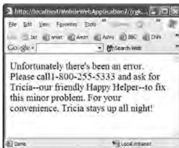
FIGURE 22.10 Rather than the default messages, intercept errors and show users something they can understand.
