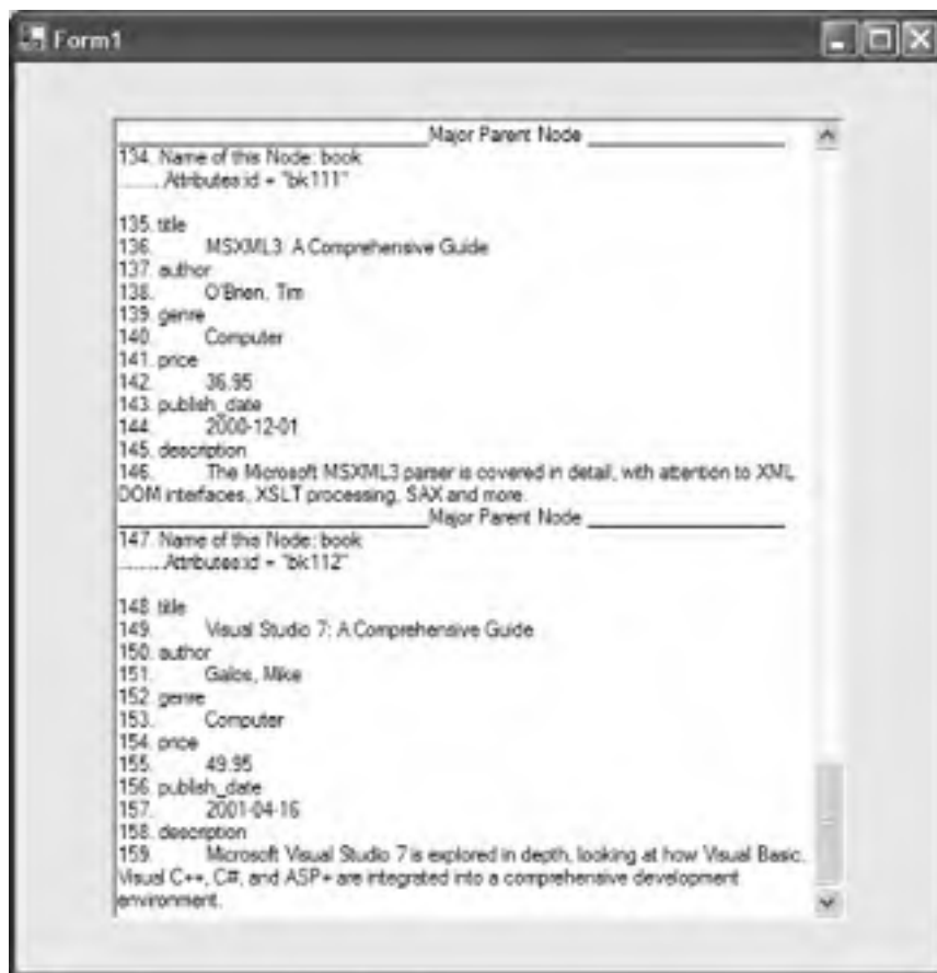
FIGURE 17.1 The program atomizes an XML document into its smallest components.
