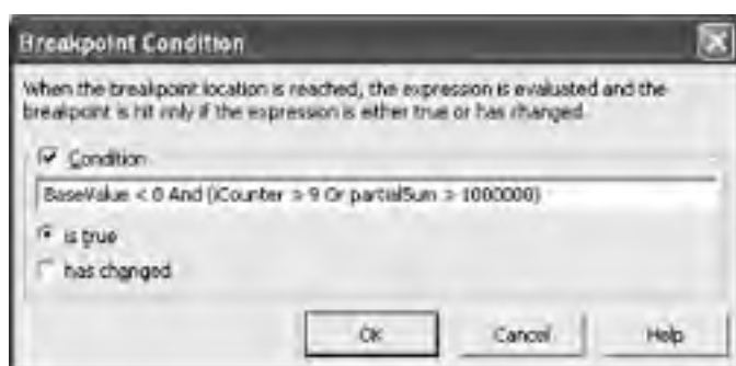
FIGURE 9.6 Setting the properties of a breakpoint
