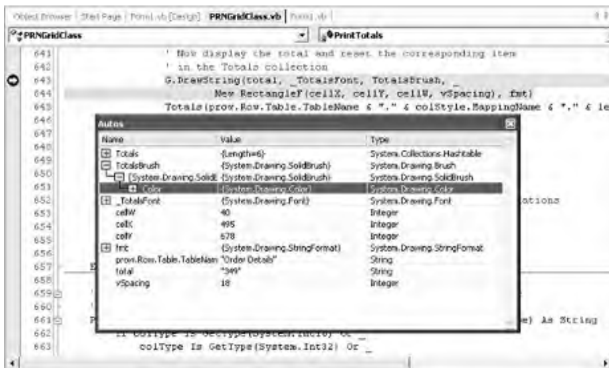
FIGURE 9.7 The Autos window displays the values of the variables used in the current statement.
