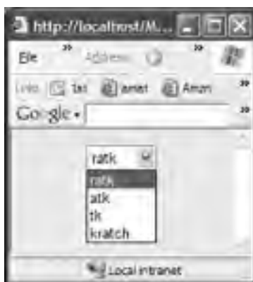
FIGURE 22.3 Simulate a mobile device during testing by resizing your browser until it's very, very small, like this.
