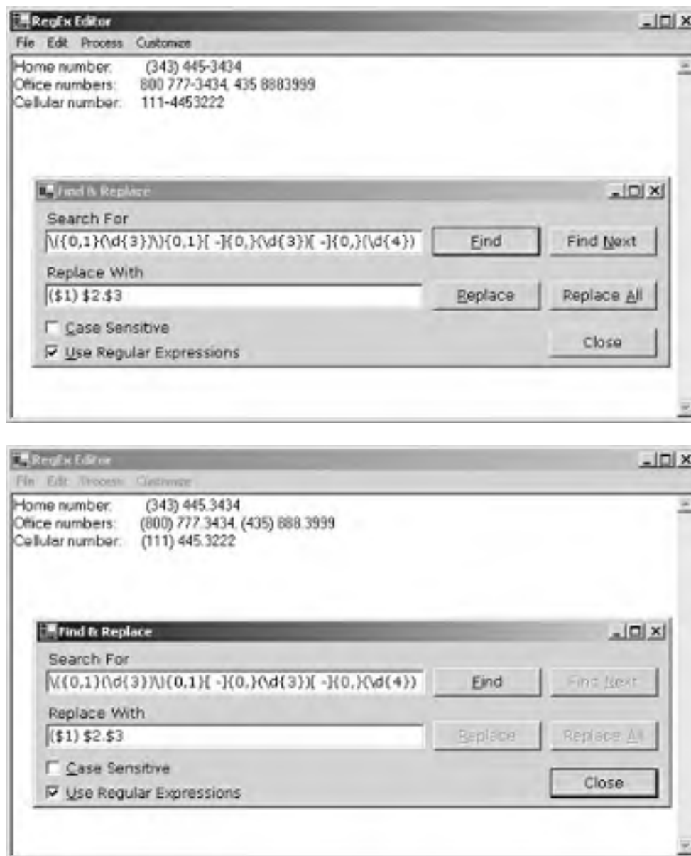
FIGURE 19.6 Using regular expressions in replacement operations. The original text (top) and the same text after the replacements (bottom).
