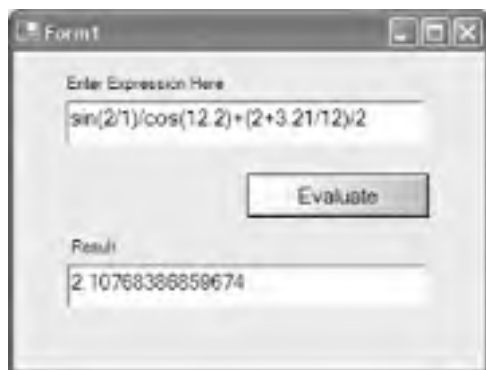
FIGURE 4.1 Borrow Excel's expression evaluation abilities to permit users to enter math expressions into your VB.NET applications.
